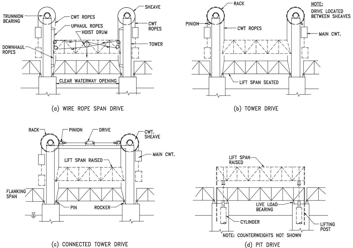
Figure 3.3.1-1: Types of Vertical Lift Bridges.
