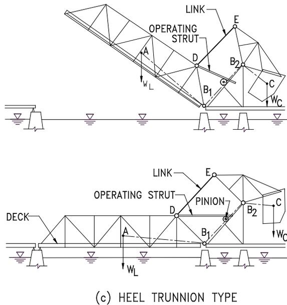
Figure 3.2.4-1: Types of Strauss Bascule Bridges.
