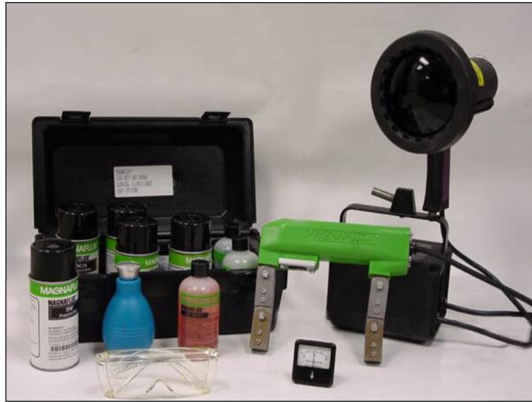
Figure 5.7.1-3: Magnetic Particle Inspection Kit.
