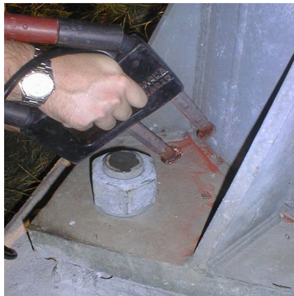
Figure 5.7.2-2: Prod MT on a Sign Structure Base.
