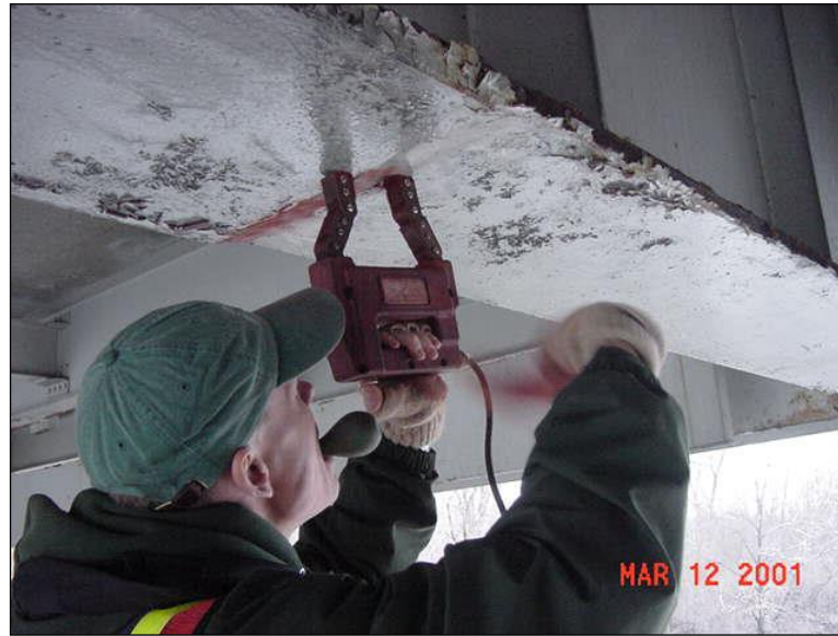
Figure 5.7.2-1: Yoke MT on a Built-Up Plate Bridge Girder Butt-Weld.
