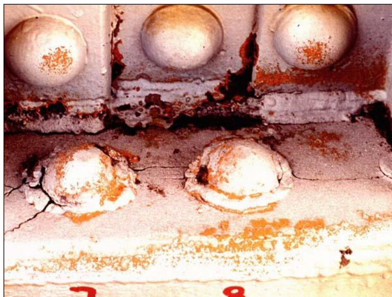
Figure 2.1.4.4-4: Fatigue Cracks on a Steel Casting.
