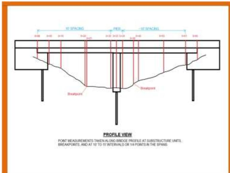
This drawing shows example locations of point measurements along the bridge profile: at substructure units, at breakpoints, at spacing of 10' along the bridge.
