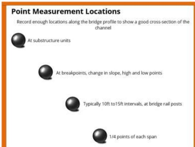
There must be enough point locations along the bridge profile to show a good cross-section of the channel. The point measurements along the bridge profile must capture the high and low points at reasonable intervals. The point measurements must be taken at the substructure units, at breakpoints (changes in slope/high & low points) between the substructure units, and at spacing typically of 10' to 15' intervals or  $\frac{1}{4}$  points of each span or at the bridge rail posts.
