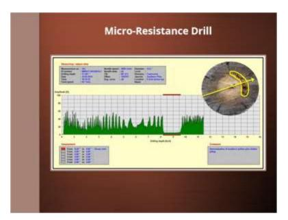
Here is a look at the computer software where readings from the Resistograph are saved. A cross section of the timber sample used for this measurement is provided as well. In this example, you can see how the graph picked up the area with a decay void that otherwise would not have been observed with visual inspection.
