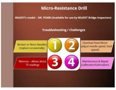
The Resistograph model owned by WisDOT, the IML PD400, has been used reliably for several years now. Here are a few tips to consider when using it.
