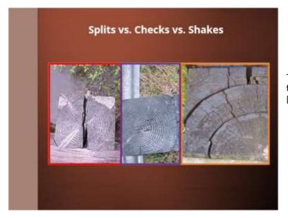
First, let's review some terminology for timber defects. This image shows the common defects associated with wood: knots, checks, shakes, and splits.
