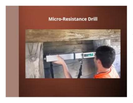
Here it is in action, showing the model WisDOT owns. It has a display screen in which the relative resistance can be observed while drilling.
