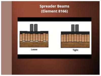
As timber expands and contracts and bolts become loose, spreader beams need to be regularly tightened and shimmed to maintain tight contact across the bottom of the slab.
