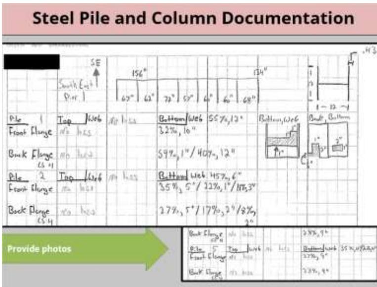
When section loss appears to be greater than 5 percent take measurements to determine the actual amount of section loss. When section loss is measured to be greater than 15 percent per element a sketch is required. This sketch should include percent section loss at each location on the element including the size and location of voids.
