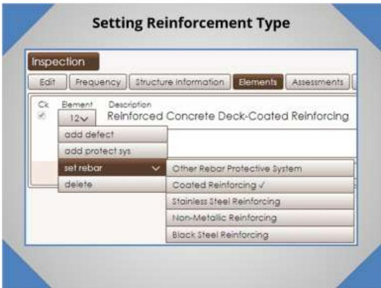
“The deck or slab rebar type can be selected by hovering over the element number, moving to ‘set rebar’, and selecting the appropriate type of reinforcement.
