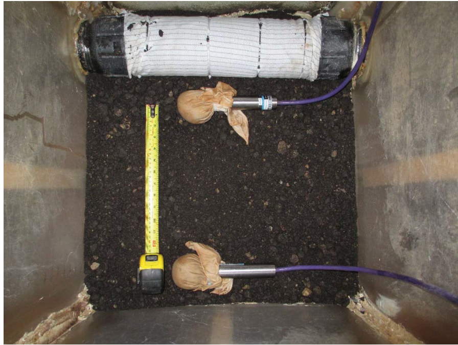
Figure 43. Geokon 3400 dynamic piezometers inside abutment model
