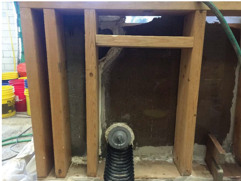
Figure 33. Drain tile plugged for saturation
