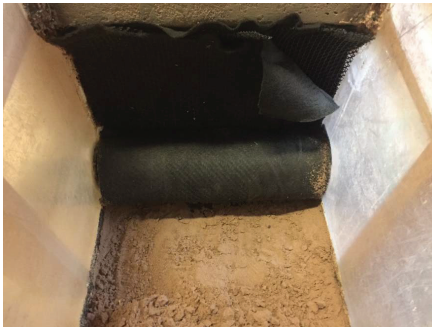
Figure 73. Geocomposite wrapped drain tile (top view)
