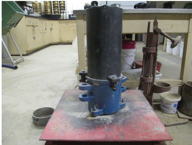
Figure 22. Vibrating table for relative density tests
