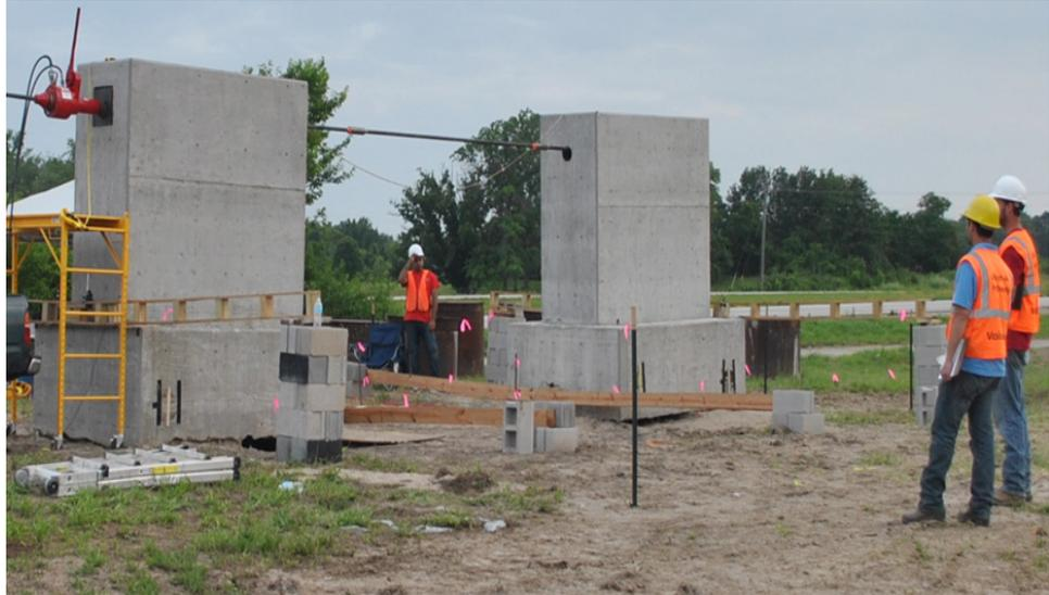
Pile structures during final load step. CIP pile cap is at left and H-pile cap is at right
