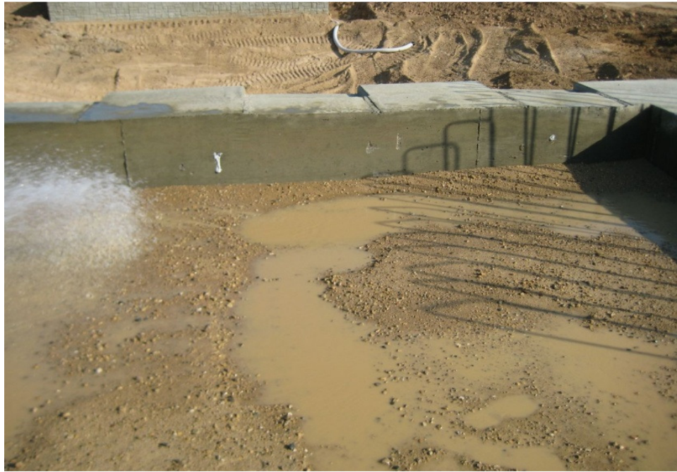
Figure 5.3. Ponding Observed on the Backfill Surface During Flooding. The picture here was taken 30 minutes after the water was turned on.
