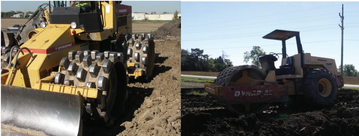
**Figure 4.28:** Field soil compactors used during field testing at the Town of Sylvania site.
