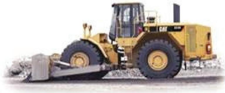
**Figure 2.10:** Caterpillar™ 824C rubber-tired roller (Operating equipment mass is 28,724 kg - 63,325 lb – Source: Caterpillar 2009).
