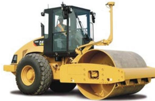
**Figure 2.8:** Caterpillar™ CS563 smooth-drum vibratory roller (Operating equipment mass is 11,120 kg - 24,520 lb. Operating drum mass at drum is 5,840 kg - 12,877 lb – Source: Caterpillar 2009).
