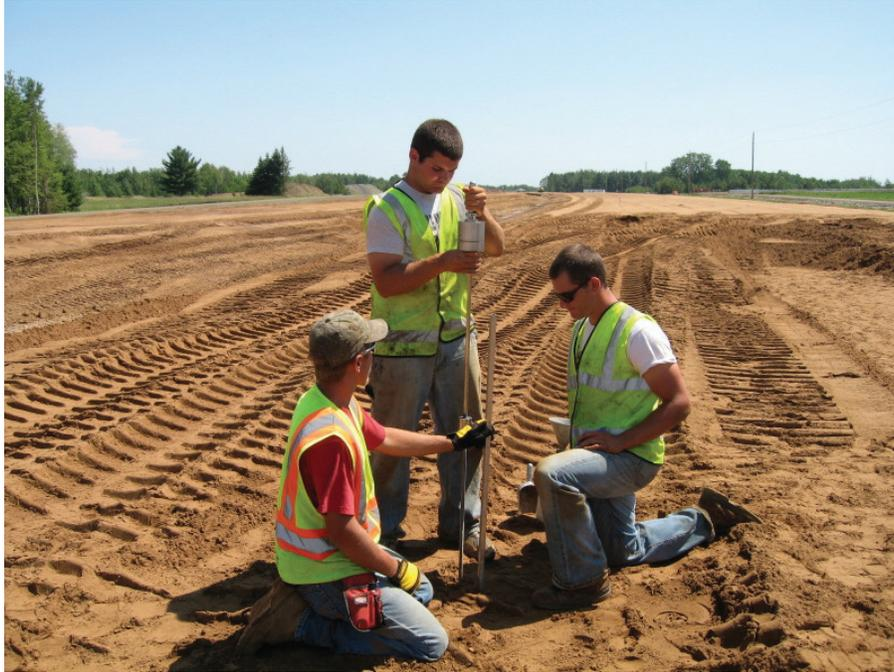
**Figure 4.3:** Testing using the dynamic cone penetrometer (DCP).
