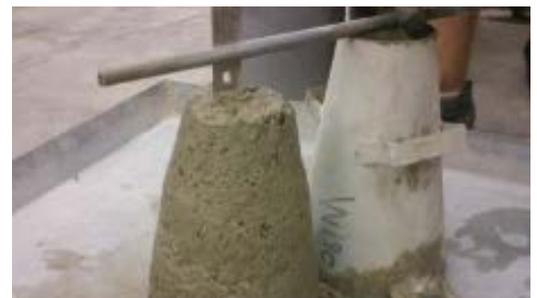
Testing the workability of concrete mixture using a slump cone
