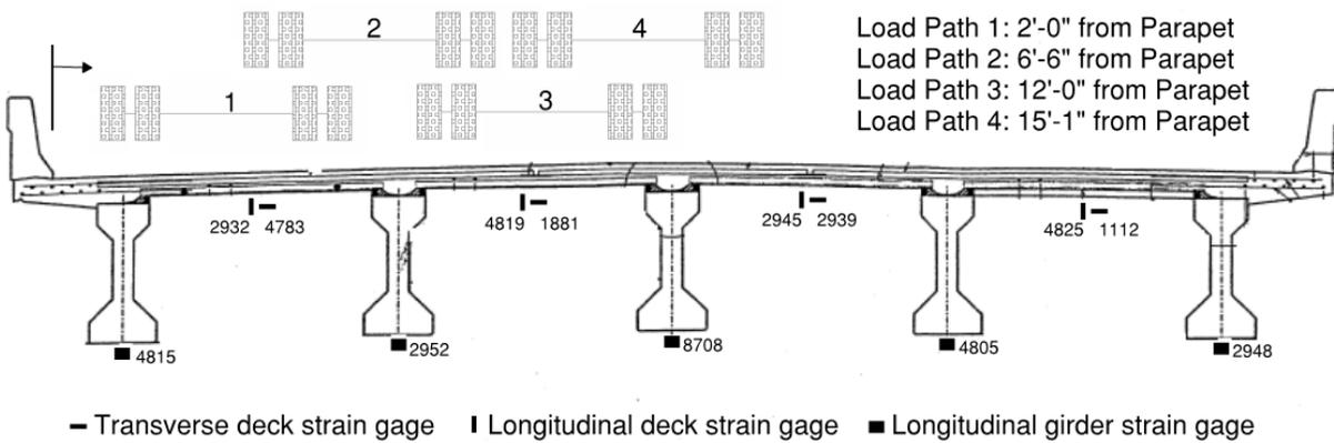
**Figure 62. US 151 northbound over STH 26 Service Road load path and gage locations - looking west**
