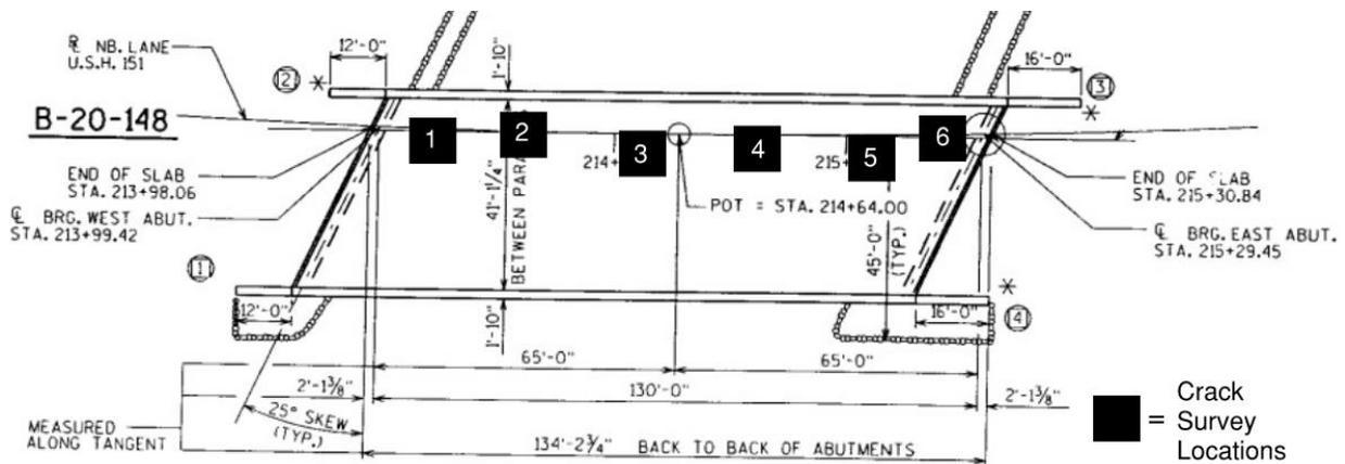
**Figure 95. US 151 over De Neveu Creek crack survey locations**
