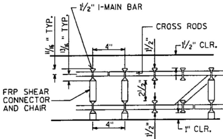
**Figure 85. US 151 over De Neveu Creek FRP deck reinforcement – 2**
