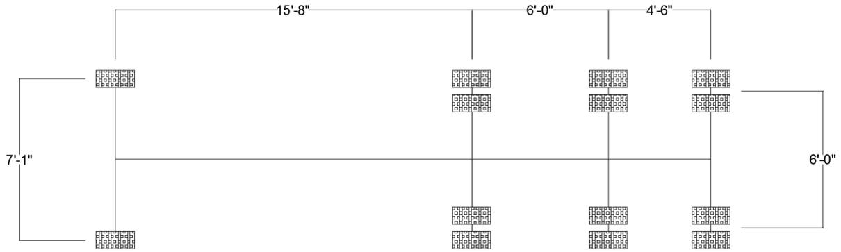
**Figure 61. US 151 northbound over STH 26 Service Road truck axle configuration**
