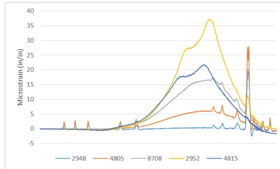
**Figure 68. Girder strain – Load Path 2**
