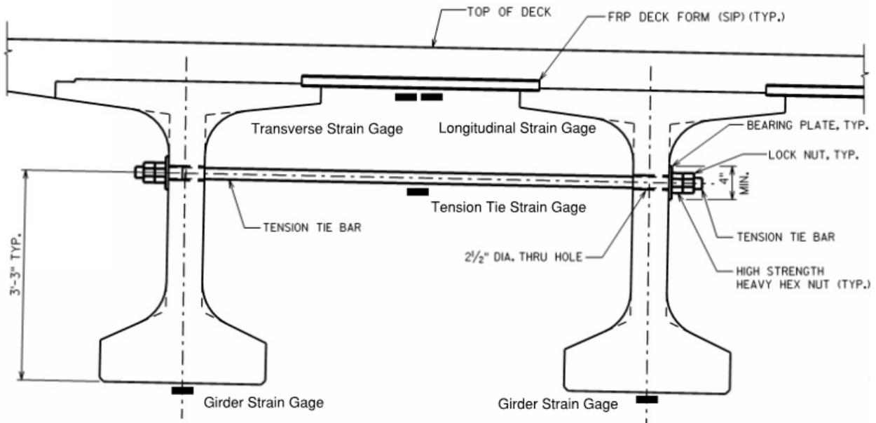
**Figure 107. US 12 over Coffee Creek typical gage configuration**
