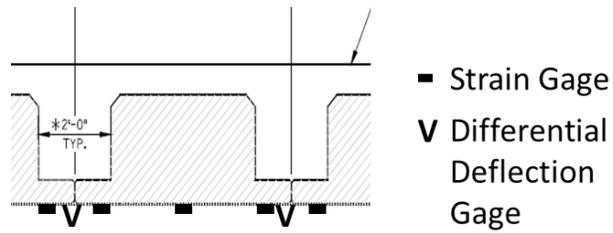
**Figure 29. US 41 over Ashwaubenon Creek instrumentation locations - typical cross-section**
