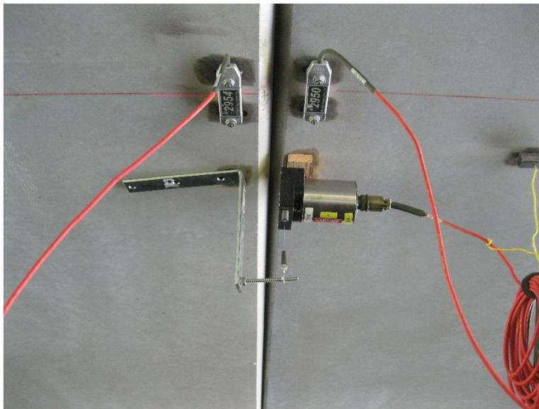
**Figure 10. STH 19 over Token Creek typical gage configuration**
