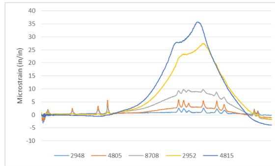
**Figure 63. Girder strain – Load Path 1**
