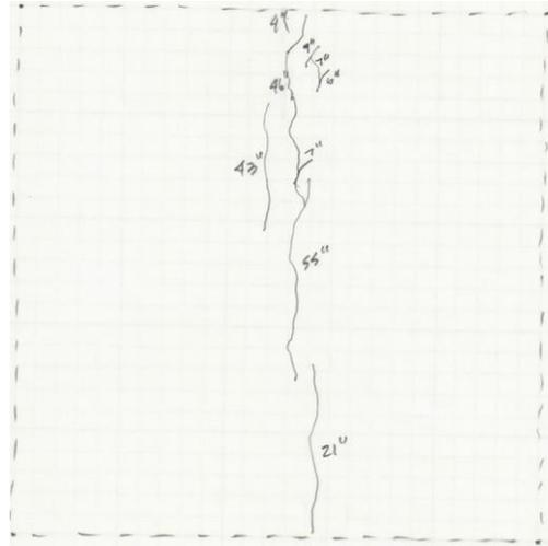
**Figure 99. US 151 over De Neveu Creek crack survey – Area 4**
