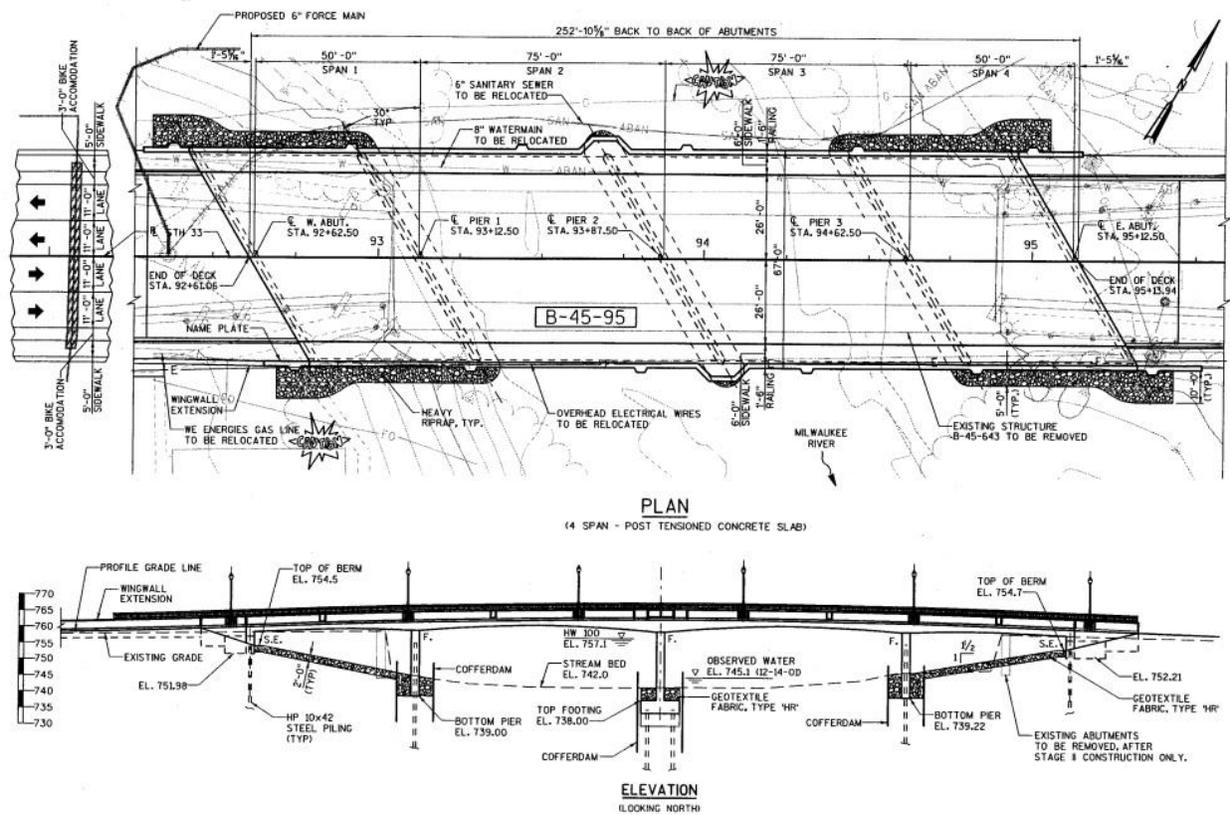
Figure 118. STH 33 over the Milwaukee River plan and section views
