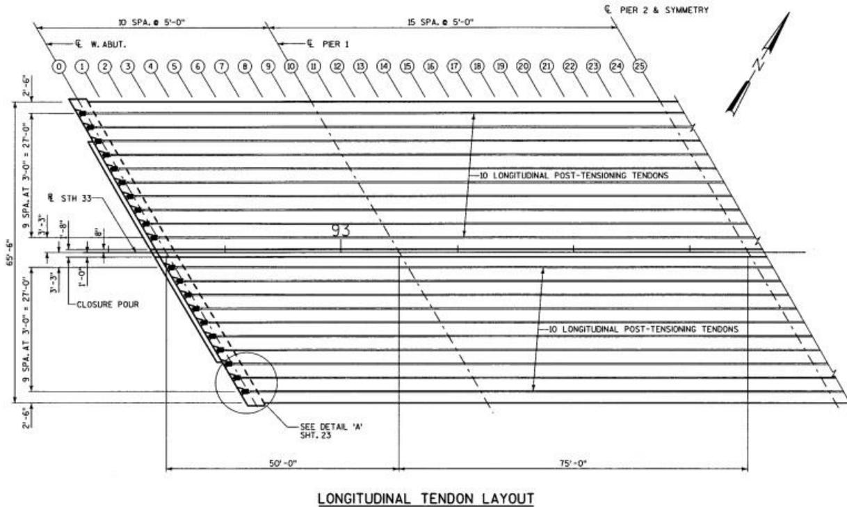
**Figure 119. STH 33 over the Milwaukee River longitudinal tendon configuration**
