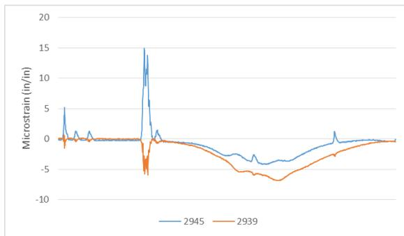
Figure 81. Bay 3 deck strain – Load Path 4
