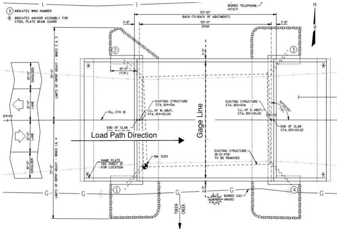
**Figure 13. STH 19 over Token Creek load path direction and gage locations**
