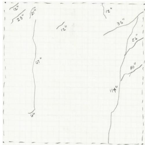
**Figure 101. US 151 over De Neveu Creek crack survey – Area 6**
