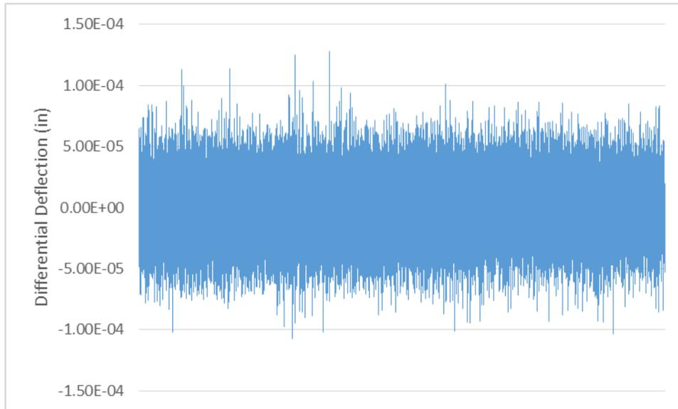
**Figure 34. US 41 over Ashwaubenon Creek differential deflection under load**
