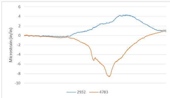
**Figure 74. Bay 1 deck strain – Load Path 3**
