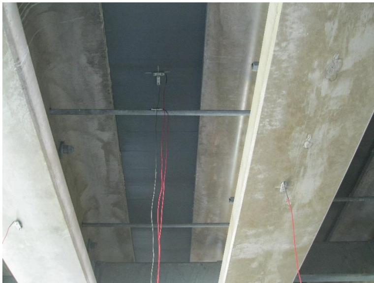
**Figure 109. US 12 over Coffee Creek typical gage configuration installed**
