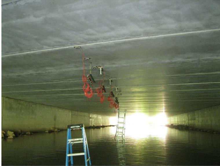
**Figure 30. US 41 over Ashwaubenon Creek panel instrumentation**
