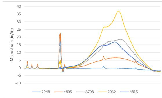
Figure 78. Girder strain – Load Path 4
