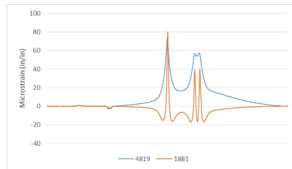
Figure 80. Bay 2 deck strain – Load Path 4
