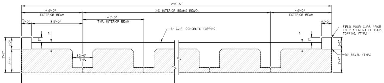
**Figure 25. US 41 over Ashwaubenon Creek inverted T superstructure**
