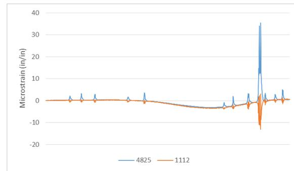
**Figure 72. Bay 4 deck strain – Load Path 2**
