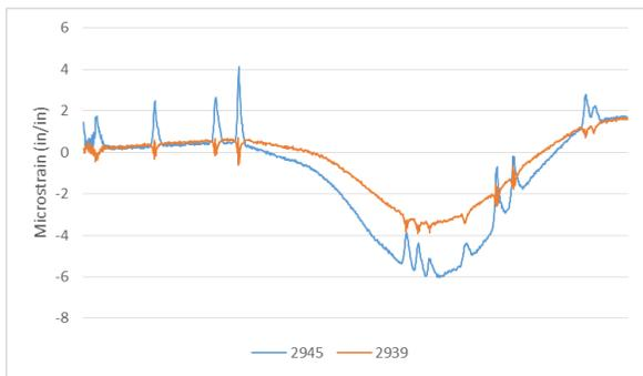
**Figure 66. Bay 3 deck strain – Load Path 1**
