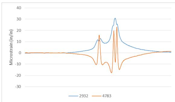
**Figure 64. Bay 1 deck strain – Load Path 1**
