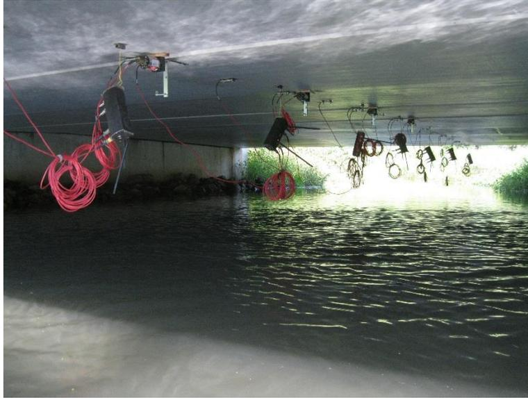
**Figure 9. STH 19 over Token Creek load test instrumentation**
