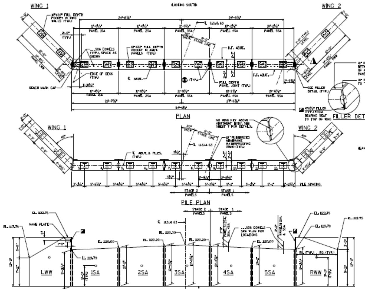
**Figure 136. US 63 over the Rush River precast abutment panel plans**
