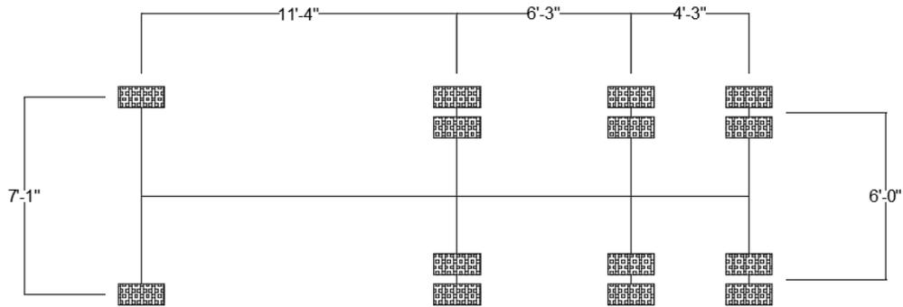
**Figure 110. US 12 over Coffee Creek tire and axle configuration**
