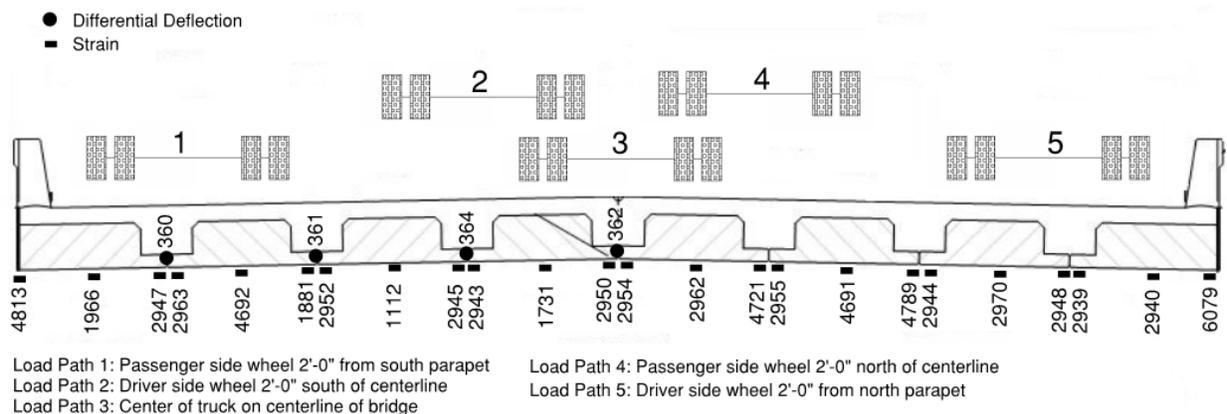
**Figure 14. STH 19 over Token Creek load path and gage positions – looking west**
