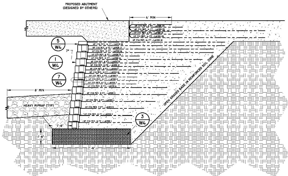
**Figure 48. SH 40 over Hay Creek GRS abutment section**
