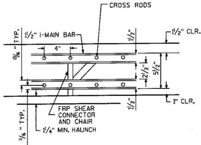
**Figure 84. US 151 over De Neveu Creek FRP deck reinforcement – 1**
