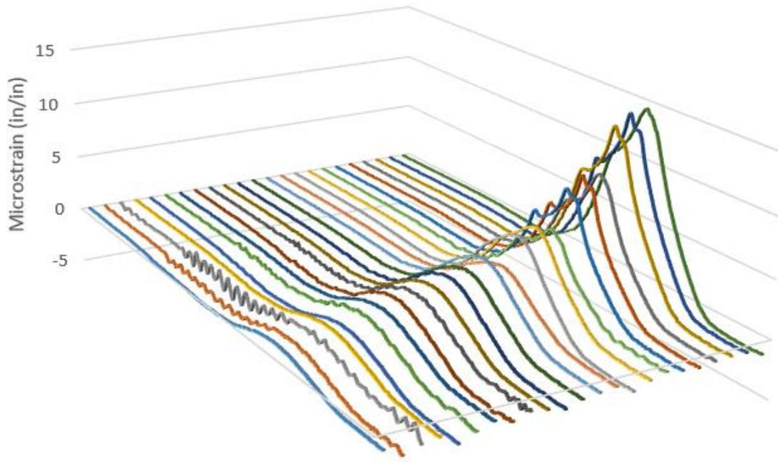
**Figure 24. STH 19 over Token Creek Load Path 5 – strain distribution**
