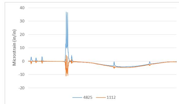
Figure 82. Bay 4 deck strain – Load Path 4
