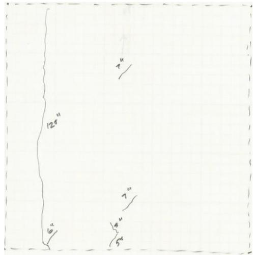
**Figure 100. US 151 over De Neveu Creek crack survey – Area 5**
