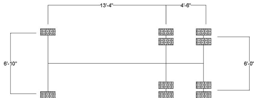
**Figure 12. STH 19 over Token Creek axle configuration**
