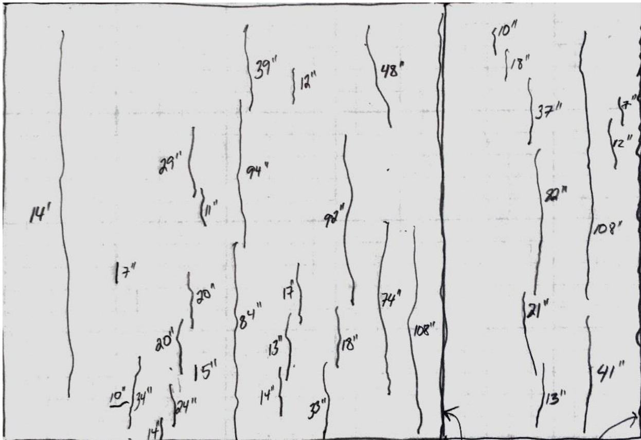
**Figure 52. SH 40 over Hay Creek crack map**
