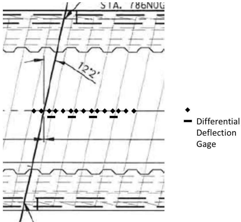
**Figure 28. US 41 over Ashwaubenon Creek instrumentation locations - plan view**
