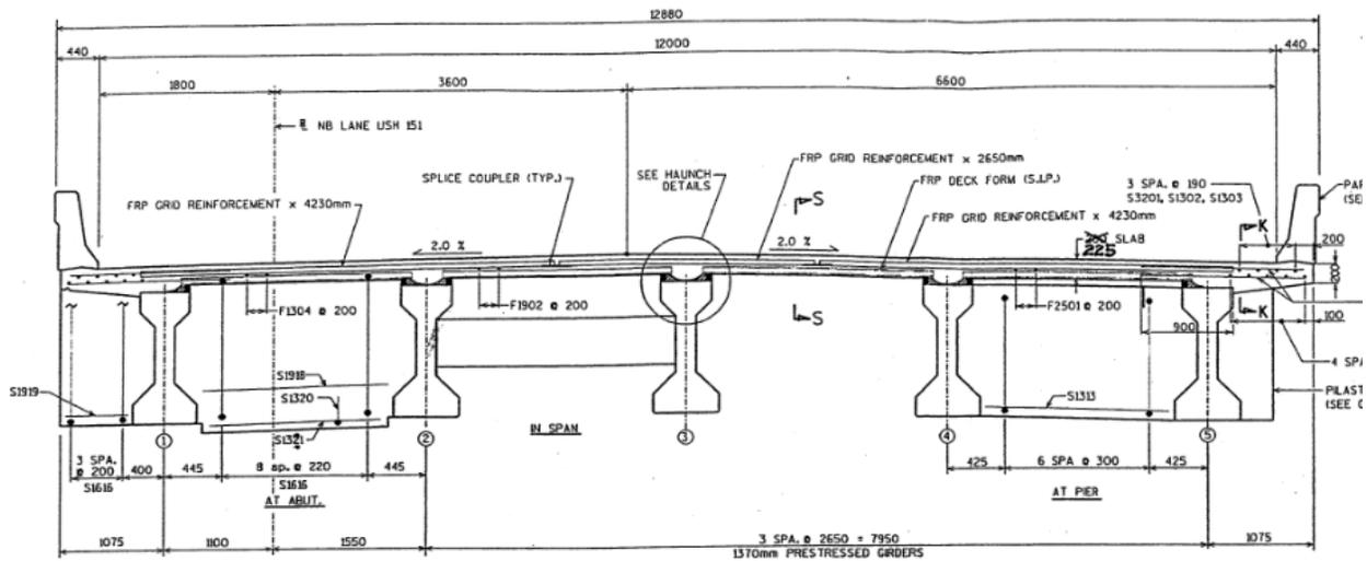
**Figure 54. US 151 northbound over STH 26 Service Road bridge superstructure plan**
