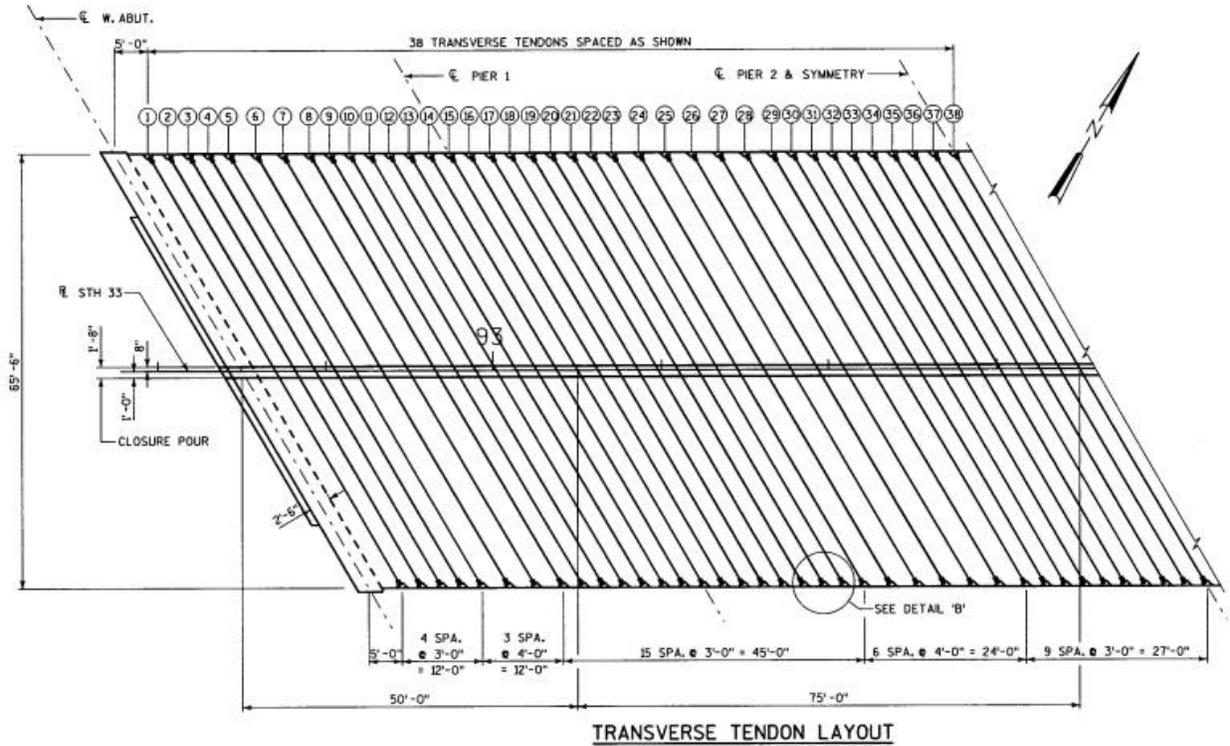
**Figure 120. STH 33 over the Milwaukee River transverse tendon configuration**
