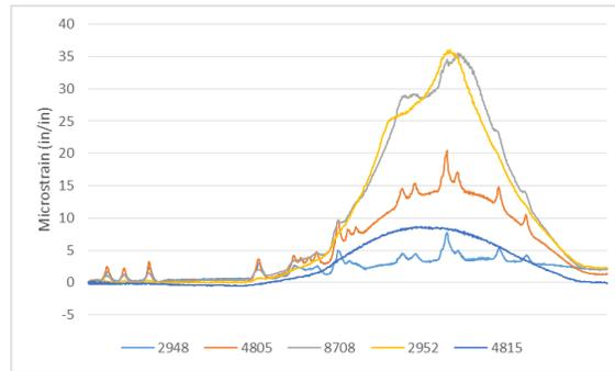
**Figure 73. Girder strain – Load Path 3**
