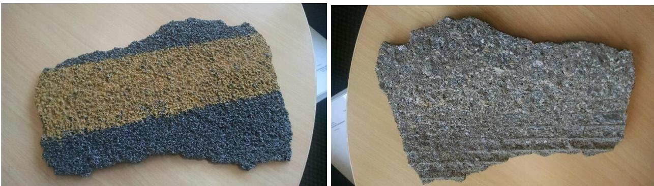
Figure 53. Delaminated multi-lift polyester overlay (from the Marquette Interchange ramp).
