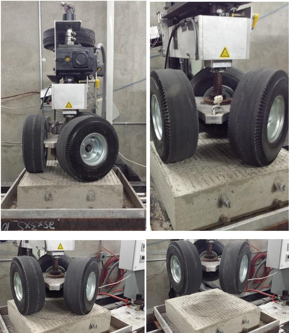
Figure 17. UWM-designed wear test device.
