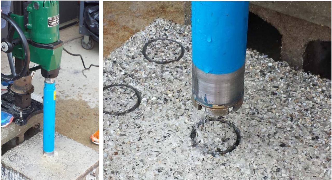
Figure 23. Coring drill setup.
