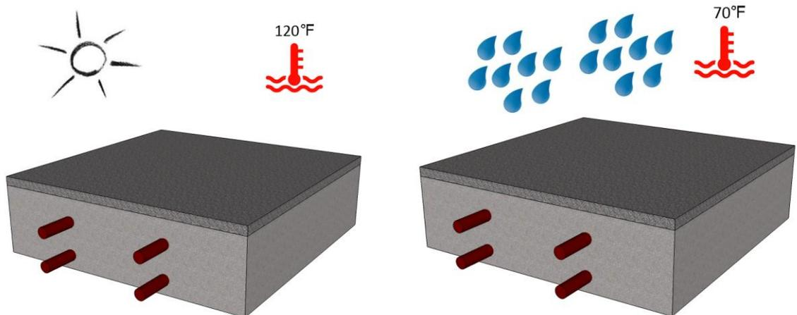
Figure 13. HURA test cycles: Heat and UV (left), rain and cool down (right).
