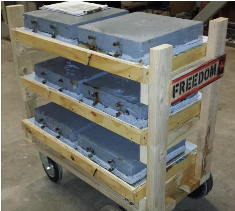
Figure 11. One of the three carts used for manual FT testing.
