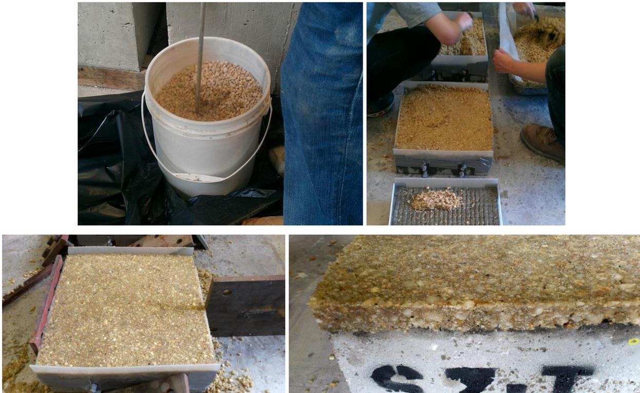
Figure 6. Pre-mixed polyester overlay system (S7) placement.
