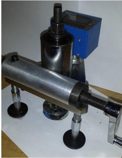
Figure 25. Pull-out test device.
