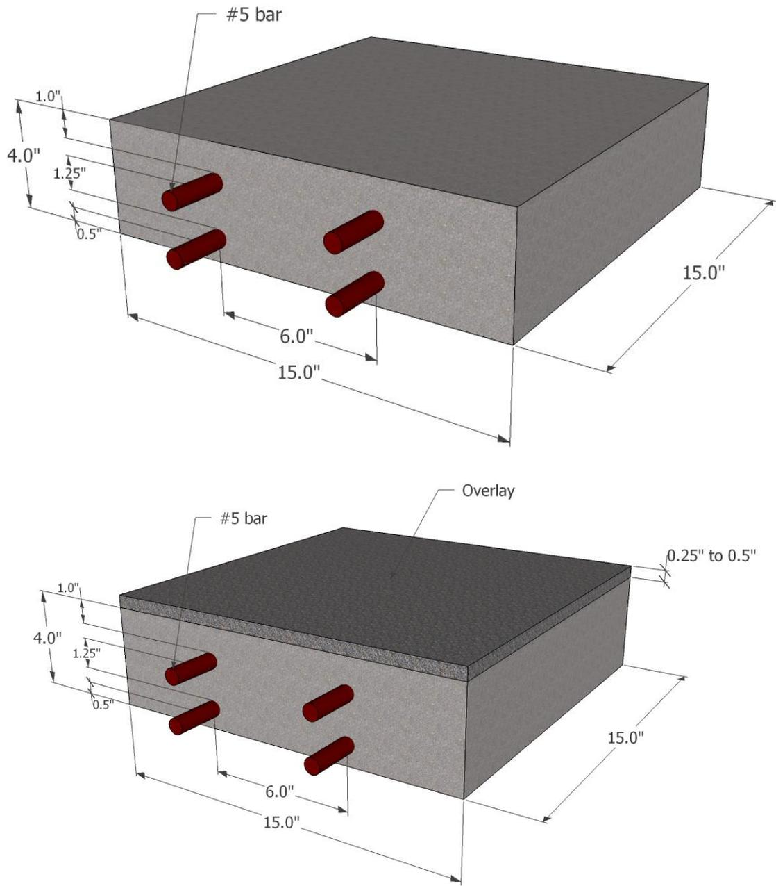
Figure 1. Concrete test specimen (with and without overlay).
