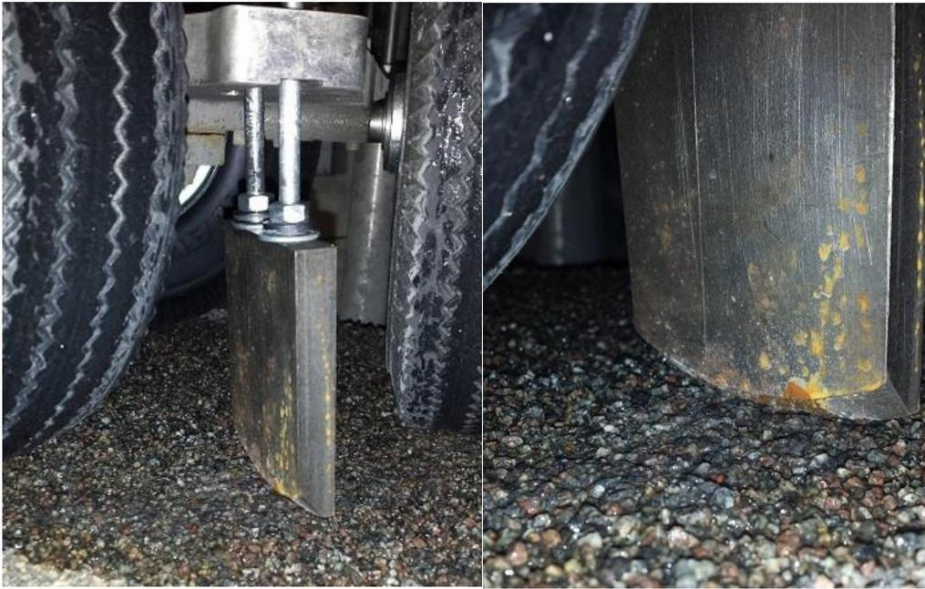
Figure 19. "Snow plow" assembly installed between two tires.
