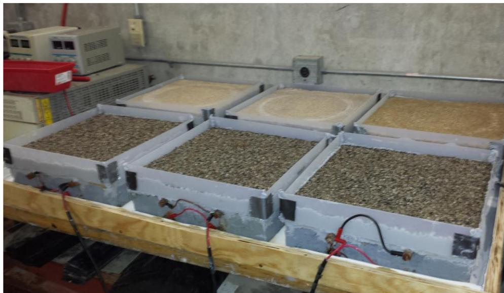
Figure 8. Accelerated corrosion setup.
