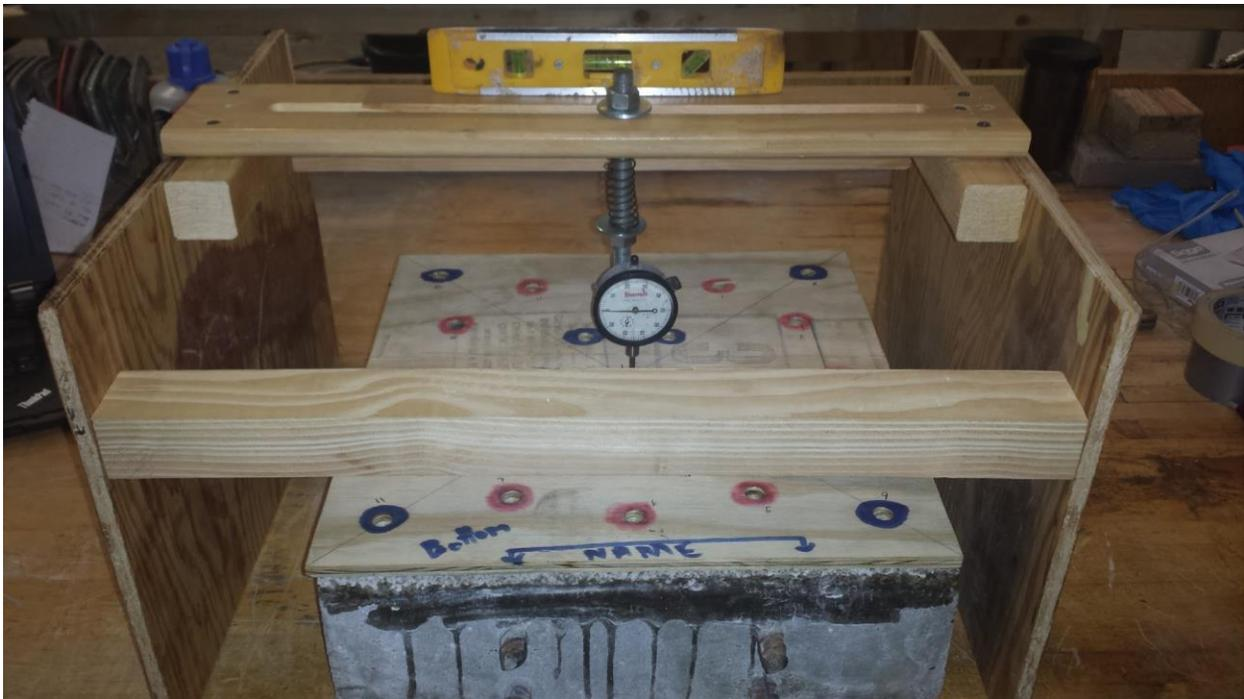
Figure 26. Measurement of the depth of surface groove (rut) through a dial gage at measurement points defined using a wooden template.
