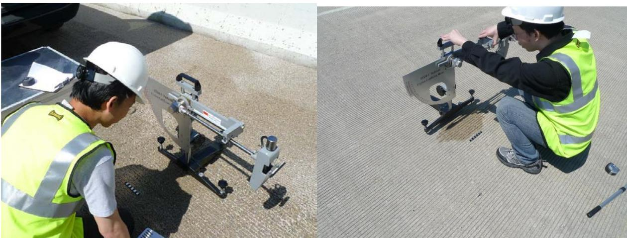
Figure 29. Friction testing using BPT.
