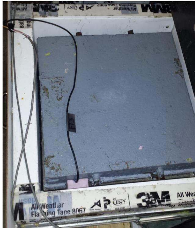
Figure 12. FT drawer with specimen placed face-down.
