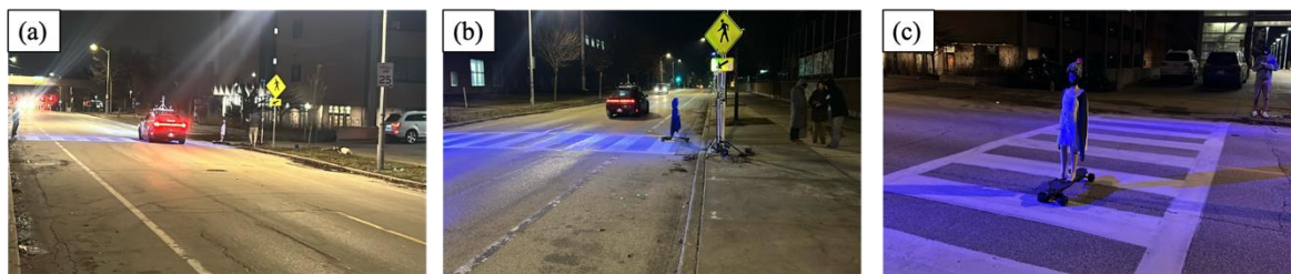
Figure 11. Test vehicle and roadway view during the Milwaukee demonstration. (a) Test vehicle approaching the illuminated crosswalk. (b) Vehicle approach with the pedestrian target near the crosswalk. (c) Roadway view showing enhanced lighting during vehicle approach.
