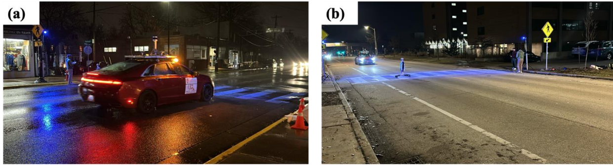
Figure 8. Nighttime field testing setup during enhanced crosswalk lighting experiments. (a) Madison field testing setup showing the instrumented test vehicle approaching the illuminated crosswalk under wet nighttime roadway conditions. (b) Milwaukee field testing setup showing the approaching test vehicle, mannequin mounted on an electric skateboard, enhanced crosswalk lighting, and field team coordination.
