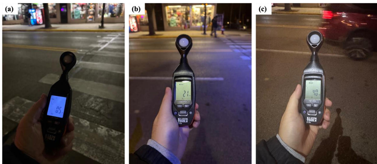
Figure 9. Madison nighttime illuminance measurements during field setup. (a) Baseline condition without enhanced crosswalk lighting, showing approximately 0.5 lux. (b) Enhanced crosswalk lighting condition, showing approximately 21 lux. (c) Enhanced lighting with additional floodlight support is used to simulate streetlight conditions, showing approximately 40 lux.
