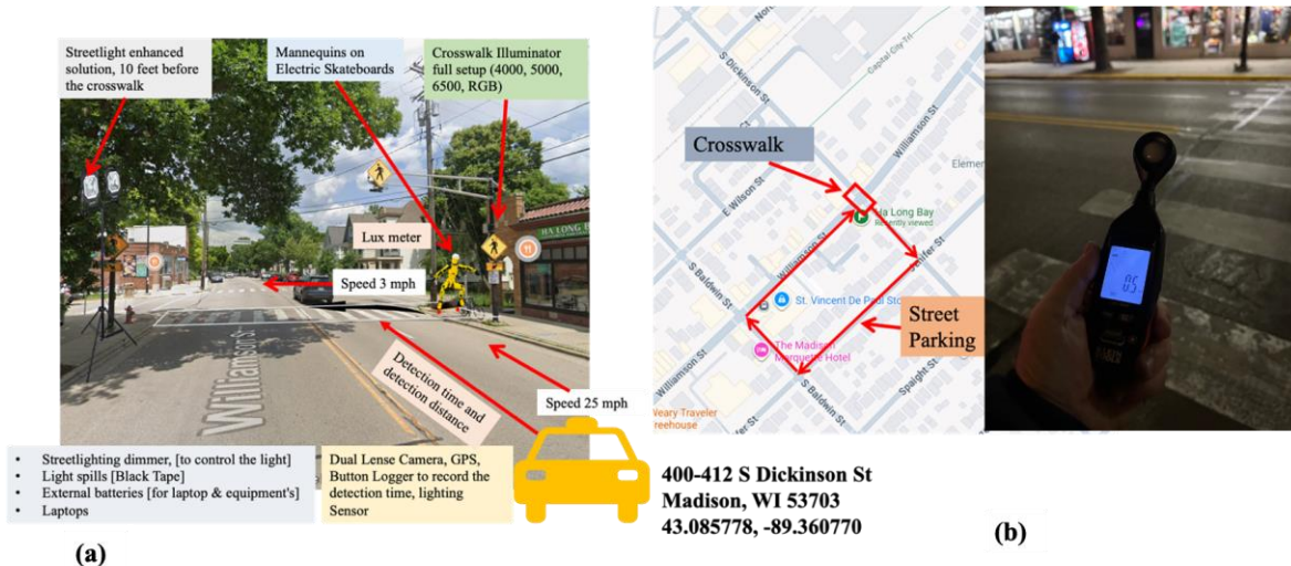
Figure 5. Madison field experiment layout, roadway map reference, and baseline nighttime illuminance measurement at Williamson Street and South Dickinson Street. (a) Field experiment layout and test site map showing the crosswalk location, mannequin crossing setup, lux meter location, vehicle approach path, and surrounding roadway context. (b) Baseline nighttime lux measurement collected before enhanced lighting, added flood light, or streetlight simulation was applied
