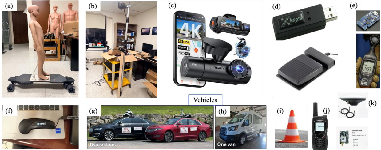
Figure 7. Field hardware and instrumentation used during nighttime crosswalk lighting experiments. (a) Mannequin mounted on an electric skateboard. (b) Temporary pole with crosswalk illuminator. (c) Camera system used to record the driver and roadway view. (d) Foot switch and reaction logging equipment used to record driver brake response. (e) Lux measurement meter used to document baseline and enhanced lighting levels. (f) Skateboard controller used to remotely control mannequin crossing movement. (g) Sedan test vehicles used for field data collection. (h) Van test vehicle used for obstruction and field testing scenarios. (i) Traffic control cone used for field setup and safety marking. (j) Satellite phone used for field communication and safety support. (k) GPS equipment used to record vehicle position, speed, heading, and timestamp.
