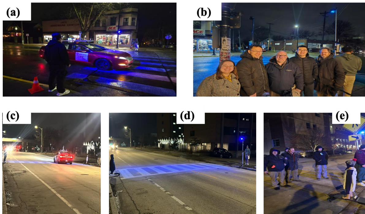
Figure 10. Enhanced crosswalk lighting demonstration at the Madison and Milwaukee field sites. (a) Madison demonstration showing the instrumented test vehicle approaching the illuminated crosswalk under nighttime field conditions. (b) Madison demonstration showing POC members and project participants during the field demonstration. (c) Milwaukee demonstration showing the instrumented test vehicle approaching the illuminated crosswalk under nighttime field conditions. (d) Milwaukee demonstration showing enhanced lighting coverage across the crosswalk. (e) Milwaukee demonstration showing POC members and project participants observing the enhanced lighting system and mannequin crossing setup.
