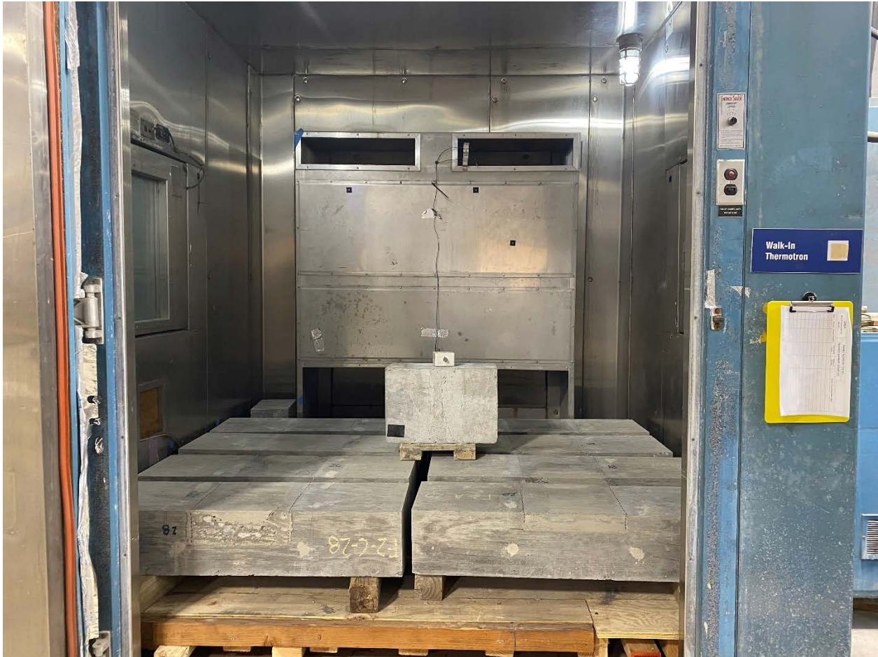
Figure 11. Thermal testing. Specimens in walk-in environmental chamber. Control concrete block (yellow arrow) had embedded thermocouples for controlling temperature cycles. Each cycle lasted approximately 1 day.
