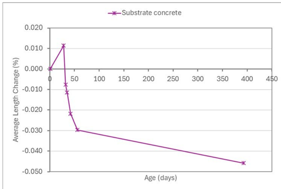
Figure 18. Drying shrinkage of repair materials and substrate concrete (substrate concrete specimens were cured in the mold for 1 day and wet-cured for 27 days before initiation of air storage)
