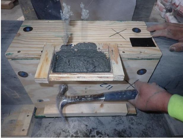
Figure C1.21. Form-and-pour in vertical orientation (patch on the vertical side)
