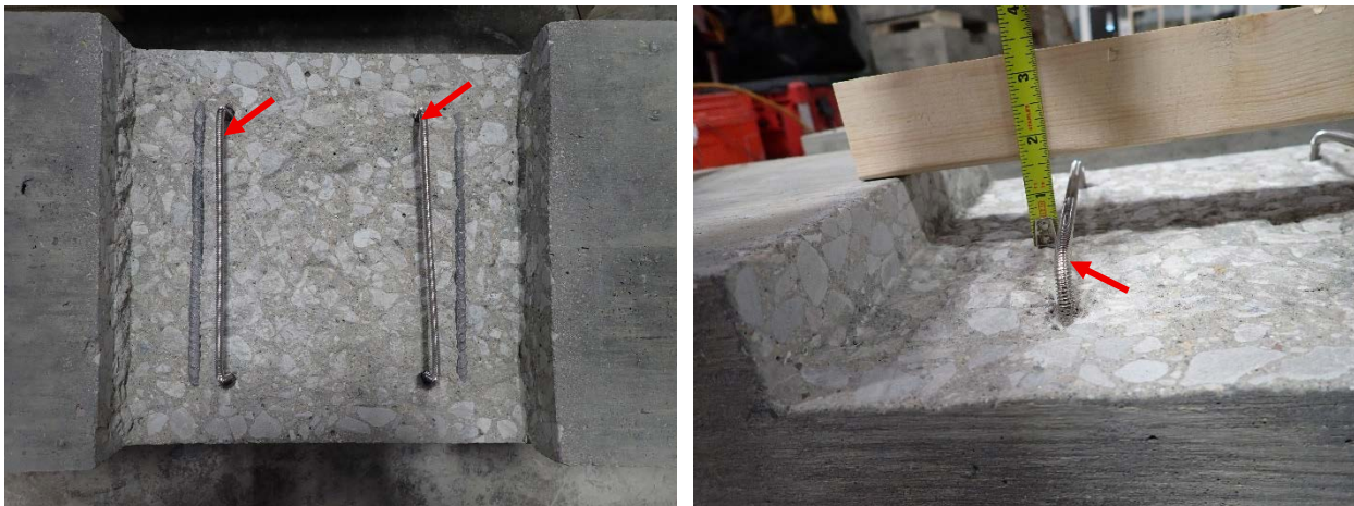
Figure 4. Anchorage by threaded rods U (red arrows) in 1-1/2-inch and 2-inch cavities
