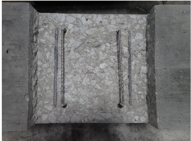
Figure C1.8. Threaded rod U (epoxy embedded)
