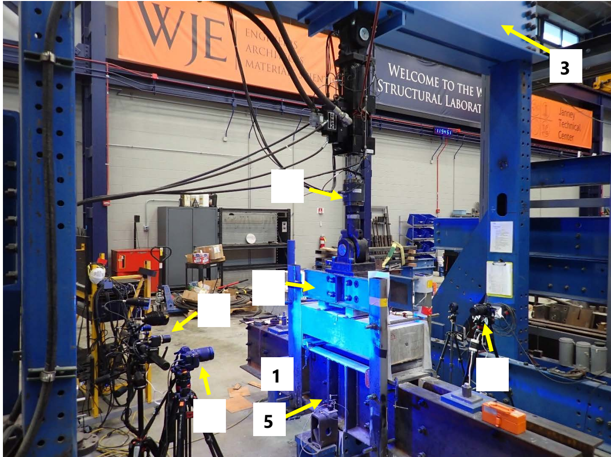
Figure 14. Overview of test setup: 1) Beam specimen; 2) 55-kip actuator; 3) Cross-head for reaction frame; 4) Spreader beam; 5) String potentiometer; 6) Camera system for 3D-DIC; 7) High-resolution digital cameras
