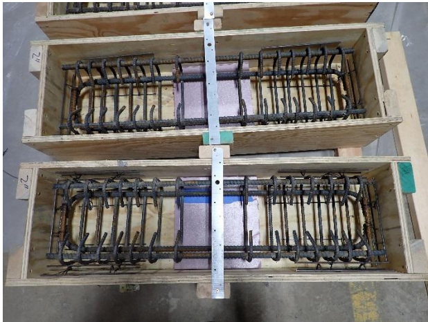
Figure C1.1. Forms and reinforcing
