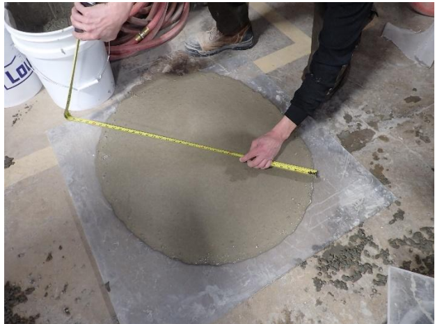
Figure C1.20. Slump flow test of form-and-pour material
