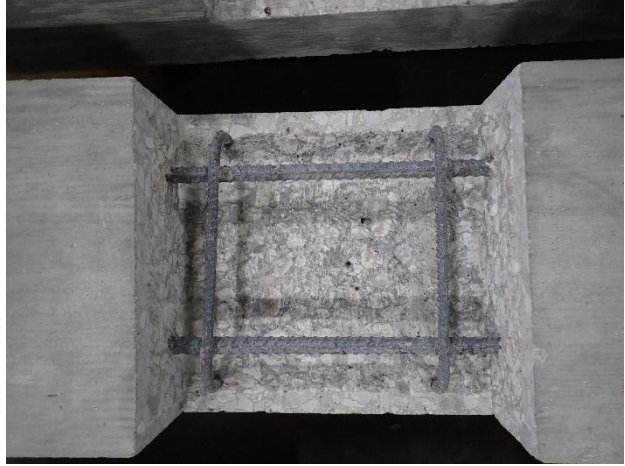
Figure C1.10. Patch encompassing existing reinforcement
