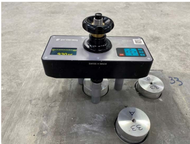
Figure 1. Tensile pull-off testing
