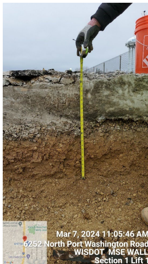
Figure 20. Concrete slab and underlying layers at the Section 1's excavation trench.
