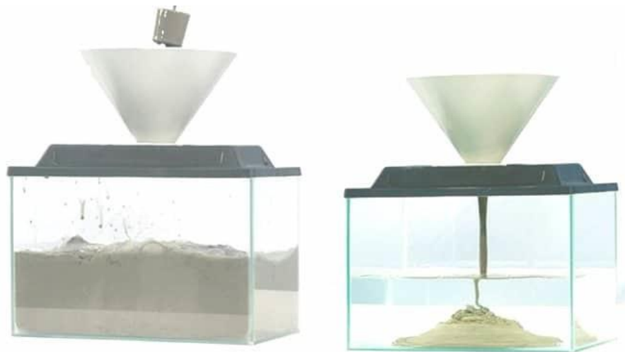
Figure 8. Effects of AWAs on underwater concrete placement: Material washout in the absence of AWAs (left) and enhanced cohesion after the addition of AWAs (right) [132]
