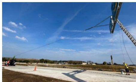
Static tests for torsional upstream and torsional downstream forces
