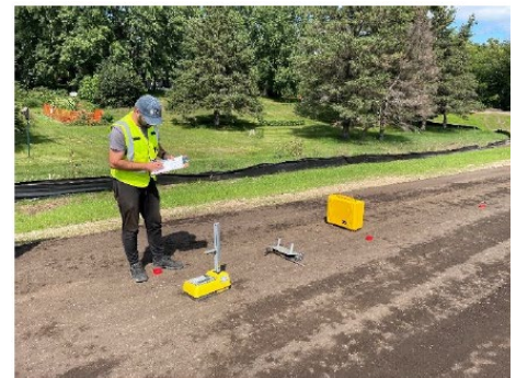
In-place density and moisture content test by nuclear density gauge (NDG) at in Dane County (left) and St. Croix County (right)
