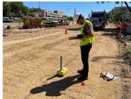
In-place density and moisture content test by nuclear density gauge (NDG) at in Dane County (left) and St. Croix County (right)
