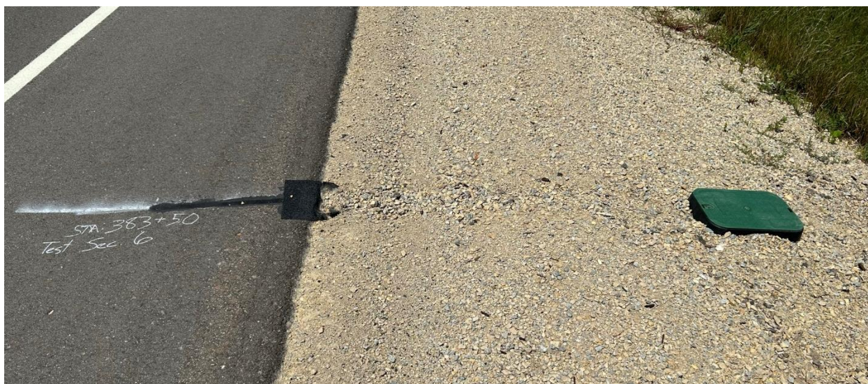
Figure 9. Photo of Installed Temperature Probe Array and Box Containing Datalogger
