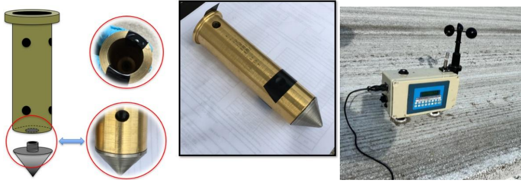
Figure 19. Approach in Measuring Curing Effectiveness Using Chilled Mirror Technology
