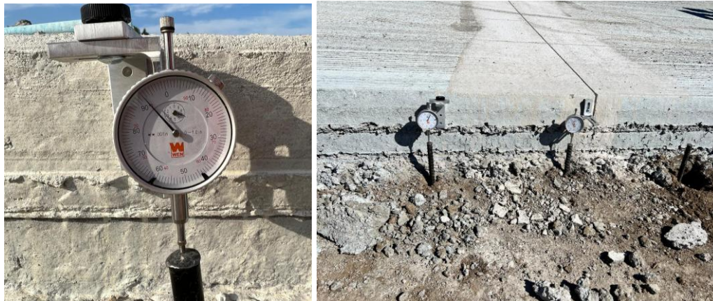
Figure 24. STH 15 Dial Gauge Placement (left), Off Set Dial Gauge Setup (right)
