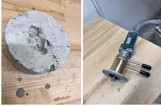
Figure 3. Concrete after grinding to collect the powder used for degree of hydration (A), The mechanical grinder used (B)
