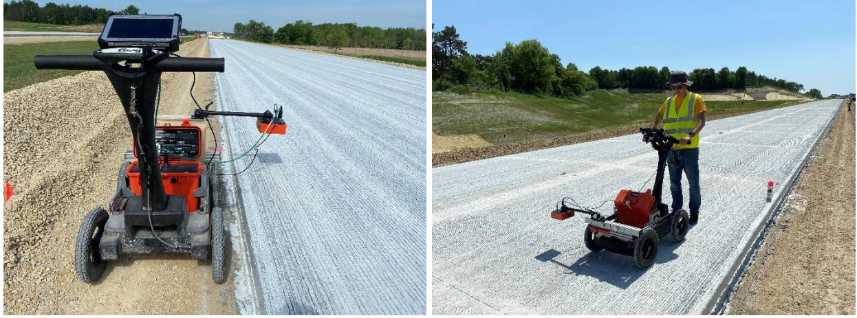
Figure 21. Modified GSSI Pavescan 1.0 GPR Used in Field Testing (left) on the side of new concrete, (right) on top of hardened concrete
