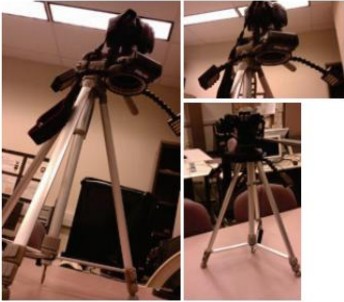
Figure A.7: Camera set-up for digital image correlation (Chen et al. 2011)
