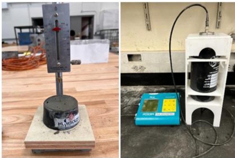
Figure 2. Vicat apparatus (left) and UPV (right) used for setting time
