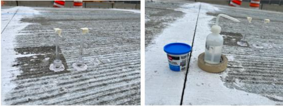
Figure 25. Karsten tube set-up during I-43 construction
