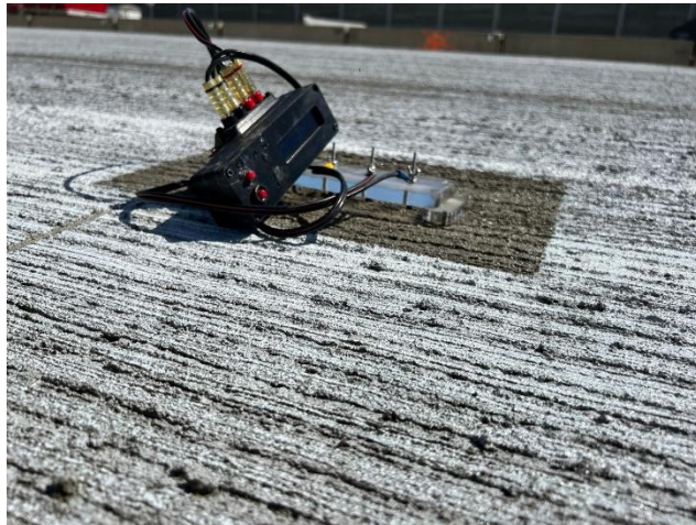
Figure 28. Embedded resistance device set-up during I-43 construction
