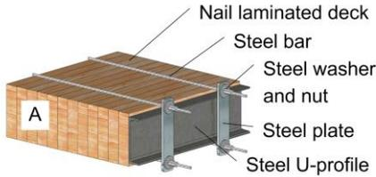
a) Measure of repair of nail-laminated decks;
