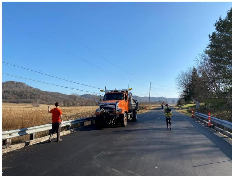
**Figure 4-13 Load truck crossing the bridge**
