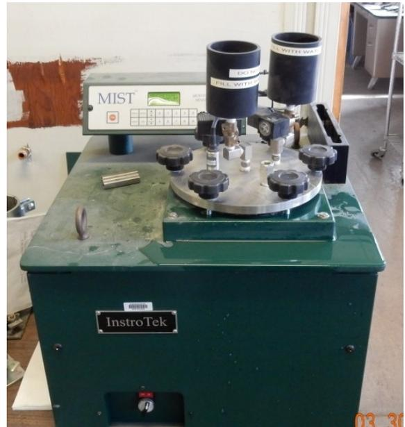
***Figure 3 Picture of MiST with lid secured ready for conditioning specimens***
