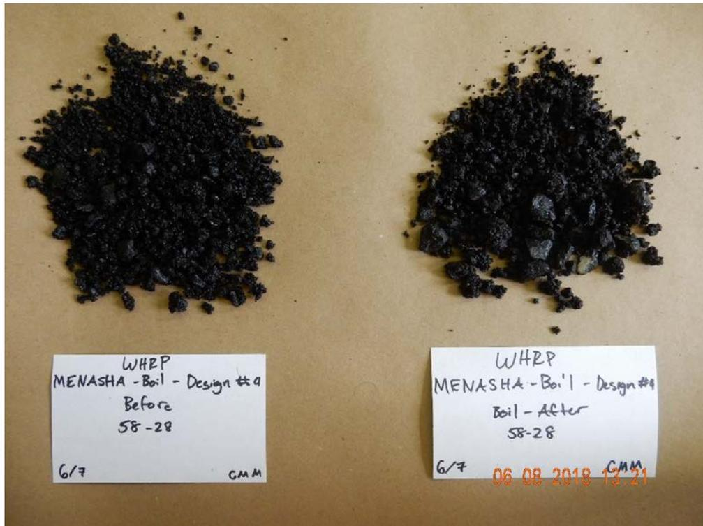
**Figure B-9 Before and after boil testing: Menasha aggregate with 58-28 binder**
