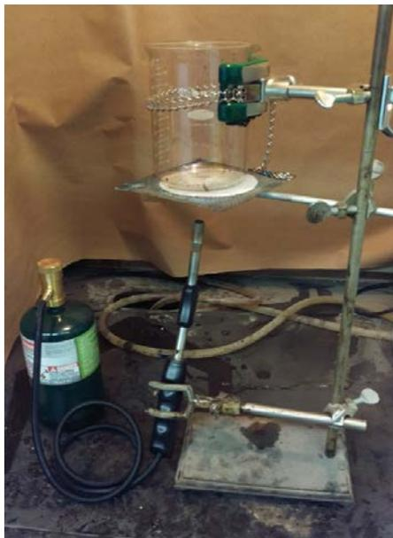
**Figure B-1 Boil testing setup using propane fuel and handheld torch**
