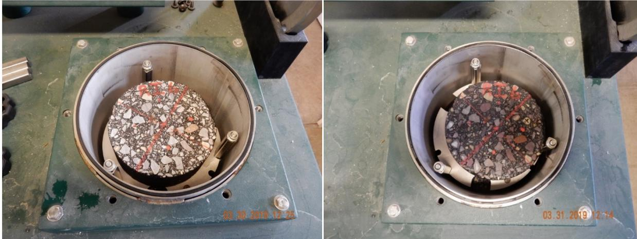
**Figure 4 Specimen before MiST conditioning (L) and after MiST conditioning (R)**
