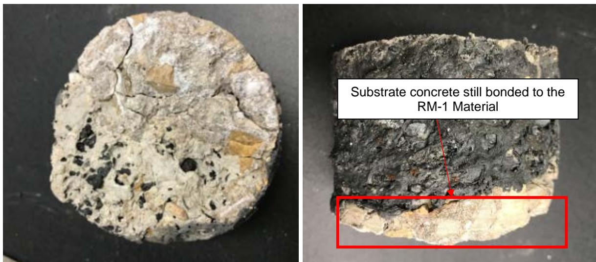
Figure 3-6. Close-up view of the bottom (left) and side (right) of the debonded portion from core #2.
