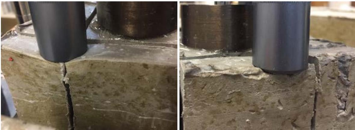
Figure 4-10. RM-4 specimens being crushed by the bond testing equipment at  $23\text{ }^{\circ}\text{C}$ .
