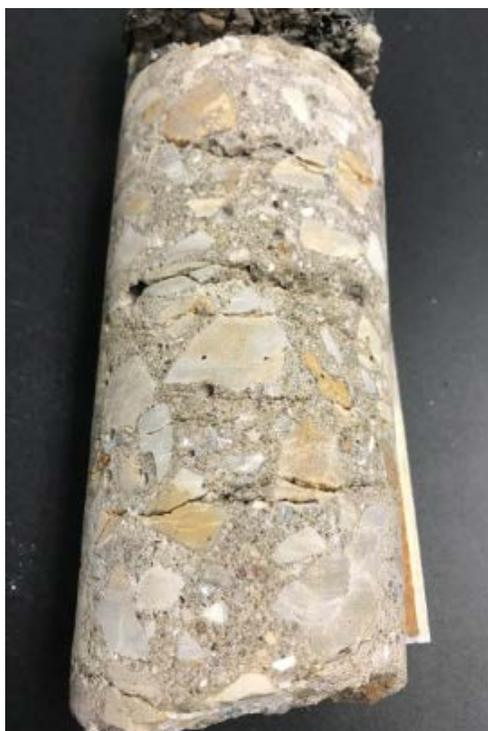
Figure 3-7. Multiple parallel horizontal cracks extending through the entire depth of core #2.
