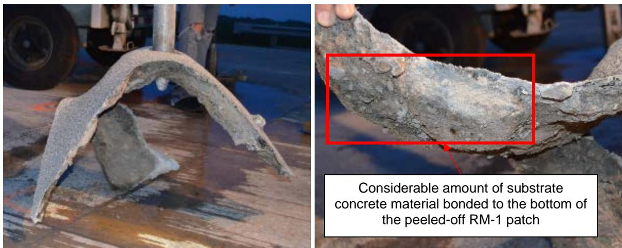
Figure 3-10. RM-1 PDRs peeling off from the concrete pavement.
