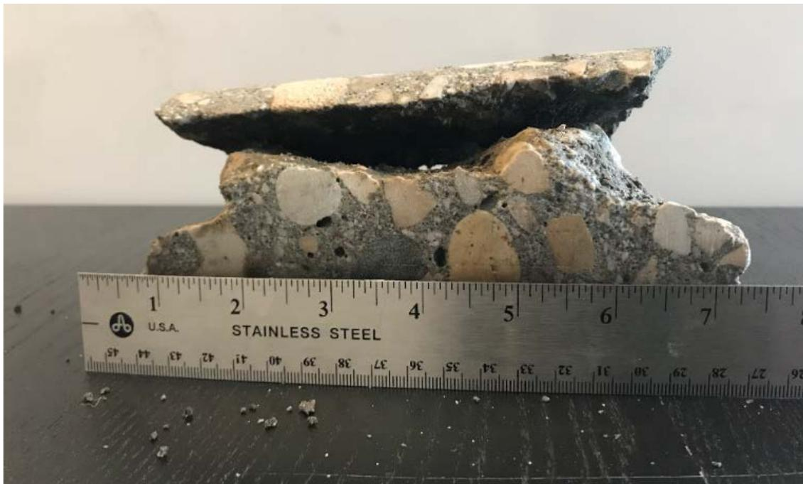
Figure A-16. Site #9, RM-4 Core #1—concrete portion
