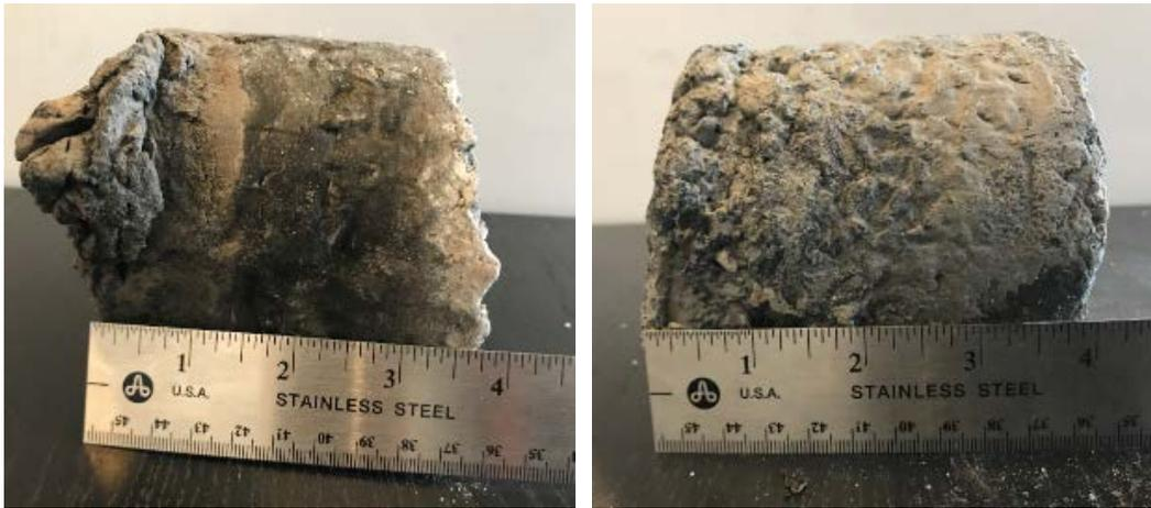
Figure 3-24. RM-5 cores from Site #20 (left) and Site #23 (right).
