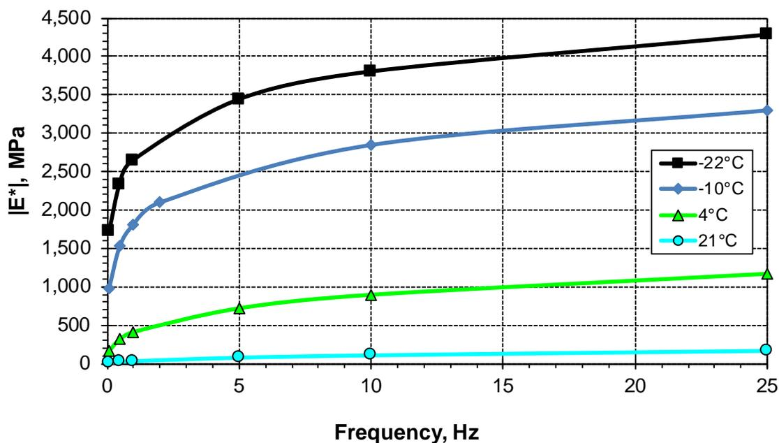
Figure 4-18. Dynamic modulus vs. testing frequency for RM-5.
