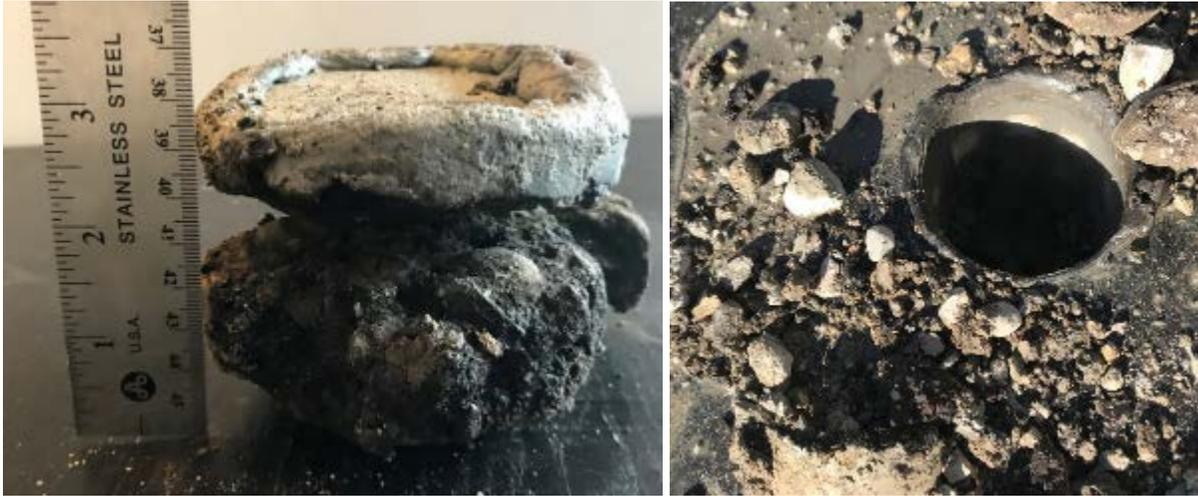
Figure 3-14. RM-3 core from Site #5 (left) and remains of underlying concrete pavement extracted from the core hole (right).
