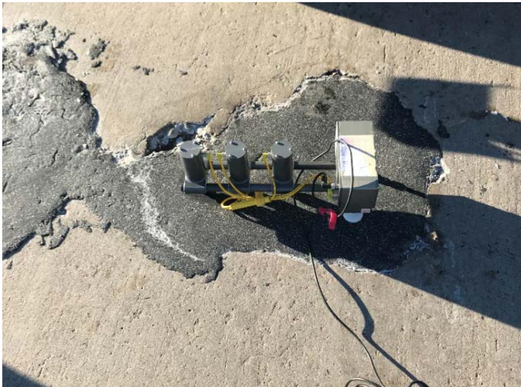
Figure D-10. PSPA testing in progress on PDR in slab interior
