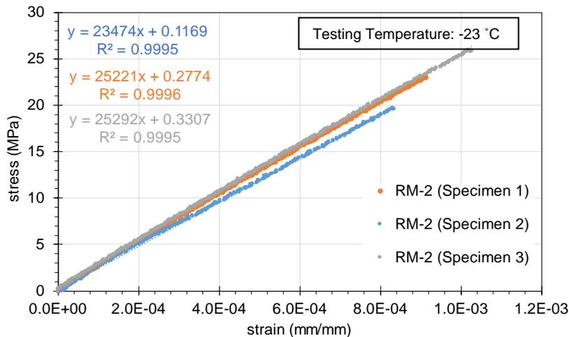
Figure 4-13. Stress-strain response curves for RM-2.
