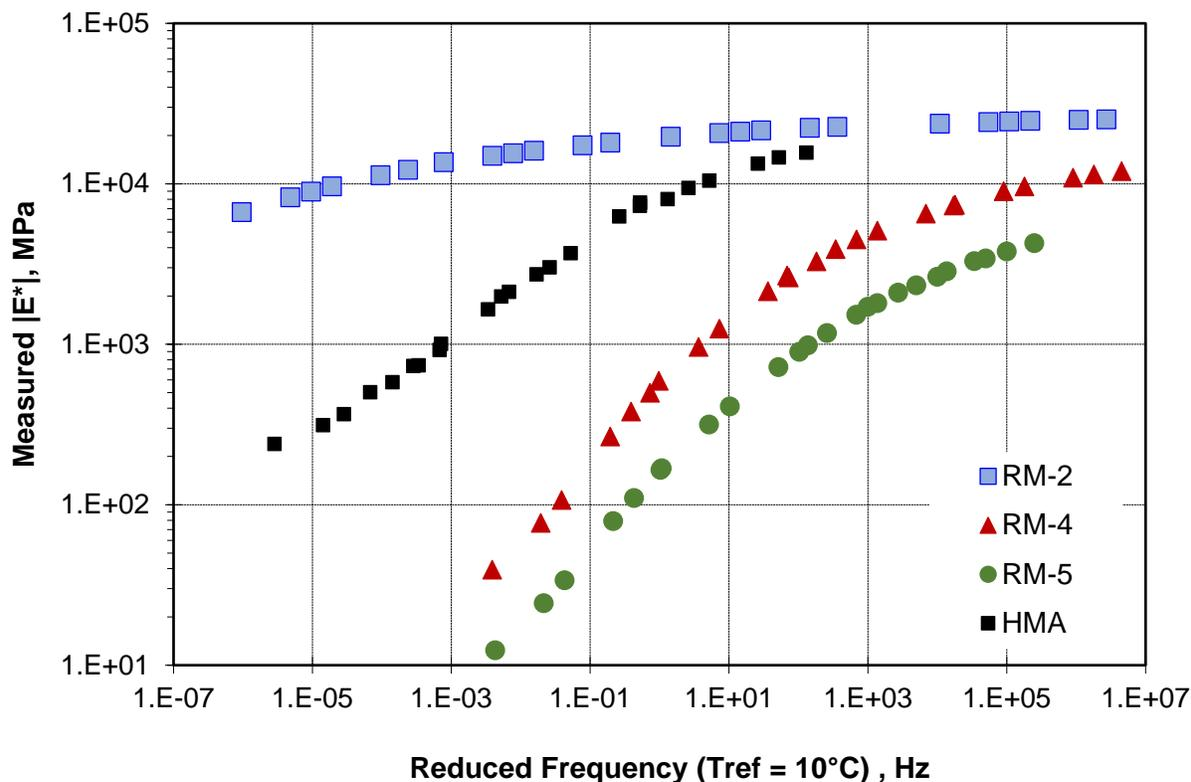
Figure 4-19. Mastercurves developed from dynamic modulus testing.
