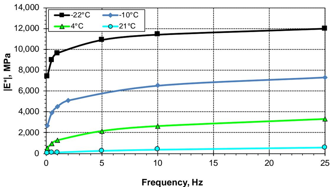
Figure 4-17. Dynamic modulus vs. testing frequency for RM-4.
