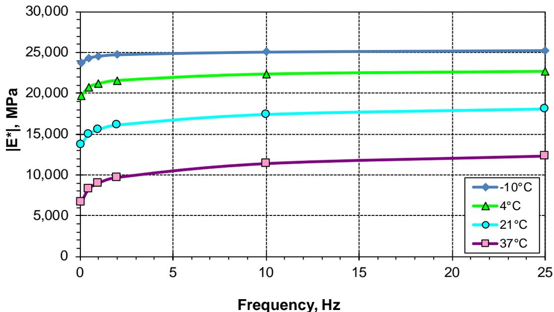
Figure 4-16. Dynamic modulus vs. testing frequency for RM-2.
