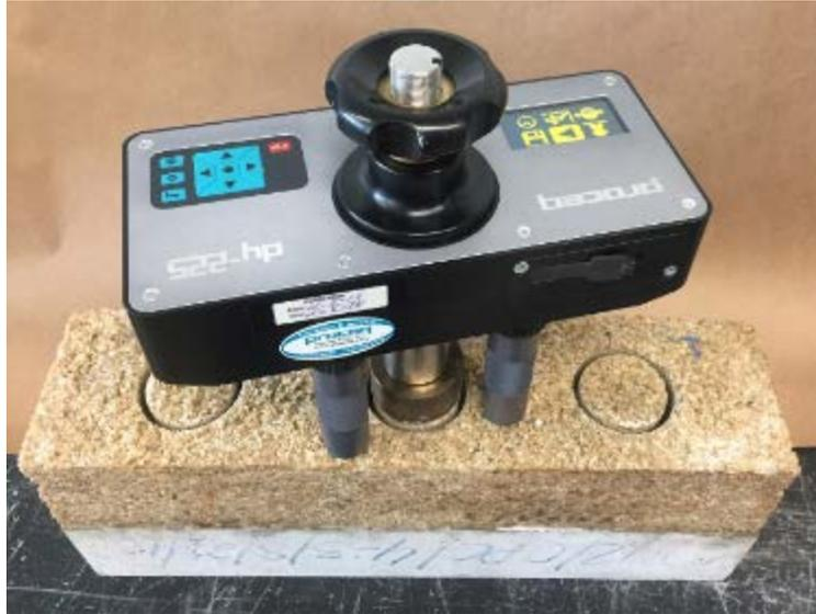
Figure 4-7. RM-2 specimen prepared for bond testing.
