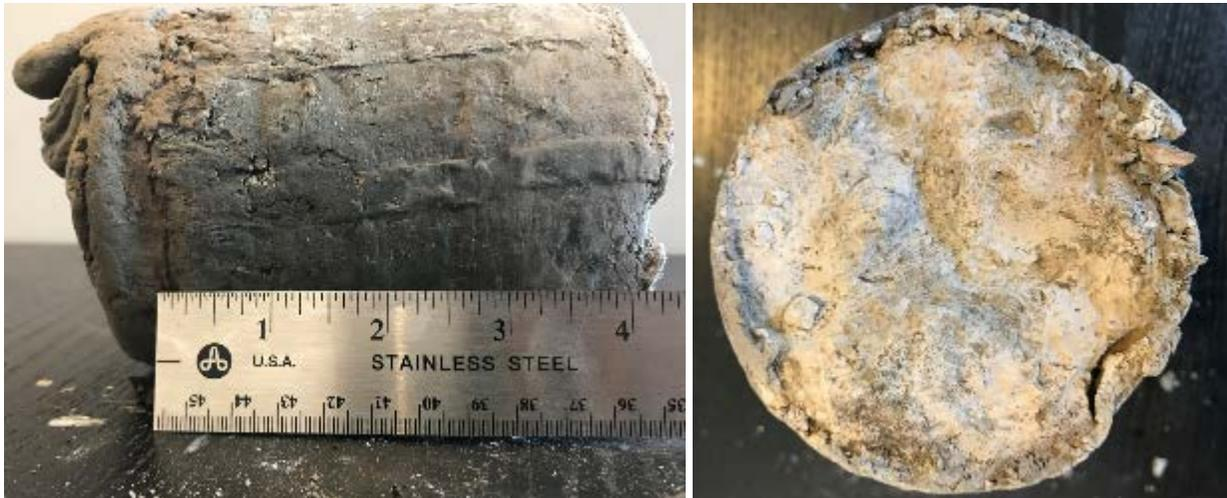
Figure 3-18. RM-4 core from Site #11 (left) and bottom of the core showing substrate concrete material bonded to the repair material (right).
