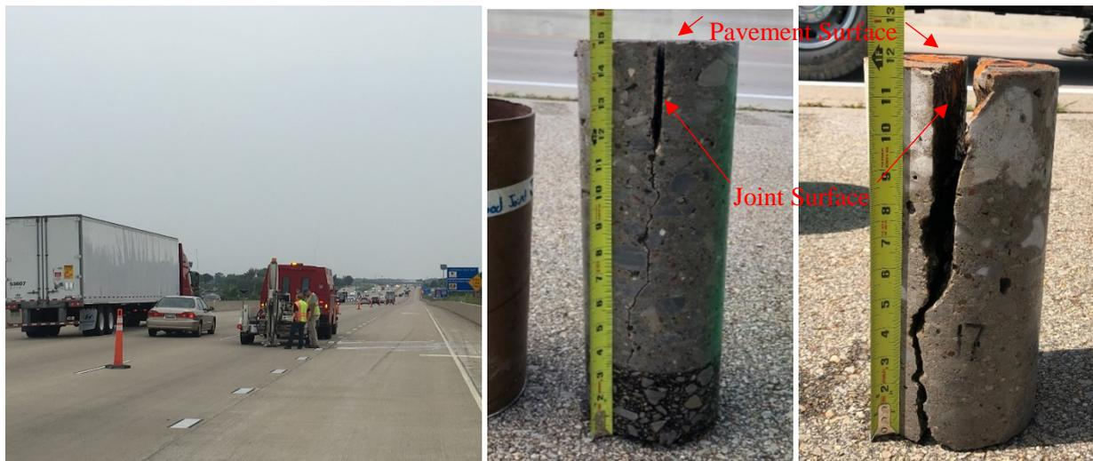
**Figure 3.2 (a) Taking field cores (b) A core sample of good joint (c) A core sample of spalled joint**
