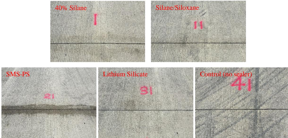
**Figure 5.2 Appearance of Joints Right After Sealer Applied**
