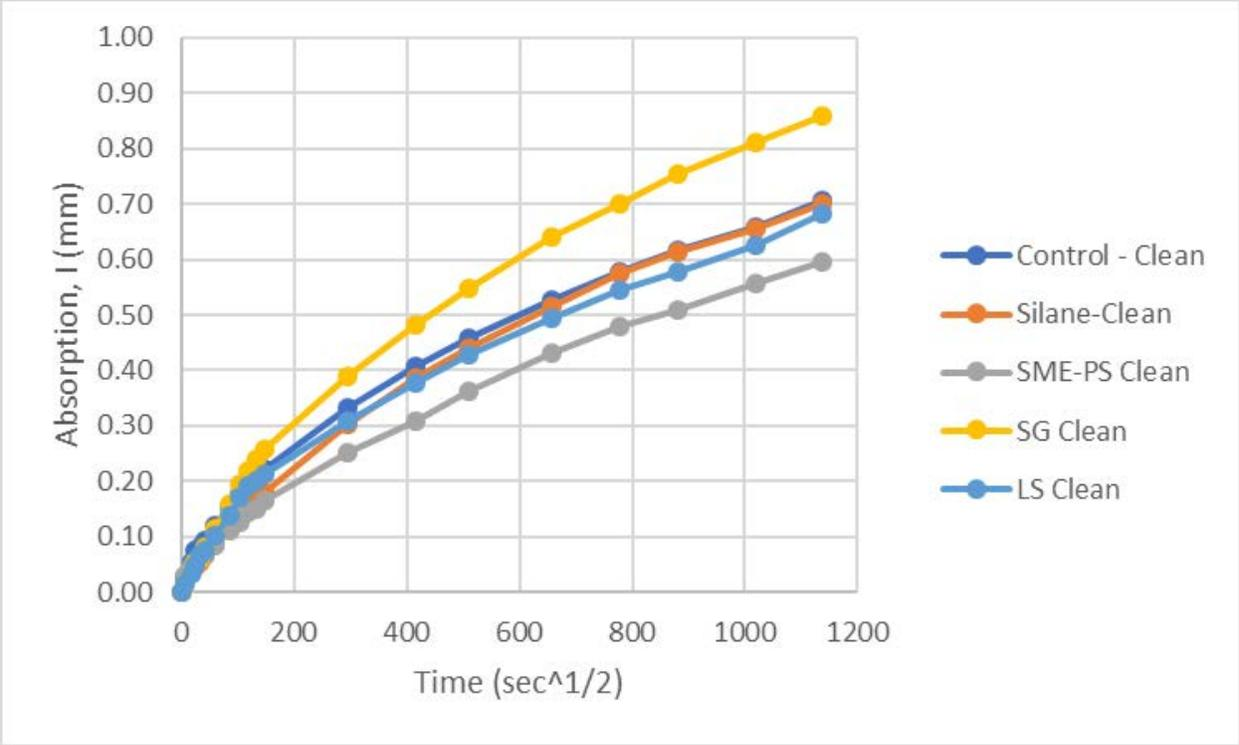
Figure F.12 I-39 Average Clean Core Absorption
