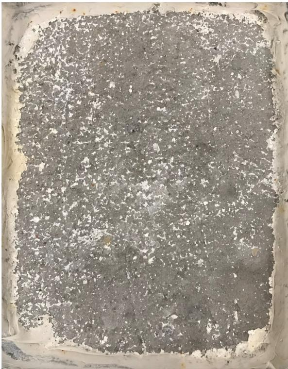
**Figure C.5 FA Silane applied dry after 50 Cycles**
