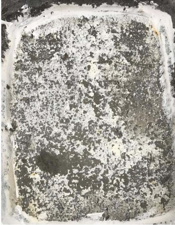
**Figure C.4 FA Control after 50 Cycles**
