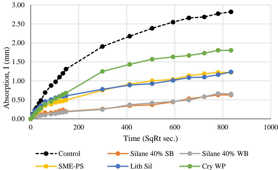
**Figure 4.1 Absorption Results for Initial Penetrating Sealer Products**
