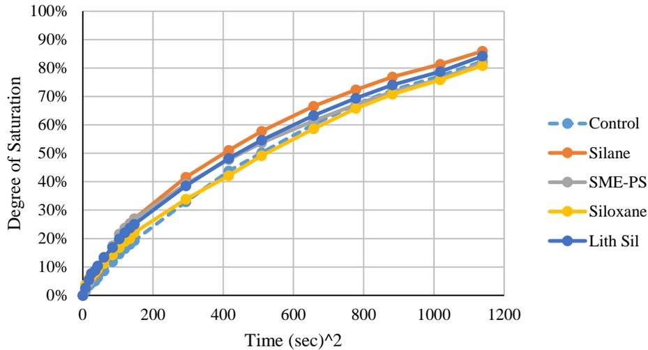
Figure 5.11 Absorption Performance of I-39 Core Samples
