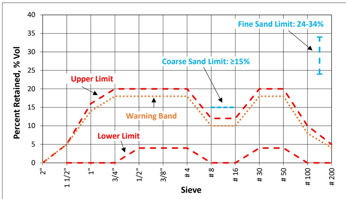
Figure 30: Tarantula Curve guidelines for workable mixtures.
