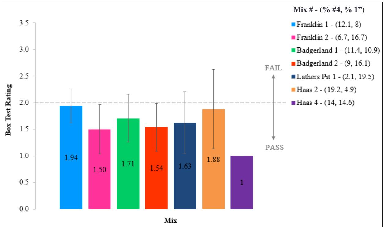
Figure 23: Average Box Test Results from Part II.
