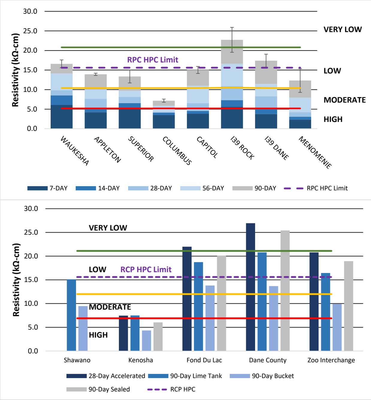
Figure 83: Phase I and II Resistivities Compared to the Rapid Chloride Penetration High Performance Concrete Equivalent Surface Resistivity Specification.
