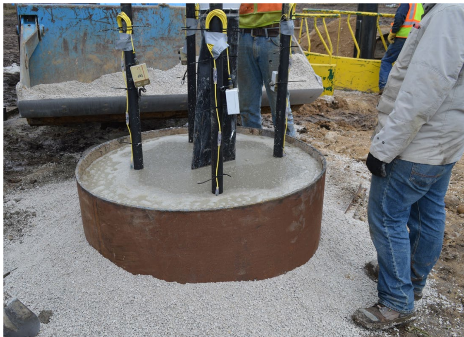
Figure 35: Completed Test Shaft 1 shortly after completion of concrete placement. Bleed water from the weak concrete of Defect 6 is evident at the top of the shaft.
