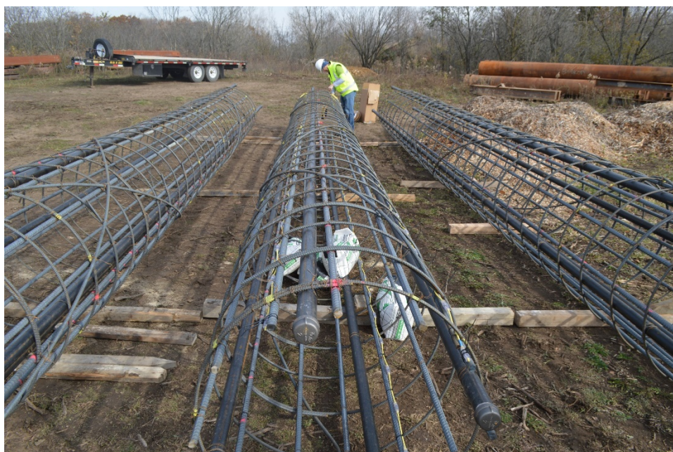
Figure 21: Reinforcing cages prior to installation of most defects.
