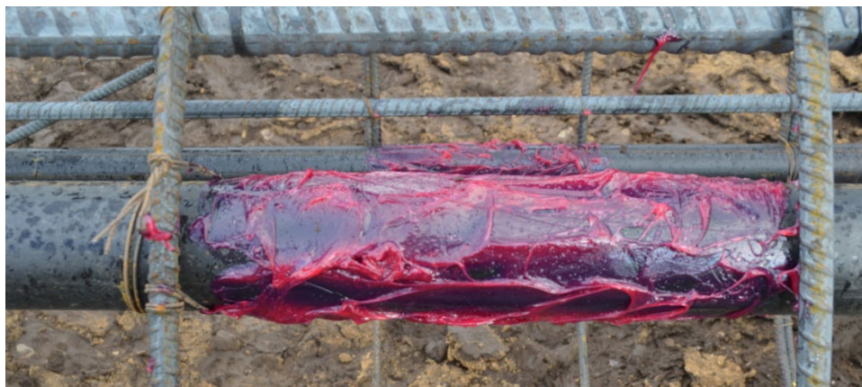
Figure 25: Defect 4 consisted of wheel bearing grease applied around the outside of the access tubes for a length of 1 ft. Defect 4 was installed in two locations: at a depth of 16.5 ft in Test Shaft 1 and a depth of 4.5 ft in Test Shaft 2.
