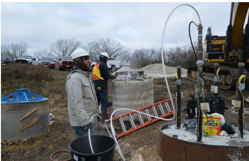
Figure 40: The access tubes were dewatered prior to performing TIP test via probe method.
