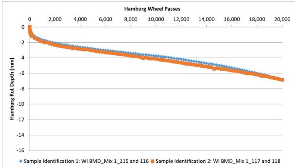
**Figure C1 Hamburg Rut Depth versus Number of Cycles – Mix 1 (4.0% Design Air, Top – 3.5% Design Air, Middle – 3.0% Design Air, Bottom)**
