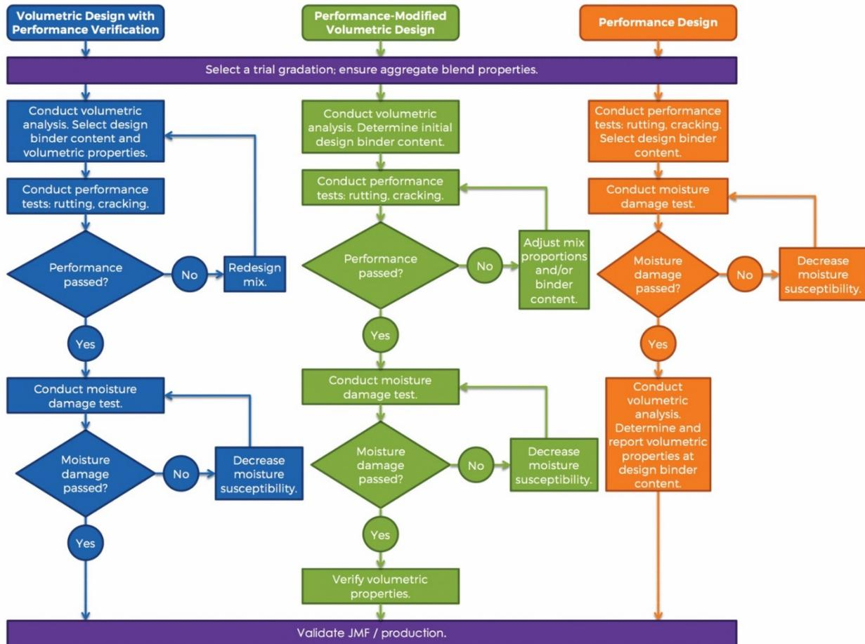
**Figure 4 Schematic Illustrations of Three BMD Approaches (NCAT, 2017)**
