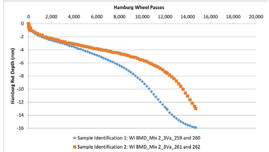
**Figure C2 Hamburg Rut Depth versus Number of Cycles – Mix 2 (4.0% Design Air, Top – 3.5% Design Air, Middle – 3.0% Design Air, Bottom)**
