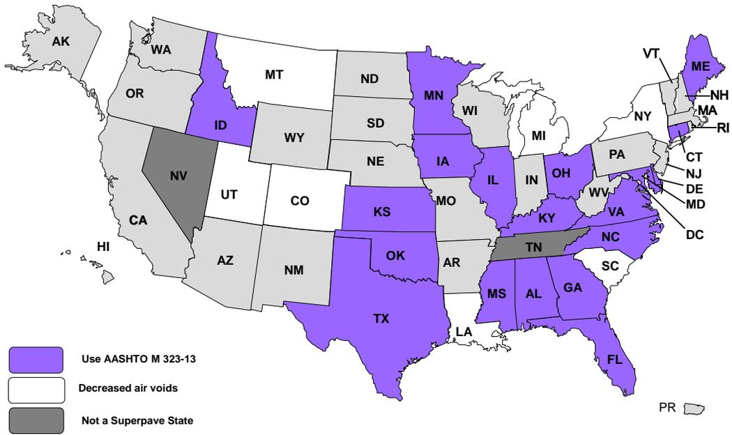
**Figure 1 Design Target Air Voids (Aschenbrener, 2014)**
