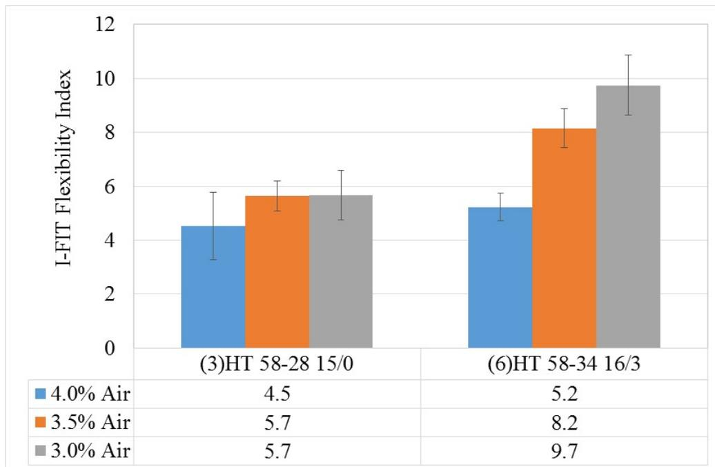
**Figure 13 I-FIT Flexibility Index for High Traffic Mixes**
