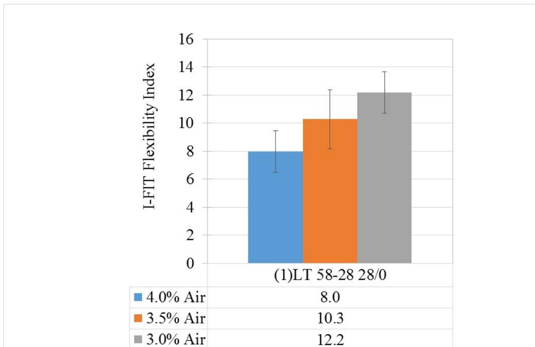
**Figure 11 I-FIT Flexibility Index for Low Traffic Mixes**
