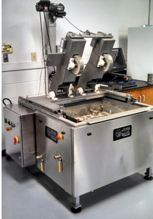
**Figure 8 Hamburg Wheel-Tracking Device**
