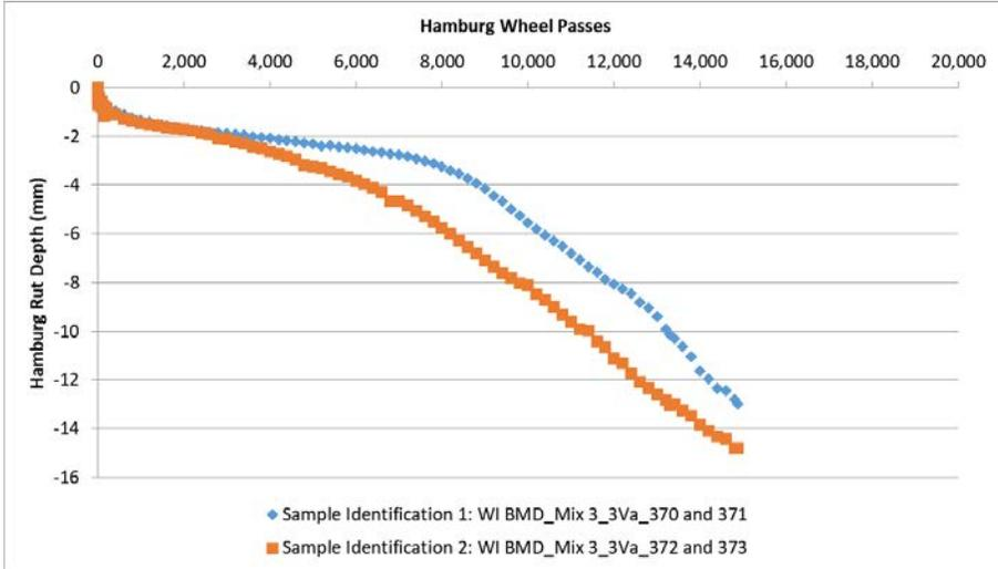
**Figure C3 Hamburg Rut Depth versus Number of Cycles – Mix 3 (4.0% Design Air, Top – 3.5% Design Air, Middle – 3.0% Design Air, Bottom)**
