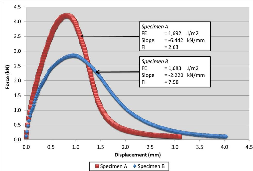
**Figure 7 Example of Raw Data from I-FIT Test**
