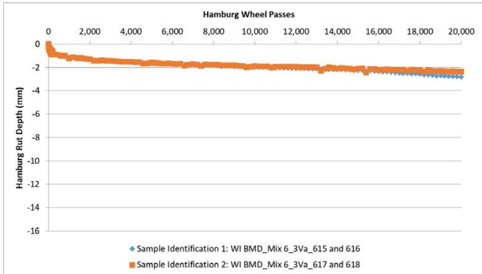
**Figure C6 Hamburg Rut Depth versus Number of Cycles – Mix 6 (4.0% Design Air, Top – 3.5% Design Air, Middle – 3.0% Design Air, Bottom)**
