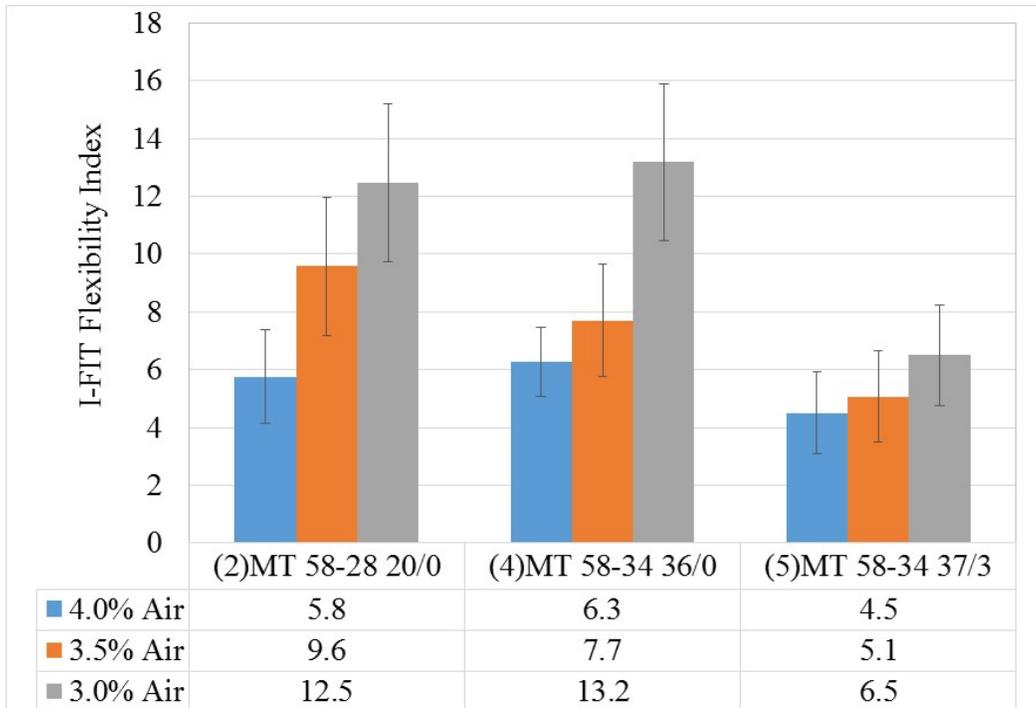
**Figure 12 I-FIT Flexibility Index for Medium Traffic Mixes**
