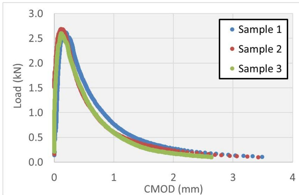
**Figure 7 Example Load versus CMOD Data – DCT Test**
