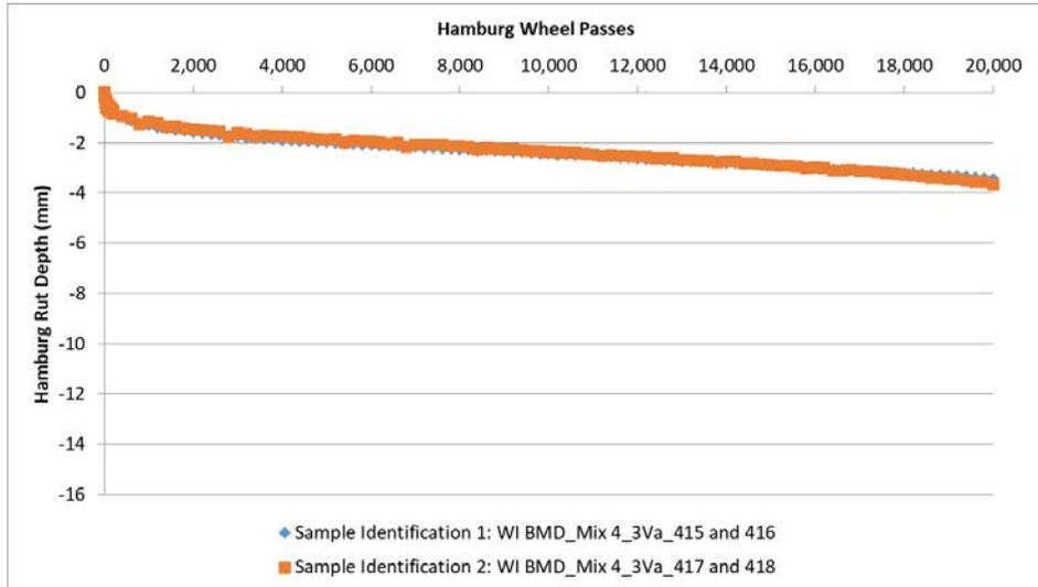
**Figure C4 Hamburg Rut Depth versus Number of Cycles – Mix 4 (4.0% Design Air, Top – 3.5% Design Air, Middle – 3.0% Design Air, Bottom)**
