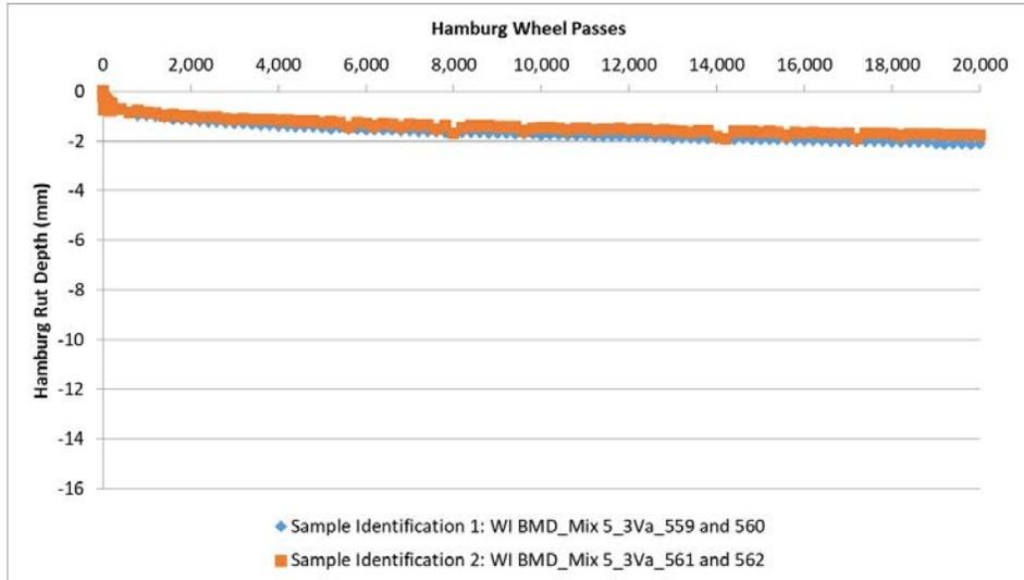
**Figure C5 Hamburg Rut Depth versus Number of Cycles – Mix 5
