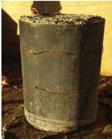
Figure 4.5. “Stress free” concrete cylinder.
