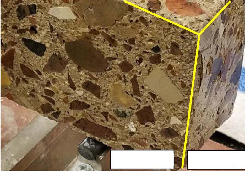
**Figure 4.4.2. Paste Deterioration and Erosion**
