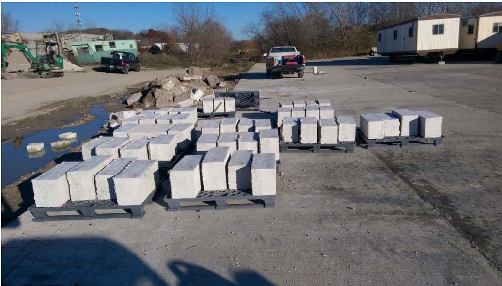
**Figure 2.6.4. Pallets of Joint Specimens Ready for Wrapping**
