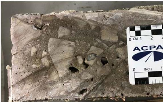
**Figure 4.5.4. Chloride Penetration of the Best Performing Limestone Mixture (L17)**
