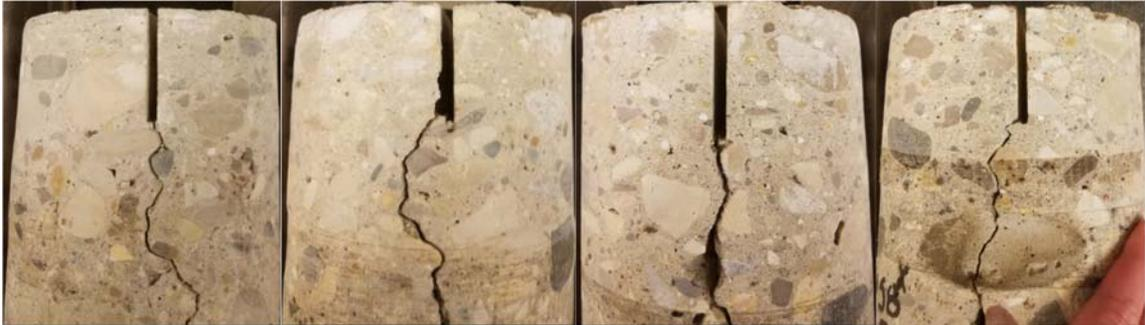
**Figure 4.2.14. Core Samples Sawed to a Depth of 2.0 in. (D/4)**
