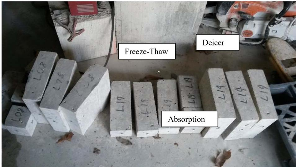
**Figure 3.1.4. Final Sample Size Before Testing**
