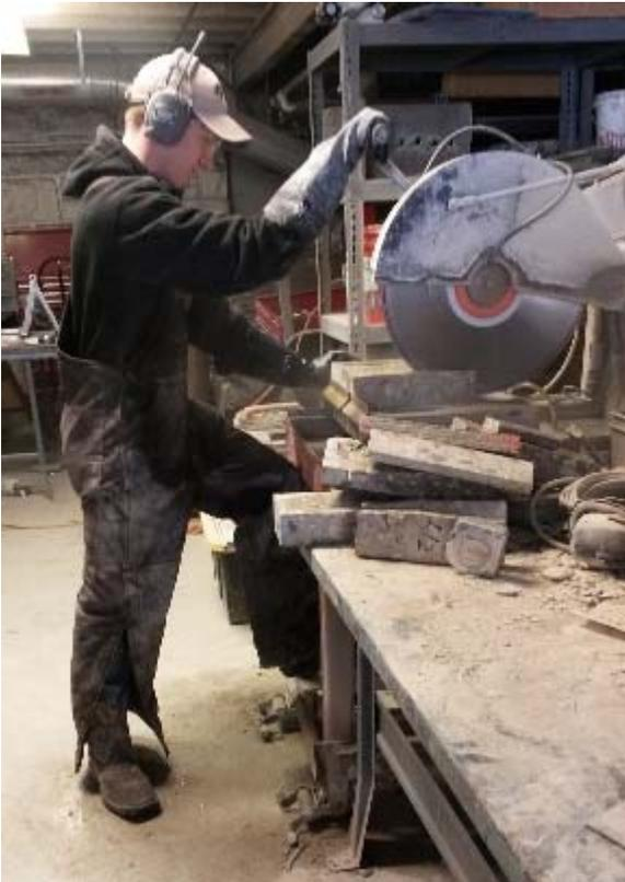
**Figure 3.1.2. Final Sizing on Concrete Slab Saw**
