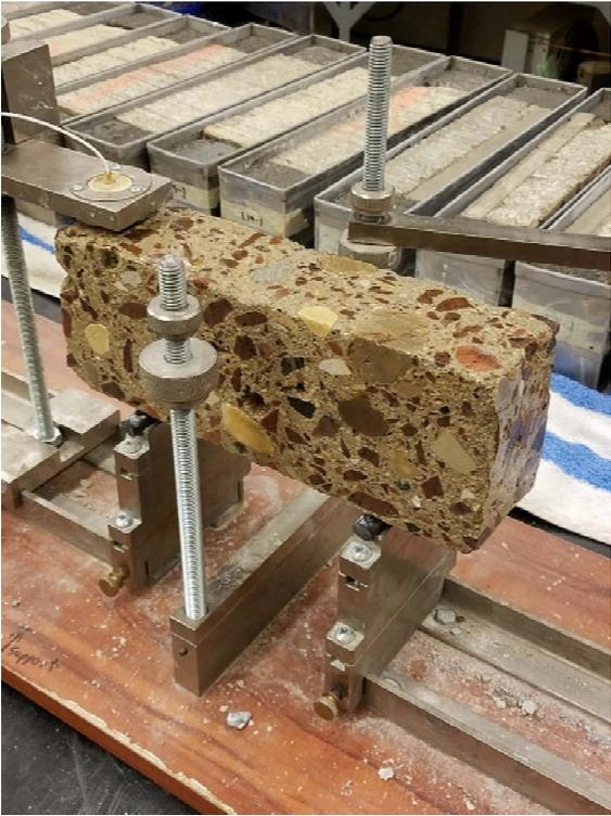
**Figure 3.3.1. Dynamic Modulus Testing**
