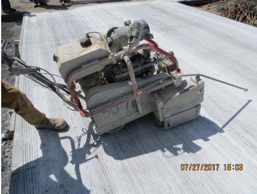
**Figure 2.10.13. Husqvarna SOFF-CUT Model 4000 Early Entry Saw**
