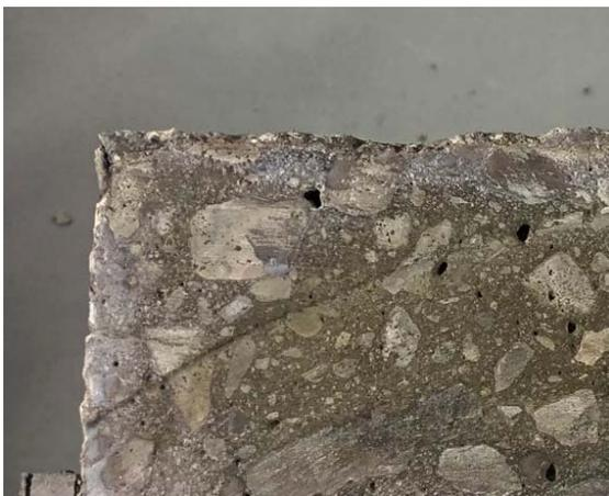
**Figure 4.5.7. Chloride Penetration of Silane-Coated (Ls16)**
