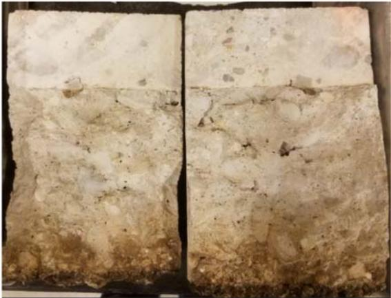
**Figure 4.2.16. Core Samples Sawed to a Depth of 2.0 in. (D/4)**
