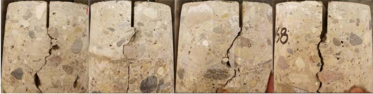
**Figure 4.2.13. Core Samples Sawed to a Depth of 1.5 in.**
