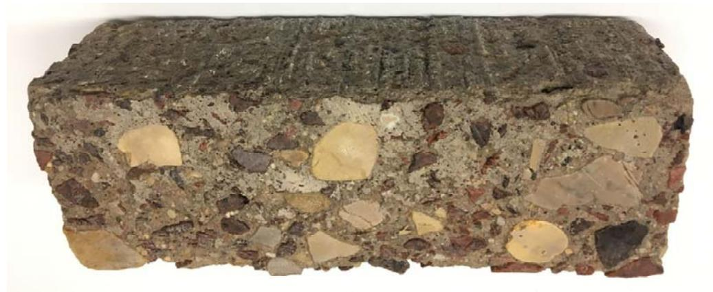
**Figure 4.4.11. Granite Mixture G06 after 600 Freeze-Thaw Cycles**
