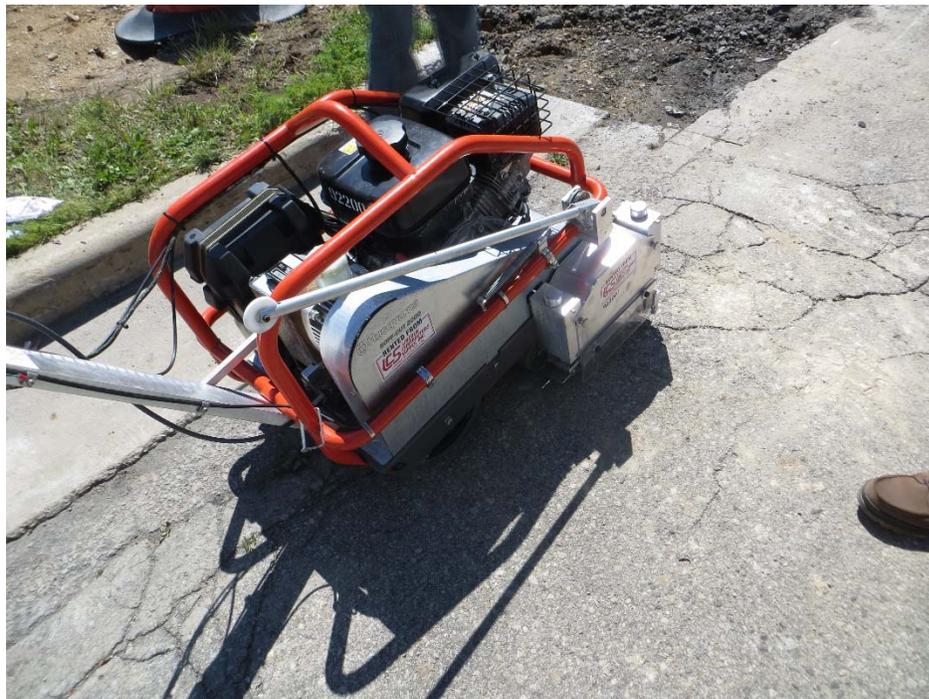
**Figure 2.10.11. Husqvarna SOFF-CUT Model 2000 Early Entry Saw**
