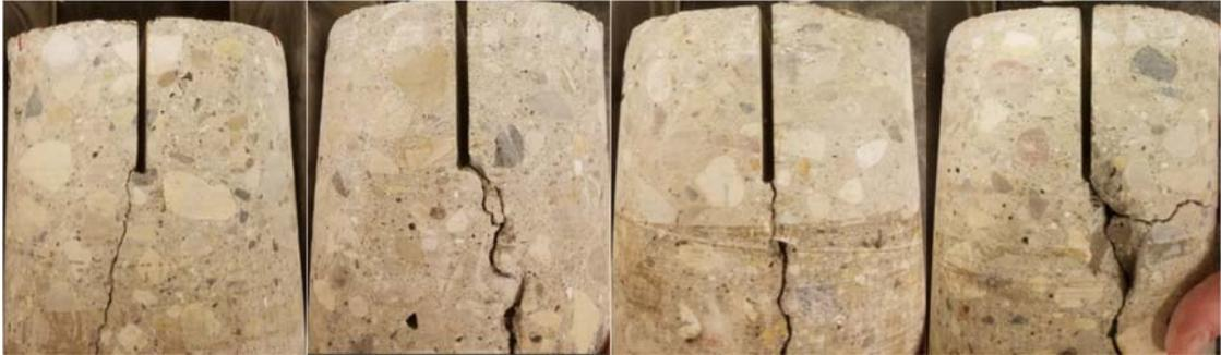
**Figure 4.2.15. Core Samples Sawed to a Depth of 2.67 in. (D/3)**
