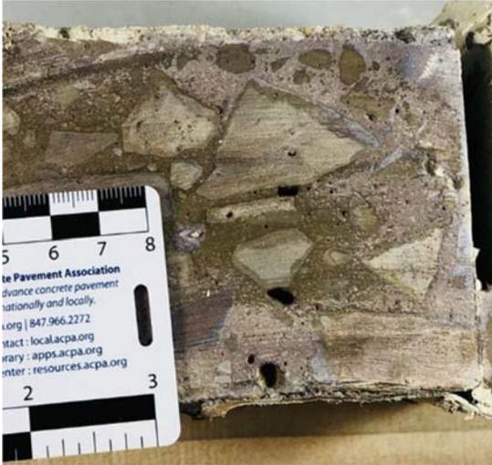
**Figure 4.5.5. Chloride Penetration of Silane Coated Mixture (Ls17)**
