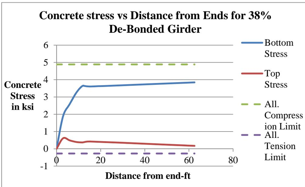
Figure 6-4. Bottom and top concrete stresses in 38% de-bonded girder.
