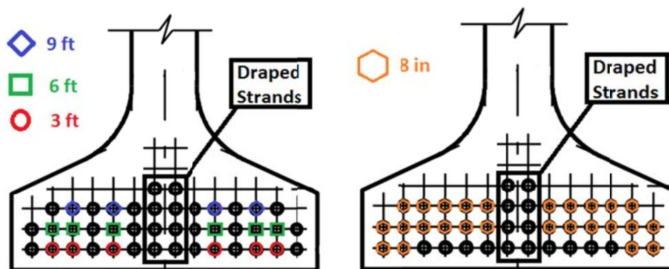
Figure 6-7. 38% debonded girder with staggered pattern (left with debonded lengths shown by symbols) and 62% debonded girder with 8in debond length (right).
