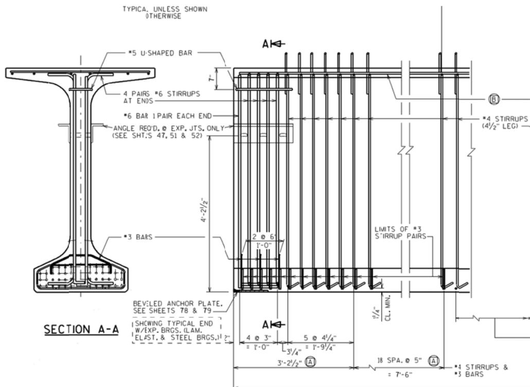
Figure 5-1. 72W cross section and reinforcement details of end zone.
