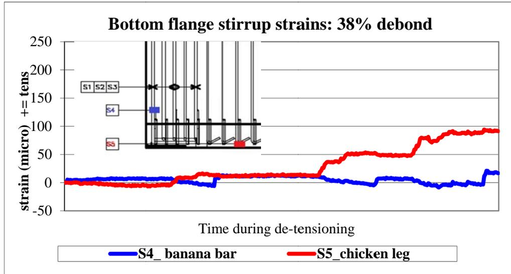
Figure 6-19. The test strain results for S4 (on banana bar) and S5 (on chicken leg bar) stirrups for 38% de-bonded girder. (*positive is tension*)
