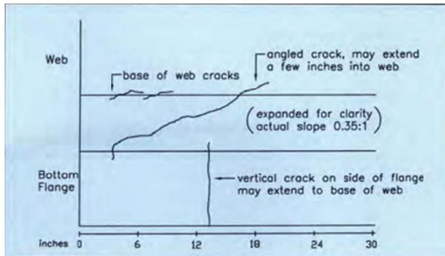
Figure 2-4. Types of crack observed (6).
