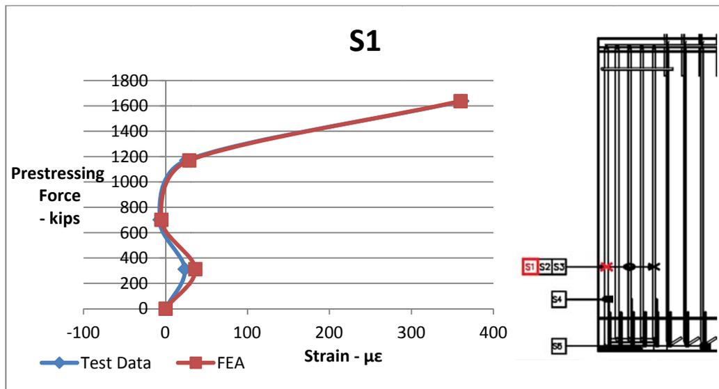
Figure 6-51. Re-bar strain comparisons between data obtained from strain gauge 1 and finite element model during prestress release for 62% de-bonded girder. (positive = tension)
