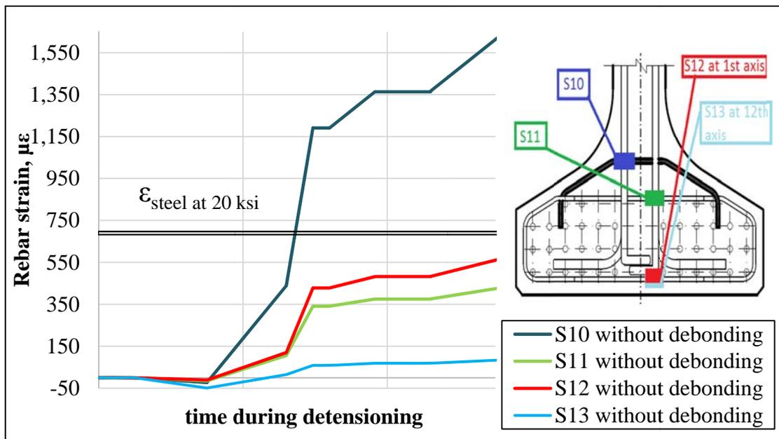
Figure 5-19. Bonded girder: Strain change of reinforcing bars in bottom flange (gauges S10 – S13). (Tension positive, compression negative)
