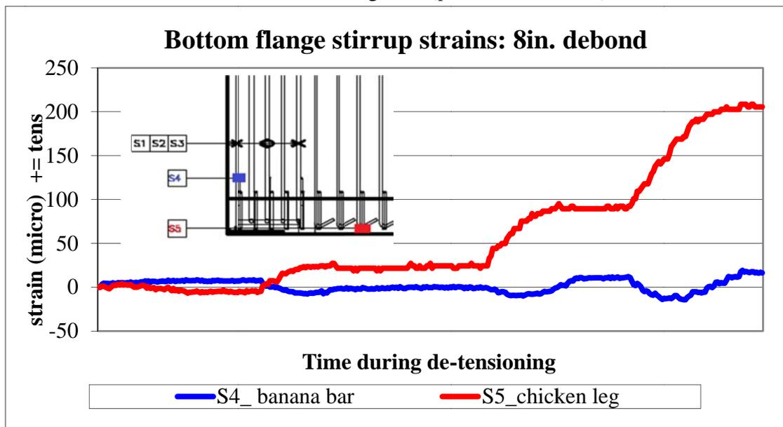
Figure 6-20. The test strain results for S4 (on banana bar) and S5 (on chicken leg bar) stirrups for 8in. de-bonded girder. (*positive is tension*)
