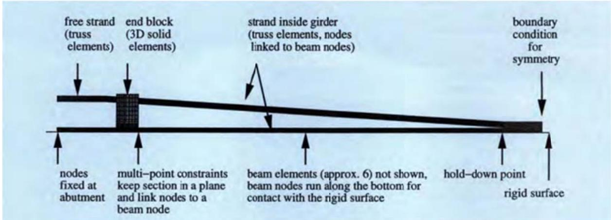
Figure 2-5. The FEA model created by Kannel et al. (6).
