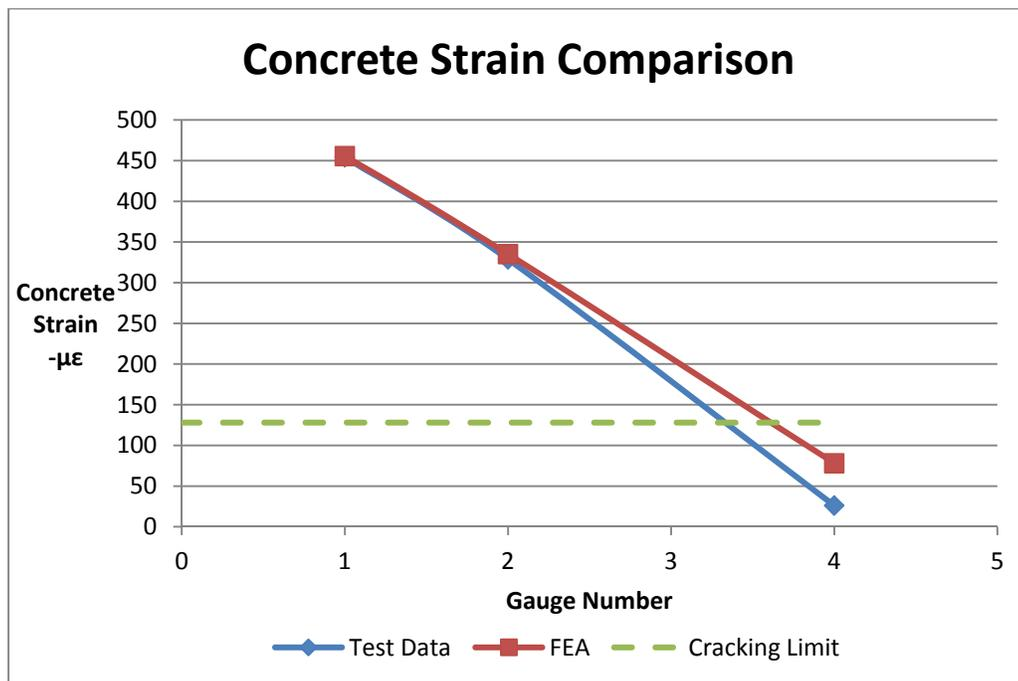
Figure 5-33. Concrete strain comparison for de-bonded girder.
