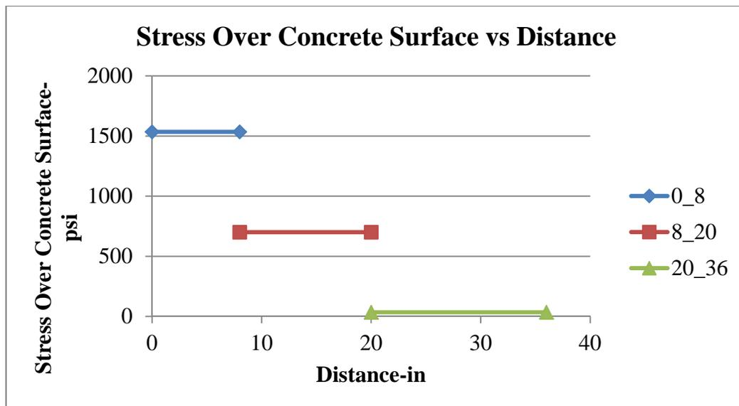
Figure 4-10. Surface traction force applied to concrete elements in models for 72W Girder.
