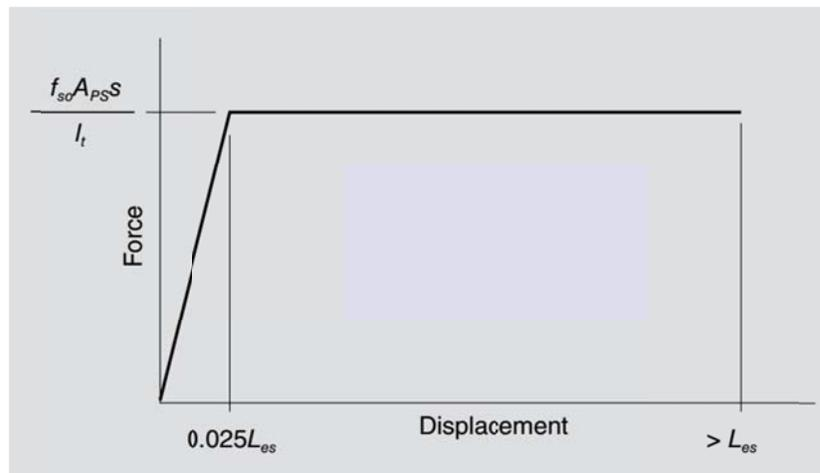
Figure 2-6. Nonlinear spring force-versus-displacement curve. (Note:  $A_{ps}$ : area of pre-stressing strand;  $f_{s0}$ : stress in strand just after transfer;  $l_t$ : transfer length;  $L_{es}$ : end slip; and  $s$ : nonlinear spring spacing) (7).
