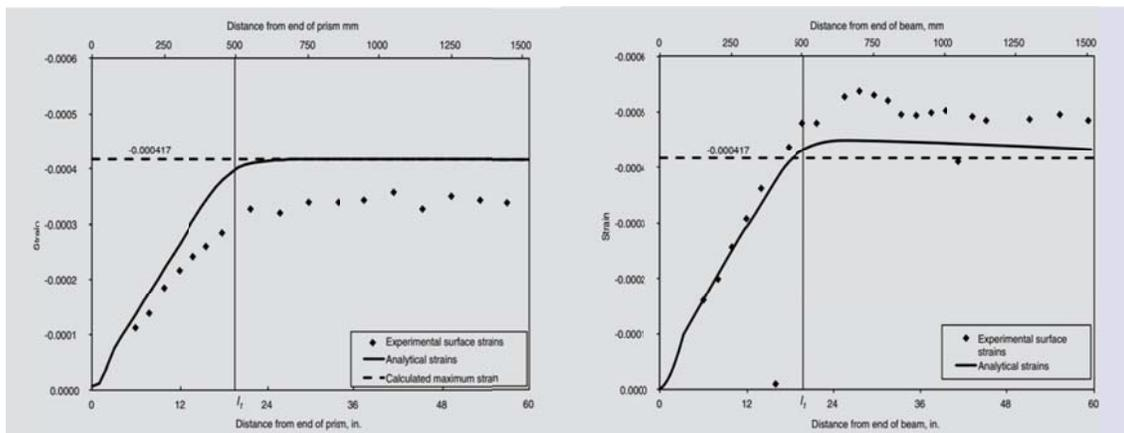
Figure 2-8. Comparison of experimental concrete surface strains and analytical concrete strains for a prism (left) and a typical T beam model (right) (7).
