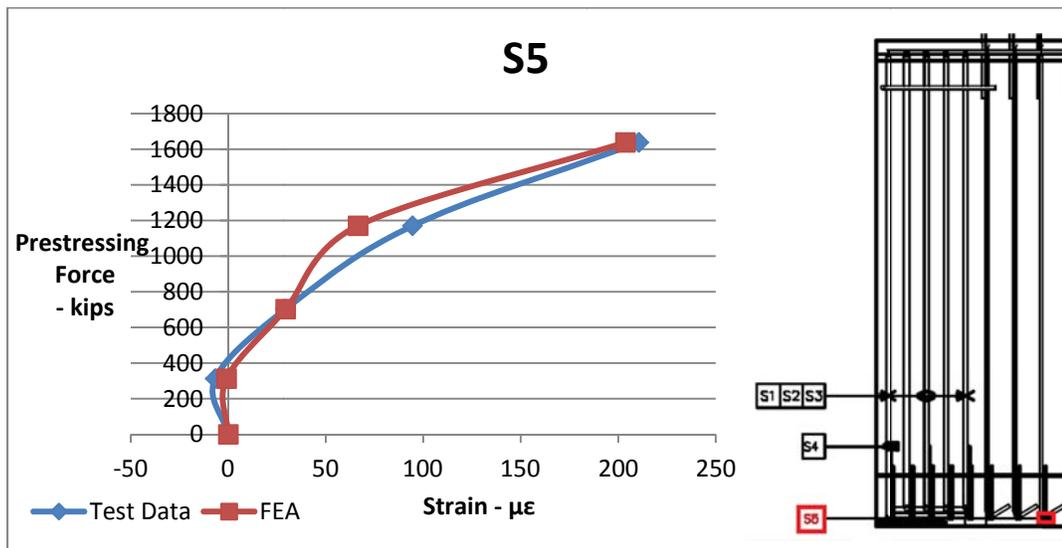
Figure 6-55. Re-bar strain comparisons between data obtained from strain gauge 5 and finite element model during prestress release for 62% de-bonded girder. (positive = tension)
