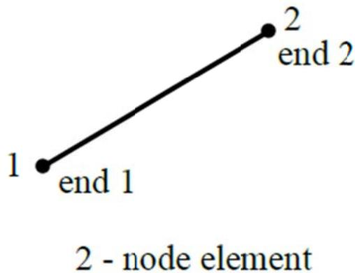
Figure 4-12. 2 Node linear Truss elements
