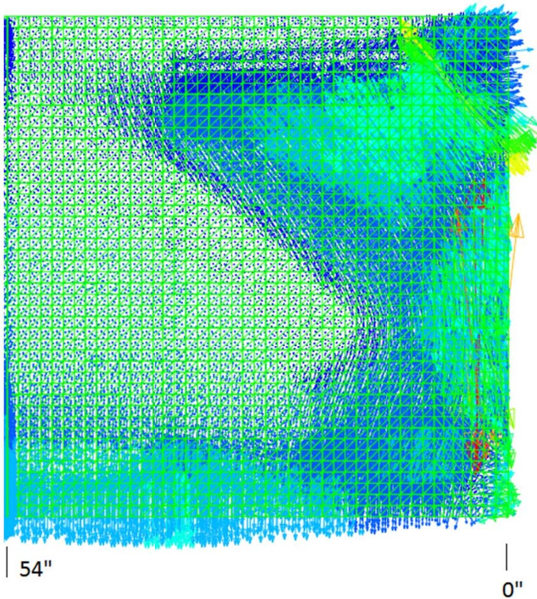
Figure 7-2. Principal tensile strains directions – 0" is the girder end.
