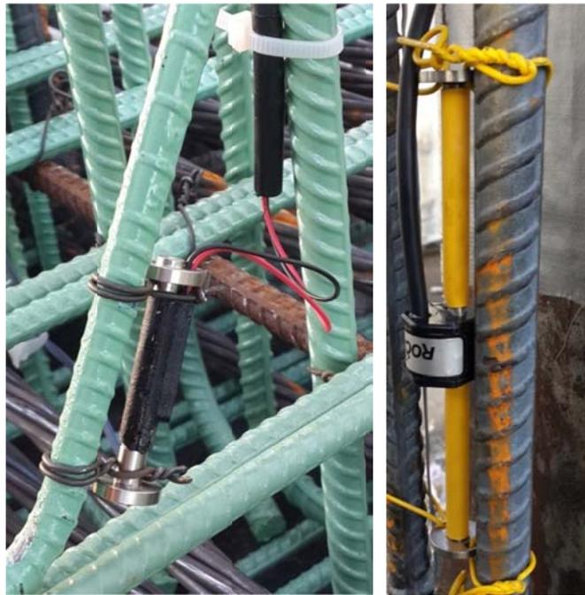
Figure 6-11. The 2in. (left) and 6in. (right) vibrating wire gauges.
