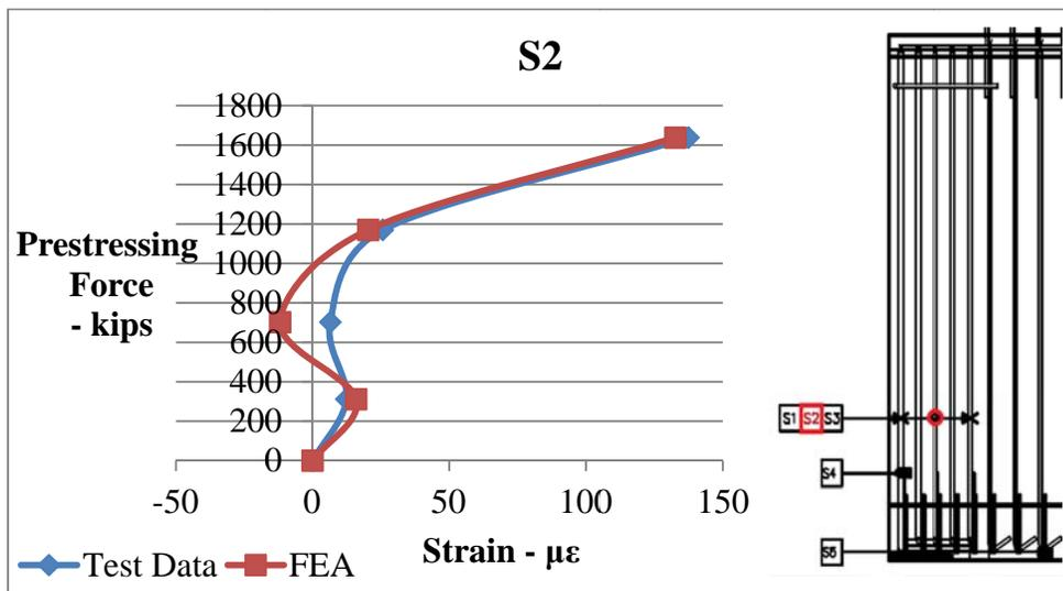
Figure 6-36. Re-bar strain comparisons between data obtained from strain gauge 2 and finite element model during prestress release for bonded girder. (positive = tension)
