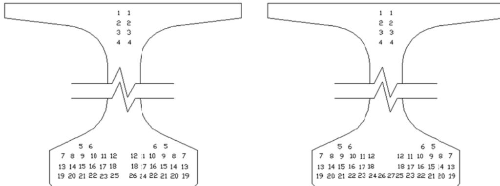
Figure 5-6. Strand cutting order for bonded girder (left) and debonded girder (right).
