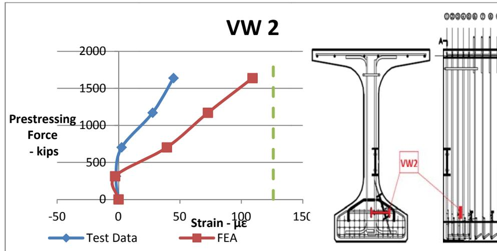
Figure 6-48. Concrete strains comparisons between data obtained via VW gauge 2 and finite element model during prestress release for 62% de-bonded girder. (*positive = tension*)
