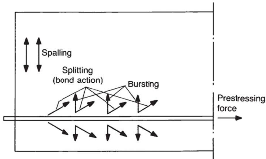
Figure 2-1. Three mechanism in FIB 2010 model code in anchorage zone (4).
