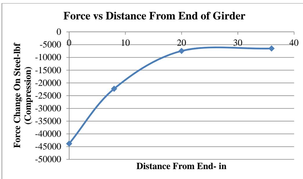
Figure 4-8. Measured prestressing force change in strand versus distance from end for 72W girder.
