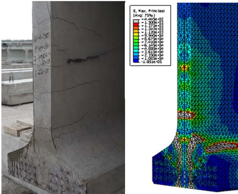
Figure 5-29. The comparison of actual girder end cracking with Abaqus model strains for bonded girder. (*tension is negative*)
