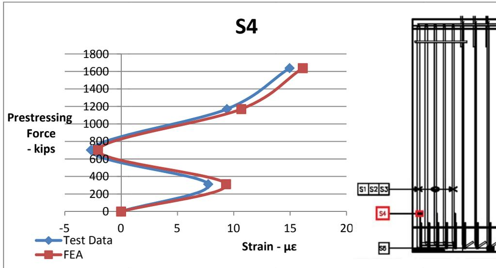
Figure 6-54. Re-bar strain comparisons between data obtained from strain gauge 4 and finite element model during prestress release for 62% de-bonded girder. (positive = tension)
