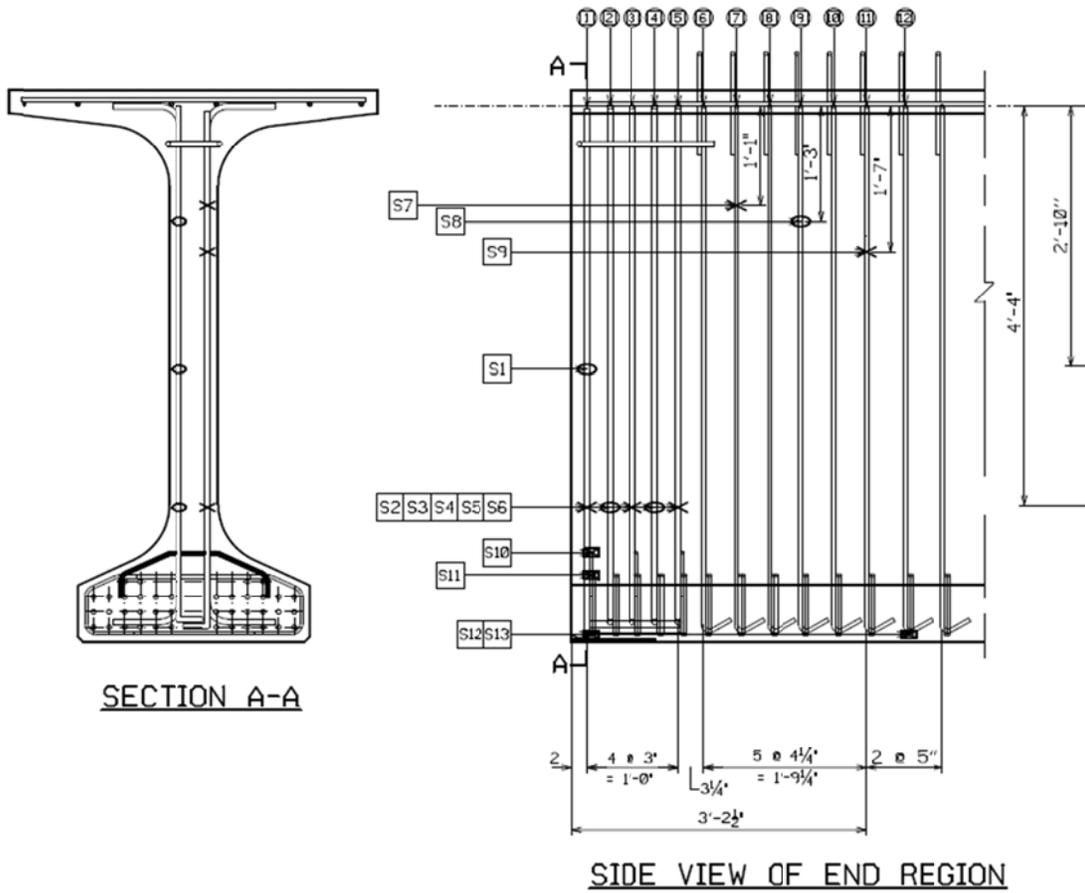
Figure 5-8. Locations of strain gauges at re-bars.
