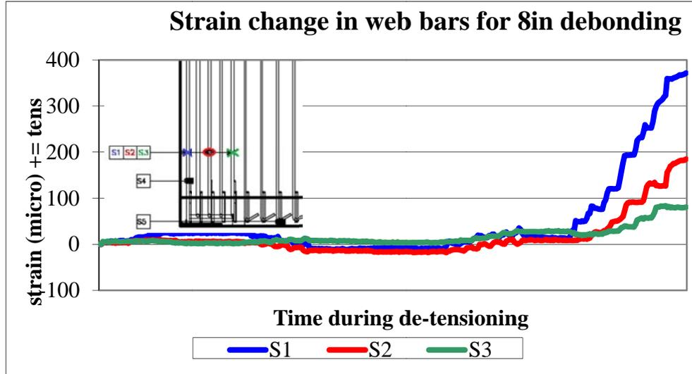
Figure 6-17. The test results of web bar gauges S1, S2, and S3 for debonded 8in. girder.
