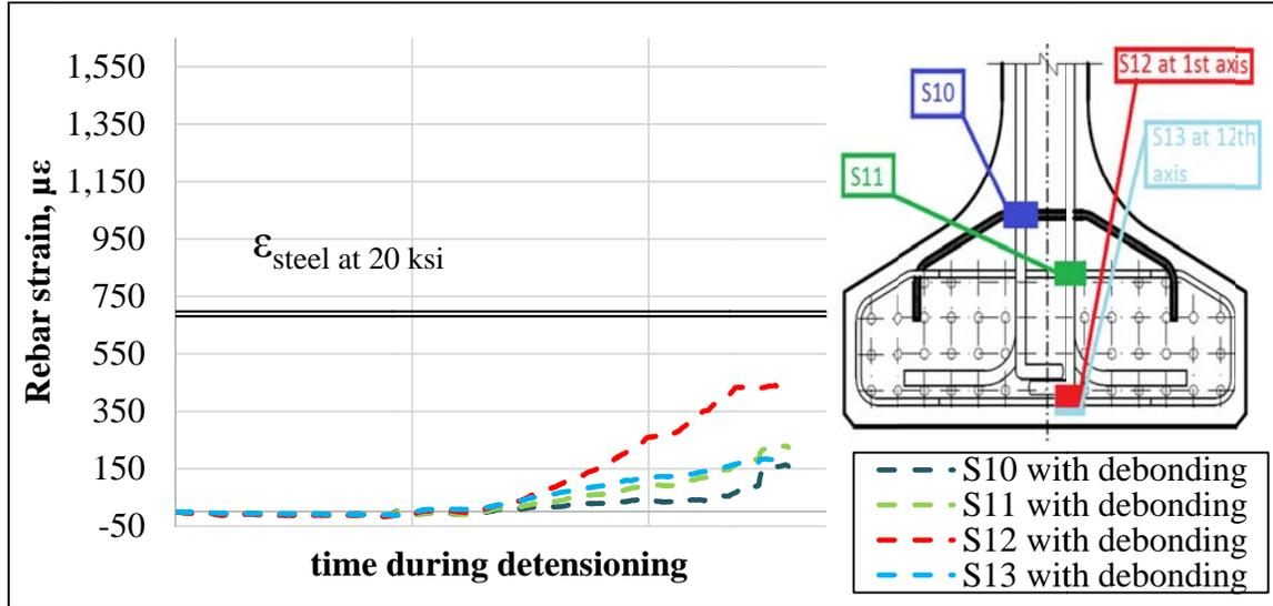
Figure 5-20. Debonded girder: Strain change of reinforcing bars in bottom flange (gauges S10-13). (*Tension positive, compression negative*)
