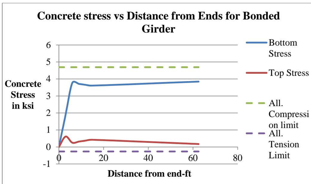
Figure 6-3. Bottom and top concrete stresses in bonded girder.
