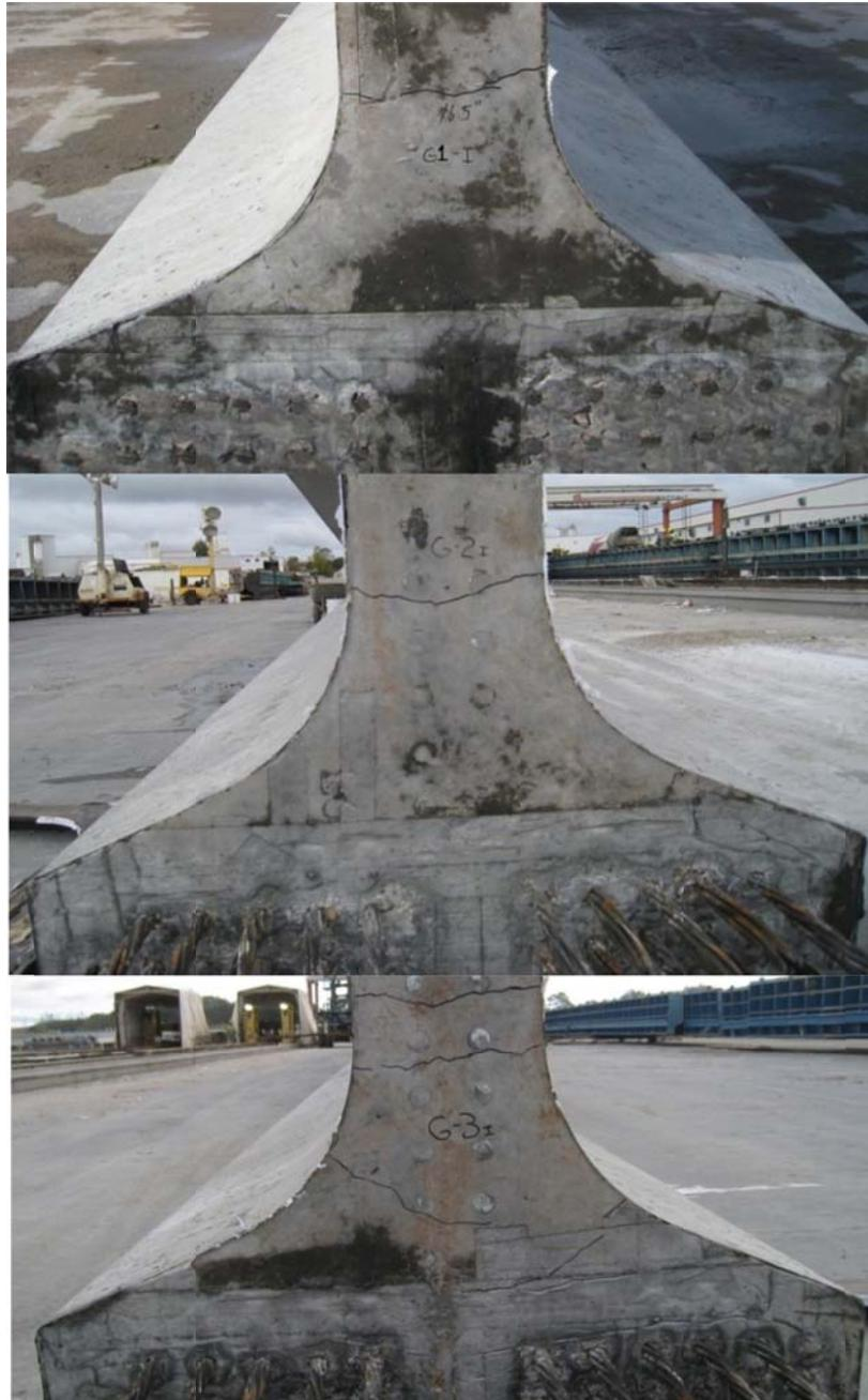
Figure 6-26. Close-up picture of bottom flange for bonded (top), 38% de-bonded (middle), and 8in. debonded (bottom) girders.
