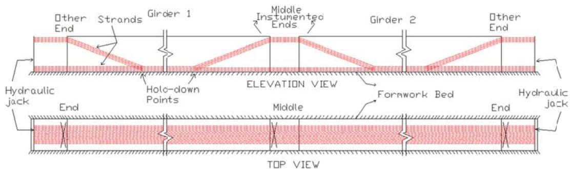
Figure 6-29. Plan of de-bonded girders in the same formwork bed.
