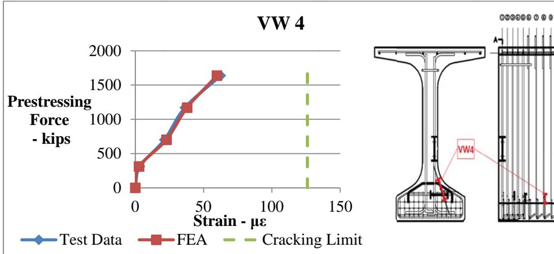
Figure 6-43. Concrete strain comparison between data obtained by VW gauge 4 and finite element model during prestress release for 38% de-bonded girder. (*positive = tension*)
