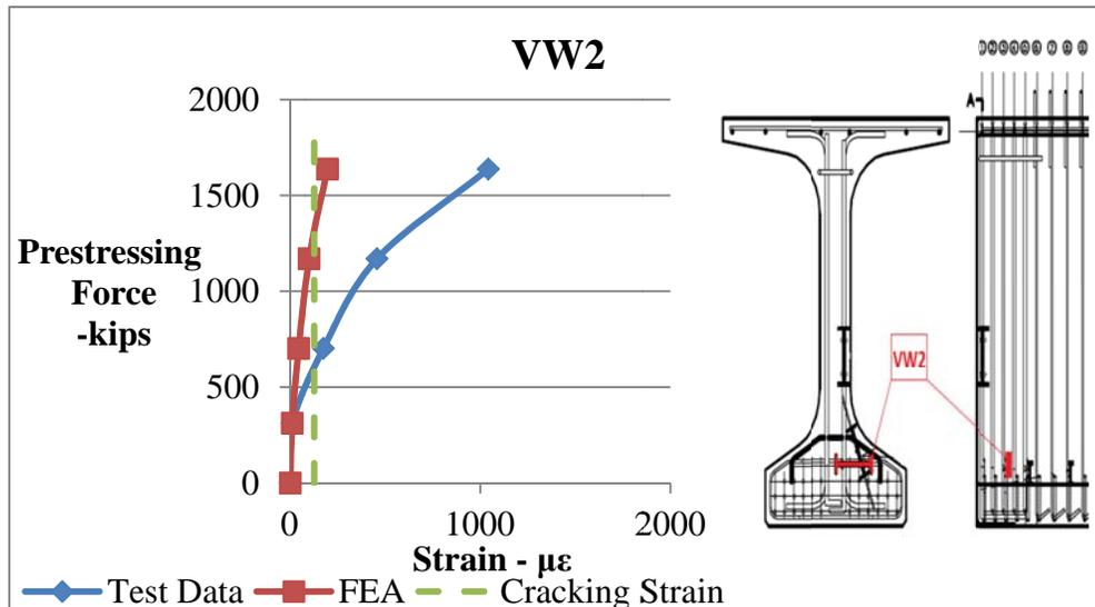
Figure 6-33. Concrete strains comparisons between data obtained by VW gauge 2 and finite element model during prestress release for bonded girder. (positive = tension)
