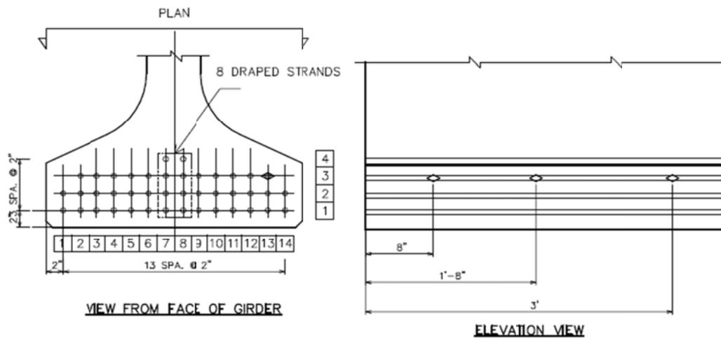
Figure 6-9. The location of Strain Gauges at Strand. Elevation view (right), and cross section view (left).
