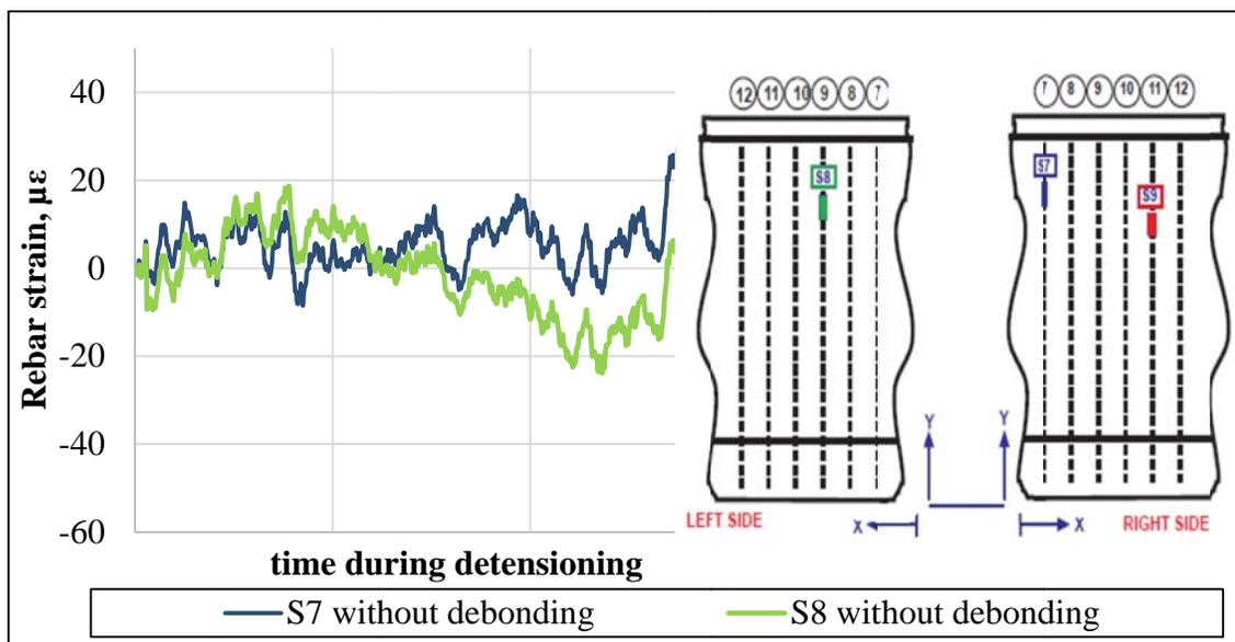
Figure 5-17. Bonded girder: Strain change of reinforcing bars in inclined crack region, close to top of girder (gauges S7, and S8). (*Tension positive, compression negative*)
