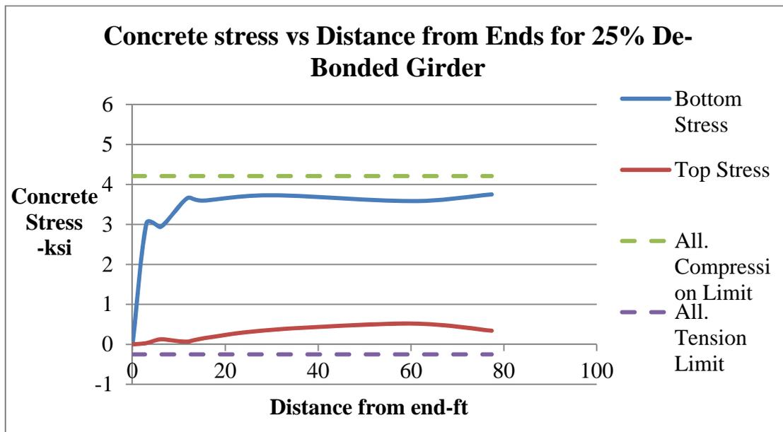
Figure 5-4. Concrete stress vs Distance from Ends for De-bonded Girder.
