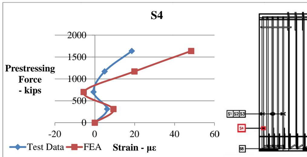
Figure 6-38. Re-bar strain comparisons between data obtained from strain gauge 4 and finite element model during prestress release for bonded girder. (*positive = tension*)
