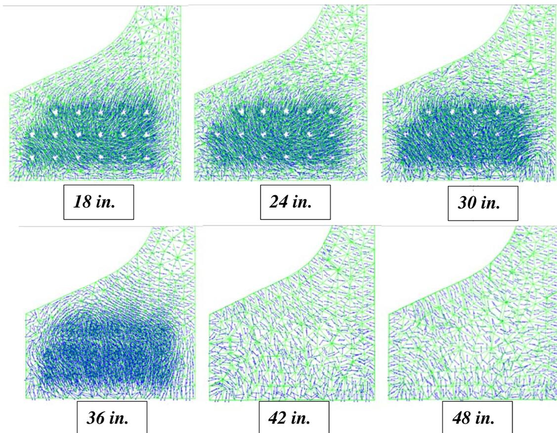
Figure 7-3. Principal tensile strains directions on the cross section of bottom flange at various distances in from the girder end.
