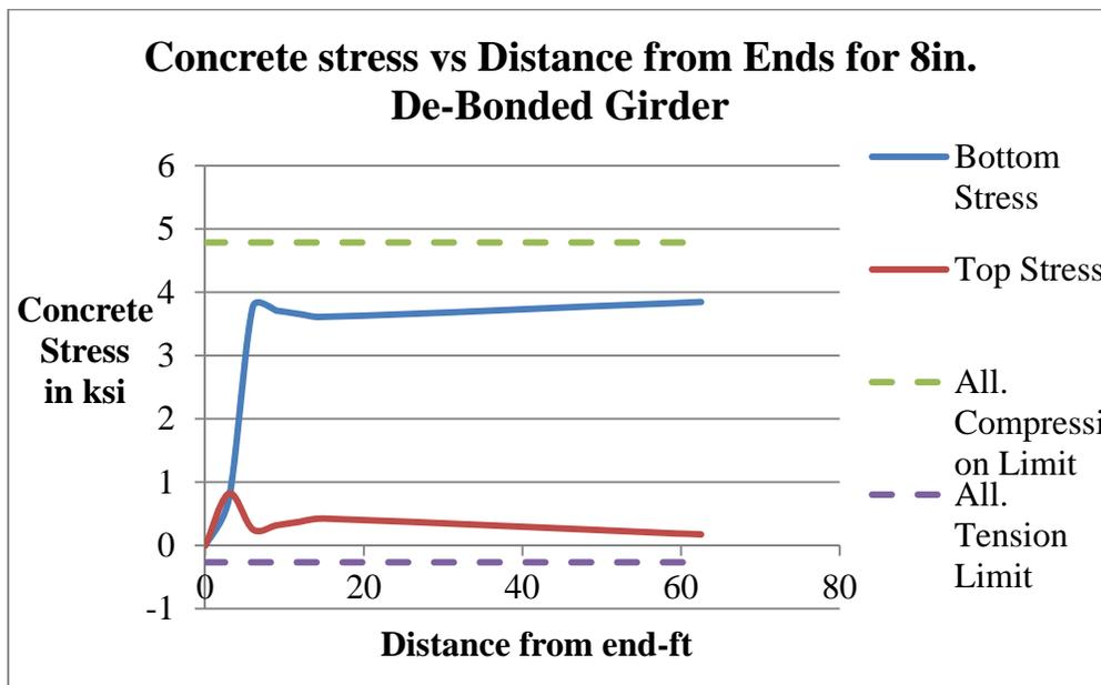
Figure 6-5. Bottom and top concrete stresses in 8in. de-bonded girder.
