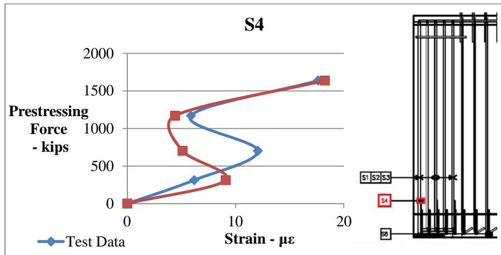
Figure 6-45. Re-bar strain comparisons between data obtained from strain gauge 4 and finite element model during prestress release for 38% de-bonded girder. (*positive = tension*)
