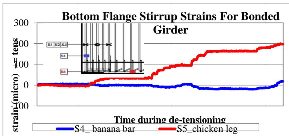
Figure 6-18. The test strain results for S4 (on banana bar) and S5 (on chicken leg bar) stirrups for bonded girder. (positive is tension)
