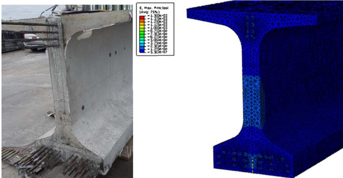
Figure 6-40. The comparison of 38% de-bonded girder ends in reality and in model.
