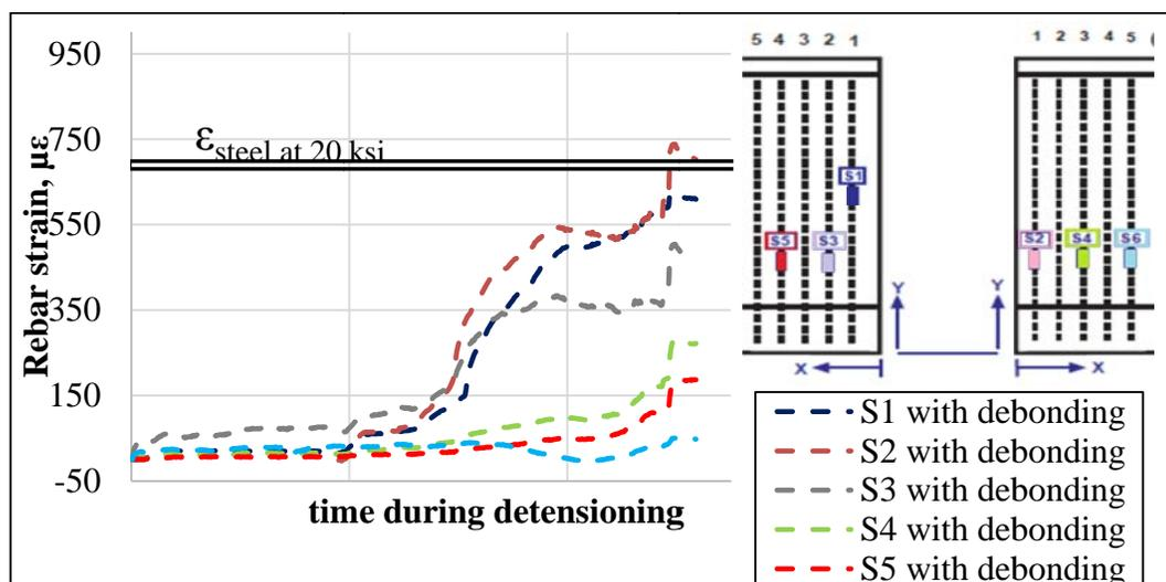
Figure 5-16. Debonded girder: Strain change of reinforcing bars in horizontal web crack region, most are 20" up from bottom (gauges S2, S3, S4, S5 and S6).
