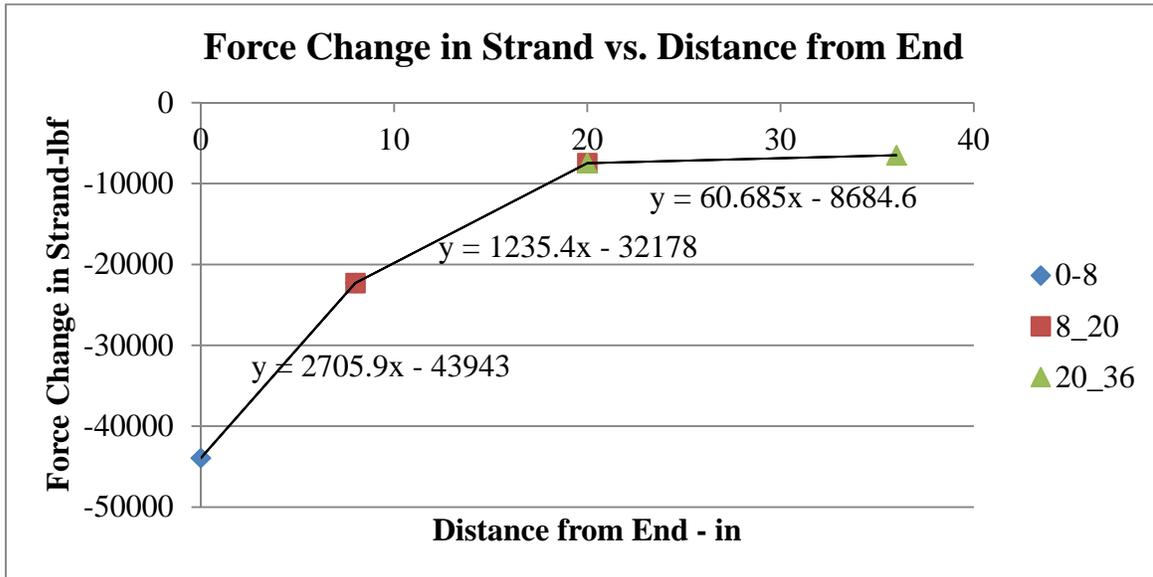
Figure 4-9. Prestressing force change in strand versus distance from end considering piecewise linear function for 72W girders.
