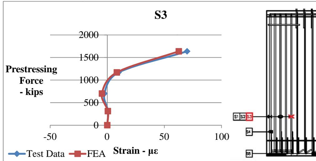
Figure 6-37. Re-bar strain comparisons between data obtained from strain gauge 3 and finite element model during prestress release for bonded girder. (*positive = tension*)
