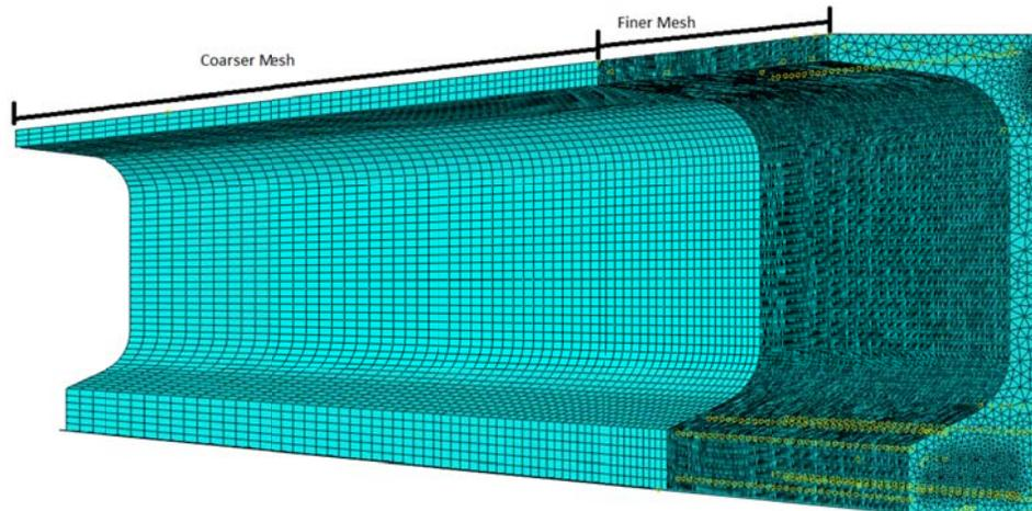
Figure 4-13. Mesh example of 54W girder.
