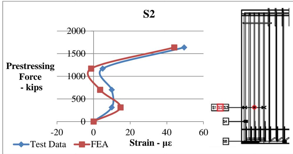
Figure 6-44. Re-bar strain comparisons between data obtained from strain gauge 2 and finite element model during prestress release for 38% de-bonded girder. (*positive = tension*)
