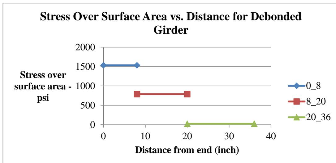
Figure 5-14. Bond Stress vs distance from ends of debonded girders.
