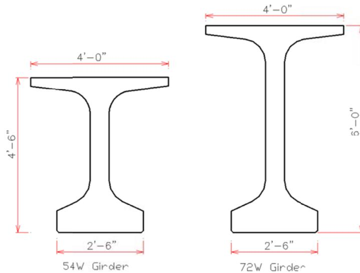
Figure 3-1. Girder sizes: 54W and 72W.
