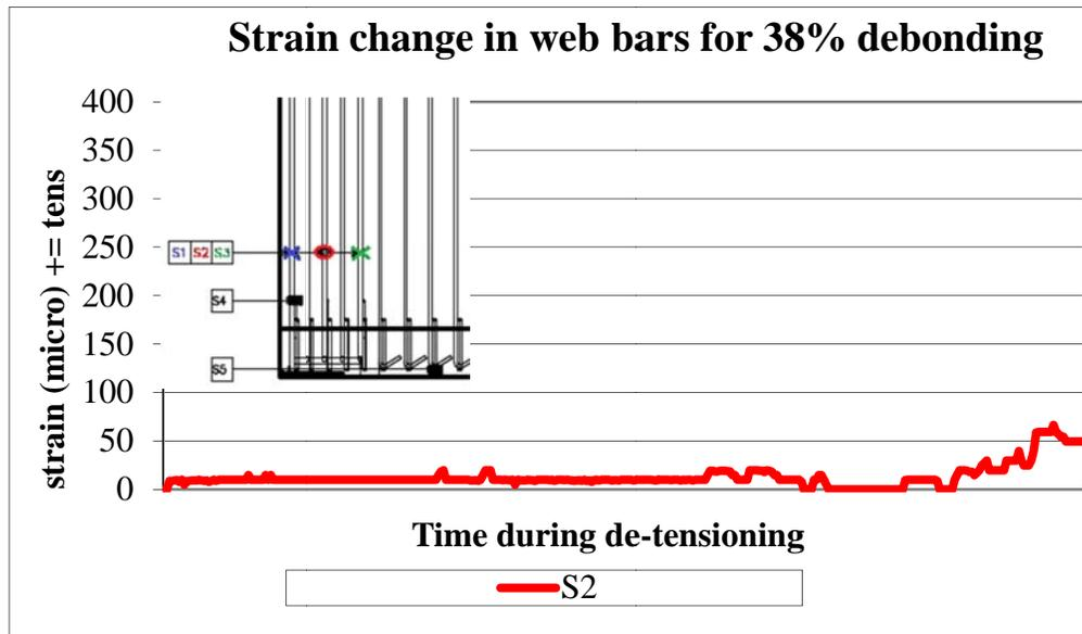
Figure 6-16. The test results of web bar strain gauge S2 for 38% debonded girder. (positive is tension)
