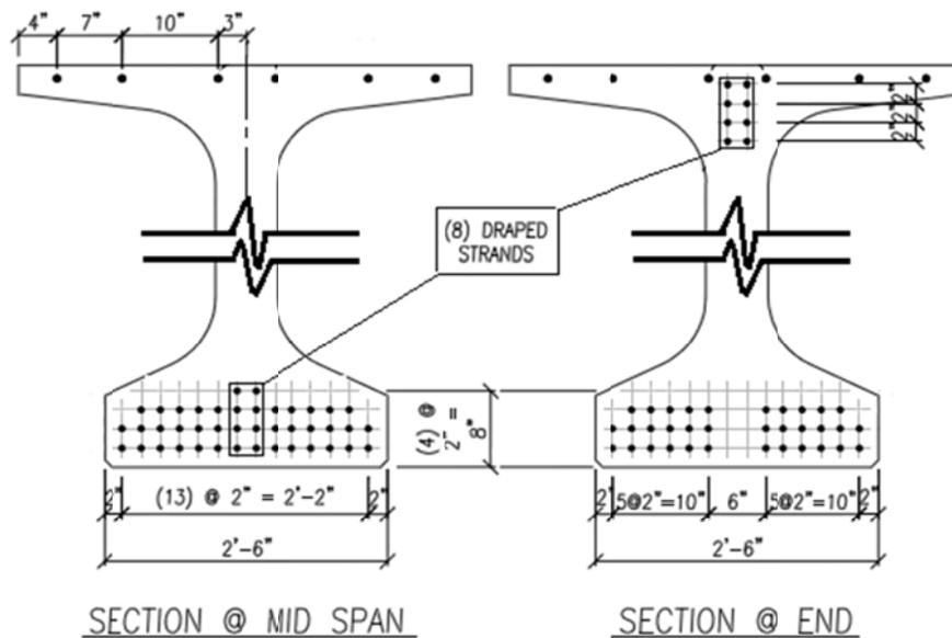
Figure 6-2. Original strand pattern at the ends of girders.
