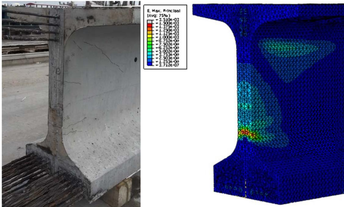
Figure 6-47. The comparison of 62% de-bonded girder ends in reality and in model.
