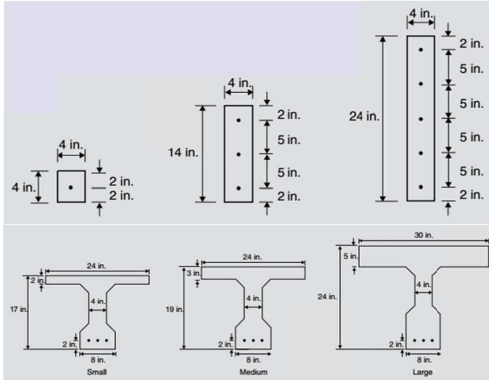
Figure 2-7. Beam (top) and T beam (bottom) cross sections (7).
