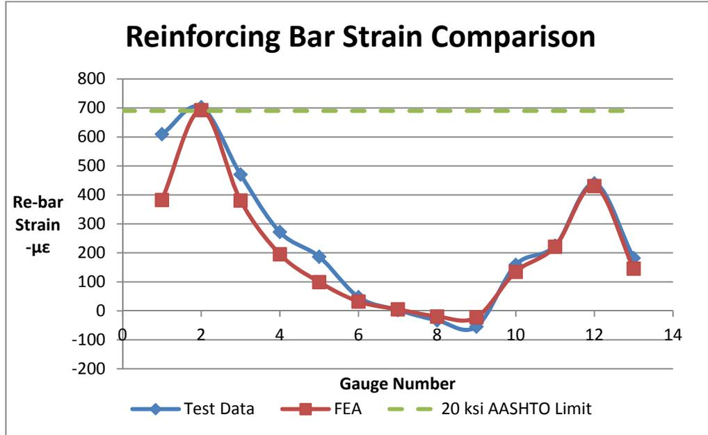
Figure 5-34. Reinforcing bar strain comparison for de-bonded girder.
