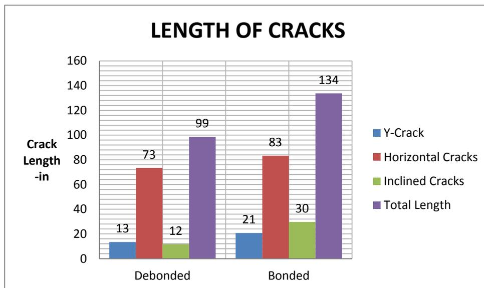
Figure 5-28. Total length of cracks at girder ends.
