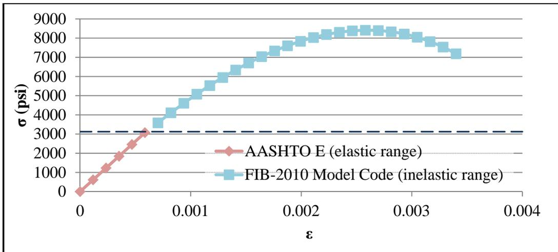
Figure 4-3. Compression constitutive graph with the model of a bonded 72W girder
