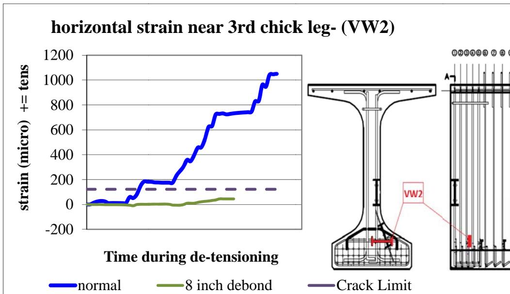
Figure 6-22. Strain Results for Vibrating wire gauge VW2. (positive = tension)
