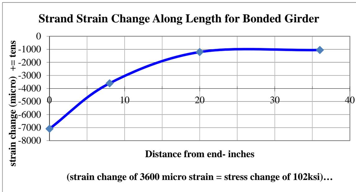
Figure 5-11. Strand test data for bonded girders.
