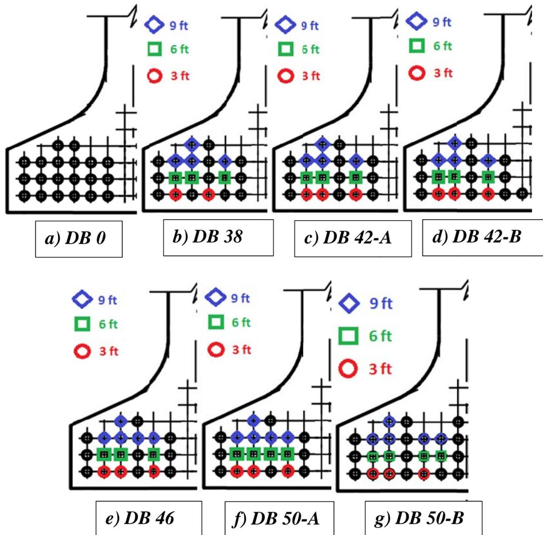
Figure 8-1. Strand patterns at the ends of girders. Distances denoted are locations where those strands start bonding.
