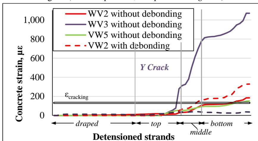
Figure 5-22. Strain change of vibrating wire gauges near the Y cracking region. (*Tension positive, compression negative, V5 is vertical*)
