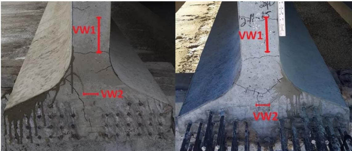
Figure 5-23. Location of vibrating wire gauges VW1 and VW2 in both bonded (left) and de-bonded (right) girders.
