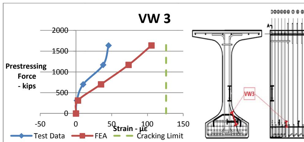
Figure 6-49. Concrete strains comparisons between data obtained via VW gauge 3 and finite element model during prestress release for 62% de-bonded girder. (*positive = tension*)
