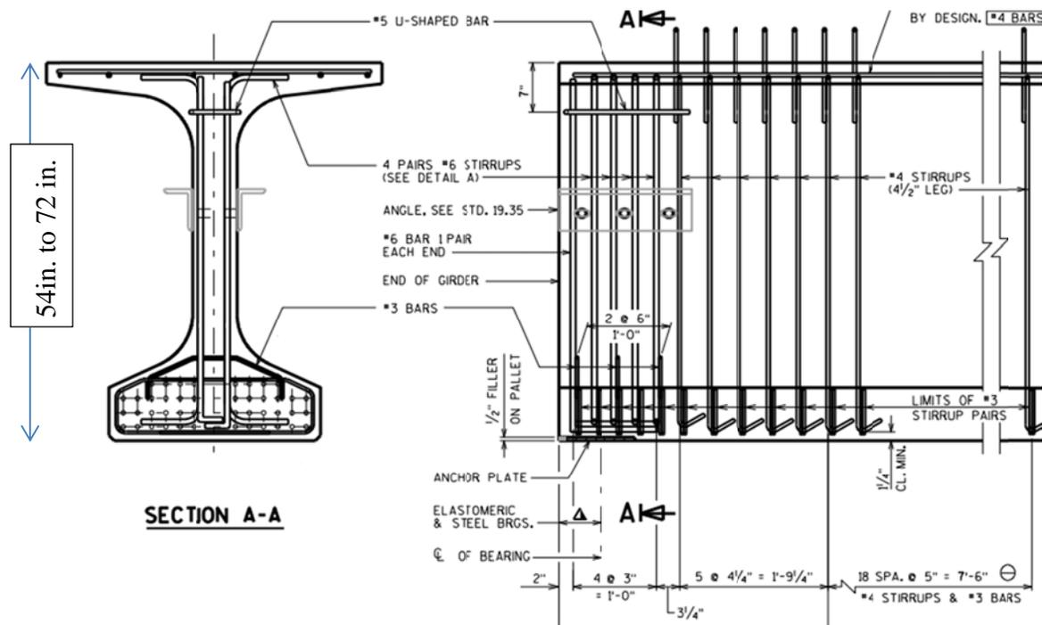
Figure 3-2. The end details of girders.
