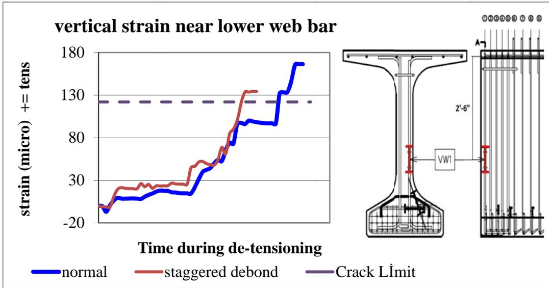
Figure 6-21. Strain results for vibrating wire gauge VW1. (positive = tension)
