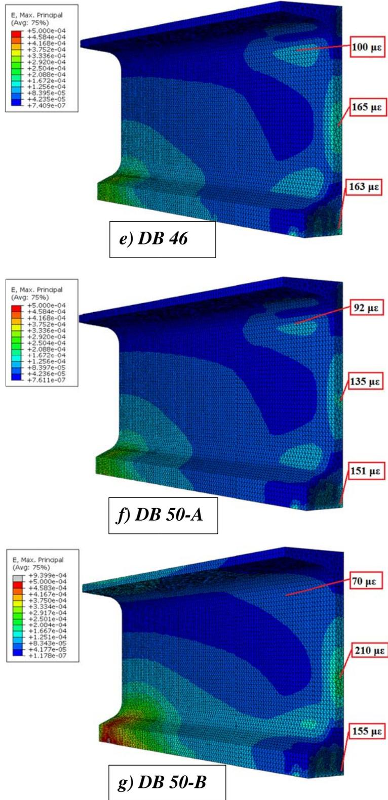
Figure 8-2. Contour plots of bonded and debonded 72W girders with 48 strands.
