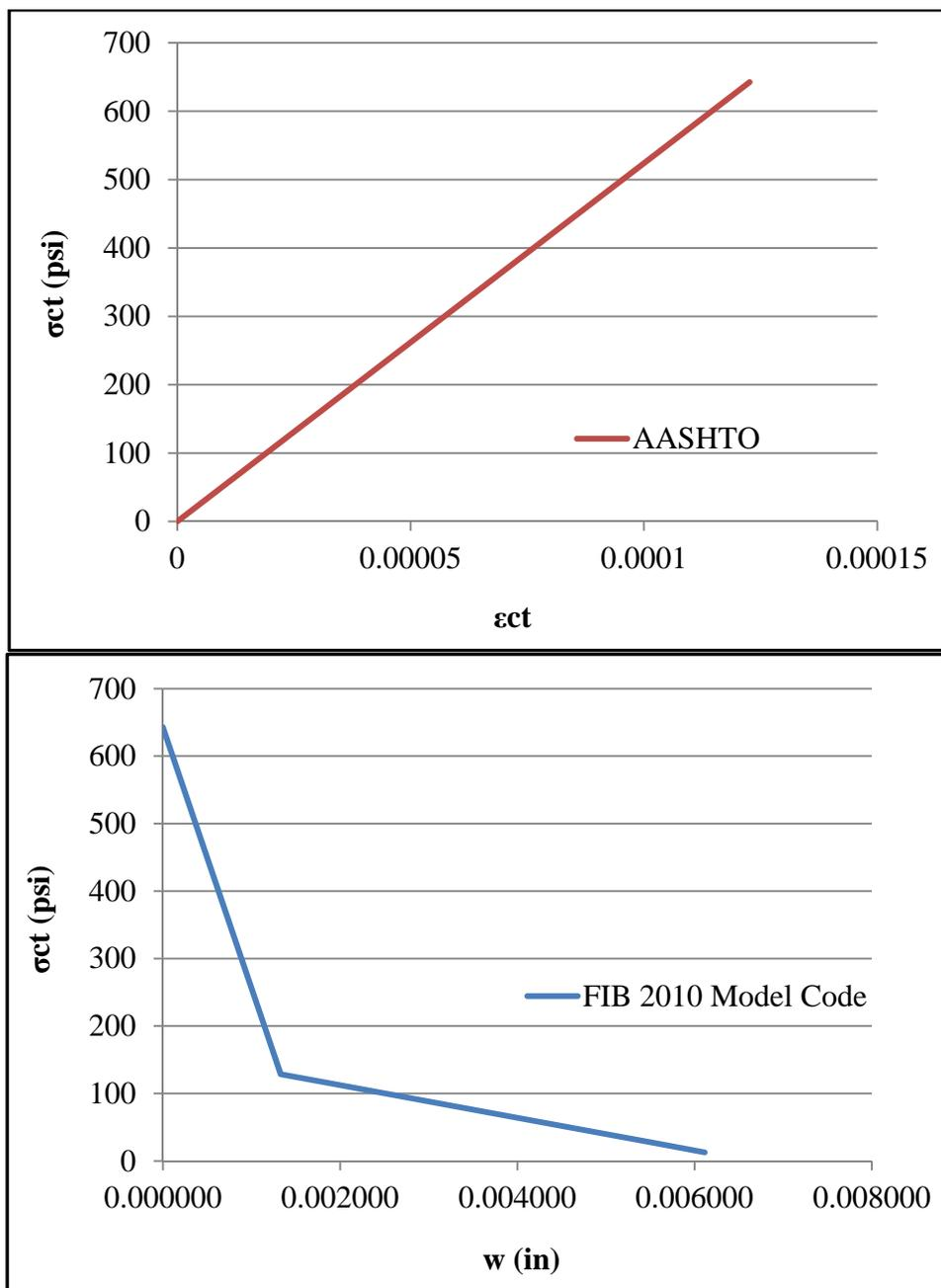
Figure 4-5. Tension Model Used in Abaqus: top = before cracking, bottom = post cracking.
