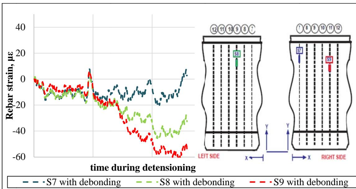
Figure 5-18. Debanded girder: Strain change of reinforcing bars in inclined crack region, close to top of girder (gauges S7, S8, and S9). (*Tension positive, compression negative*)
