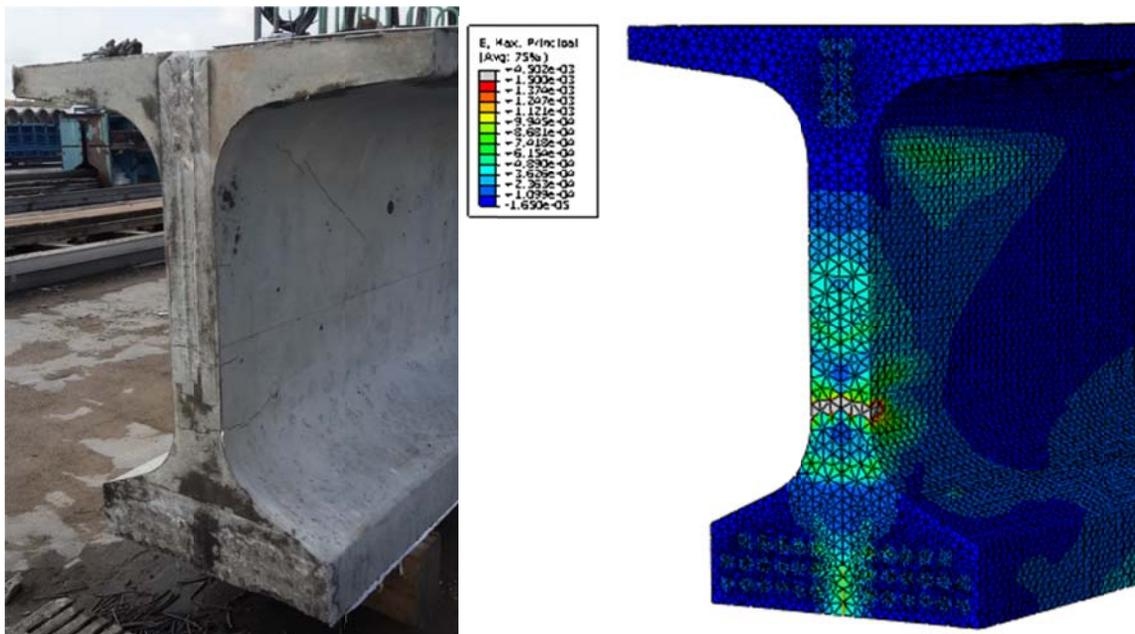
Figure 6-31. The comparison of bonded girder ends in reality and in model.
