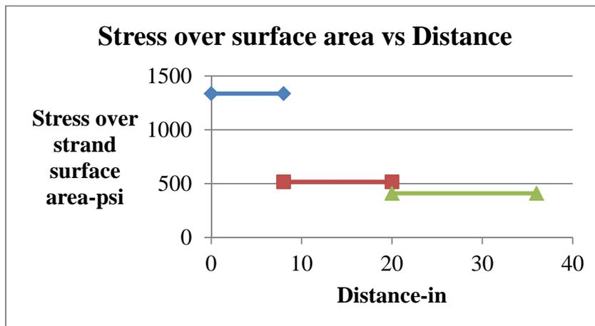
Figure 6-14. Bond Stress Variation Used in the Analytical Models.
