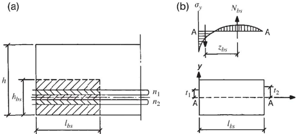
Figure 2-2. The prism analogy for calculation of the bursting force (4).
