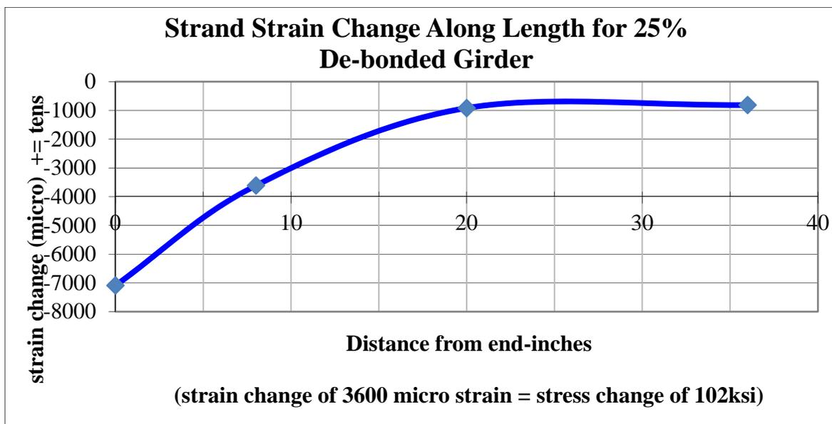
Figure 5-12. Strand test data for de-bonded girders.
