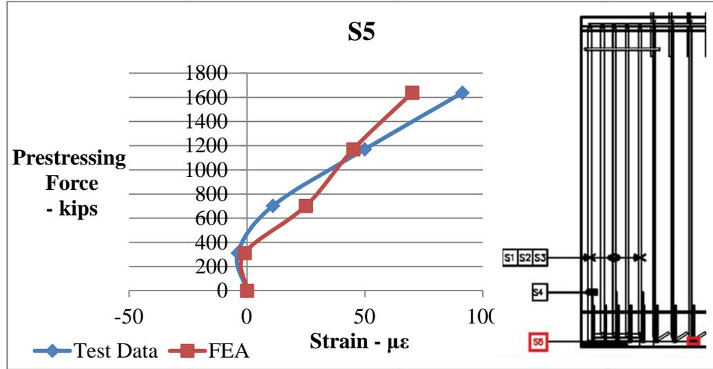
Figure 6-46. Re-bar strain comparisons between data obtained from strain gauge 5 and finite element model during prestress release for 38% de-bonded girder. (*positive = tension*)
