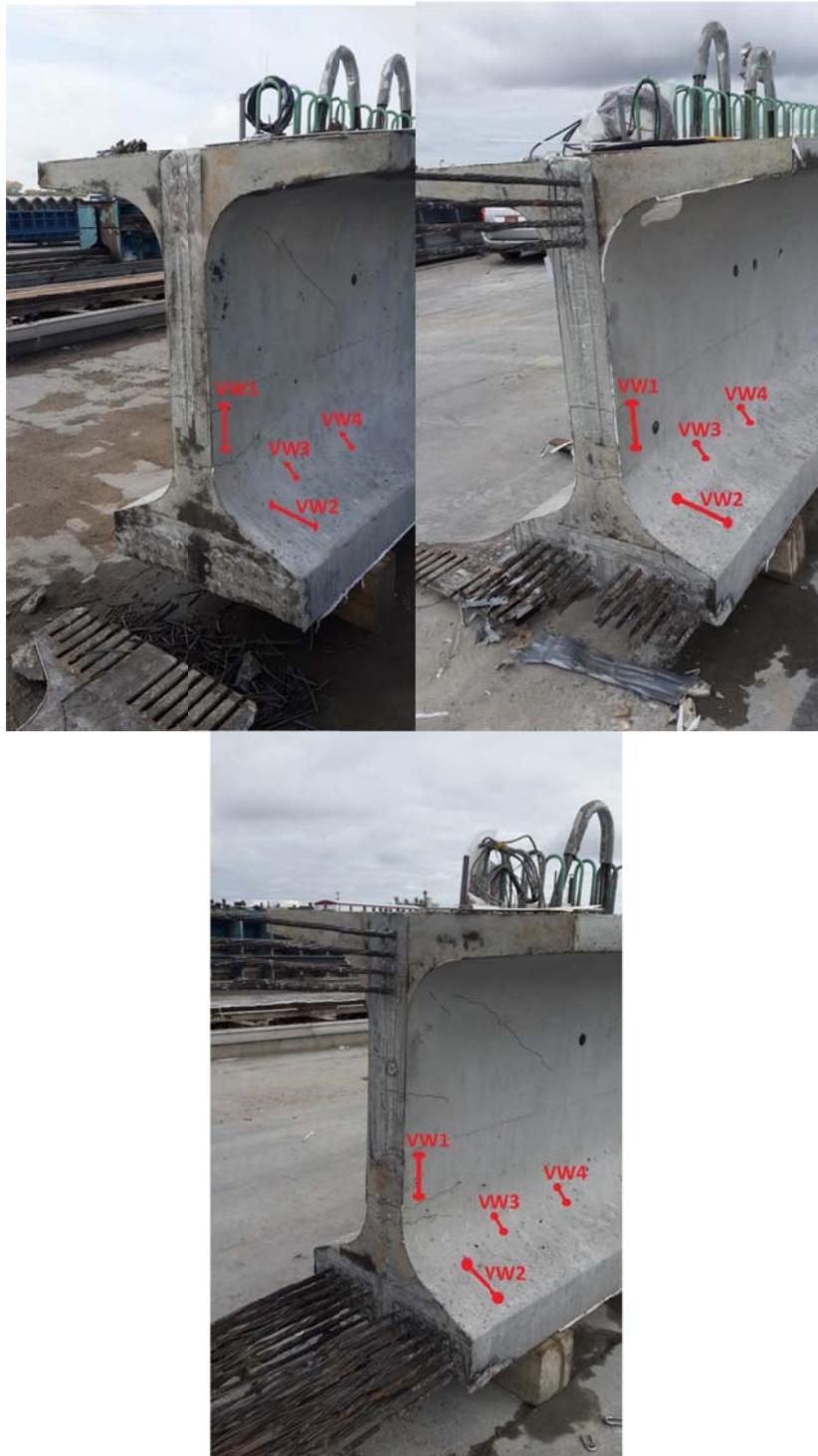
Figure 6-25. The location of vibrating wire gauges in bonded (top left), 38% debonded (top right), and the girder that is debonded 8 in. from end (bottom).
