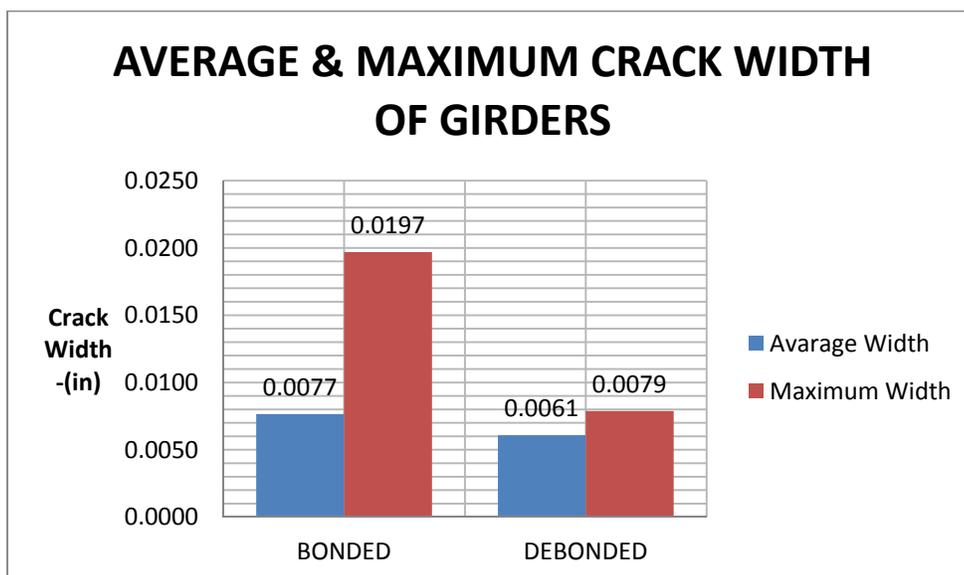
Figure 5-27. Average & maximum crack widths.
