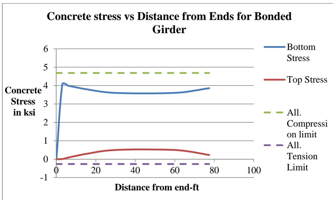
Figure 5-3. Concrete stress vs Distance from Ends for Bonded Girder.
