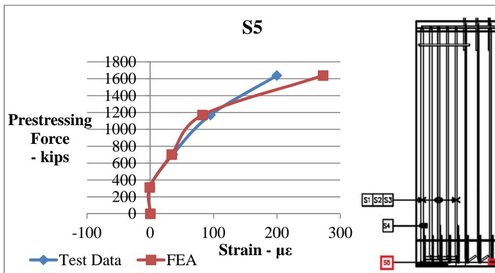
Figure 6-39. Re-bar strain comparisons between data obtained from strain gauge 5 and finite element model during prestress release for bonded girder. (*positive = tension*)
