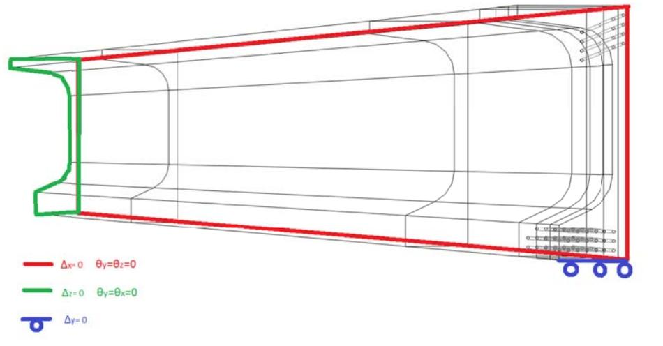
Figure 4-7. Boundary Conditions of models, mid-span section is at left, end at right.
