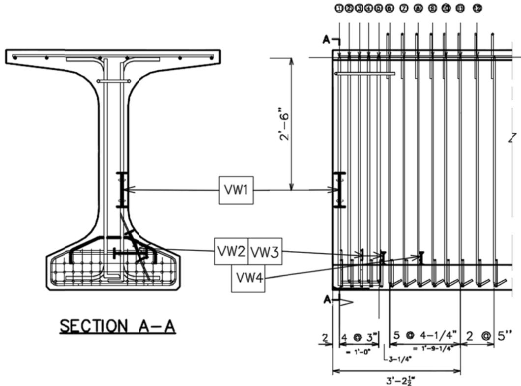
Figure 6-12. Location of Vibrating Wire Gauges.
