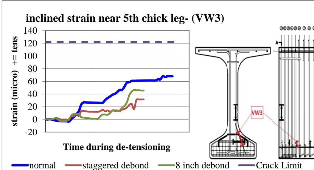
Figure 6-23. Strain Results for Vibrating wire gauge VW3. (*positive = tension*)
