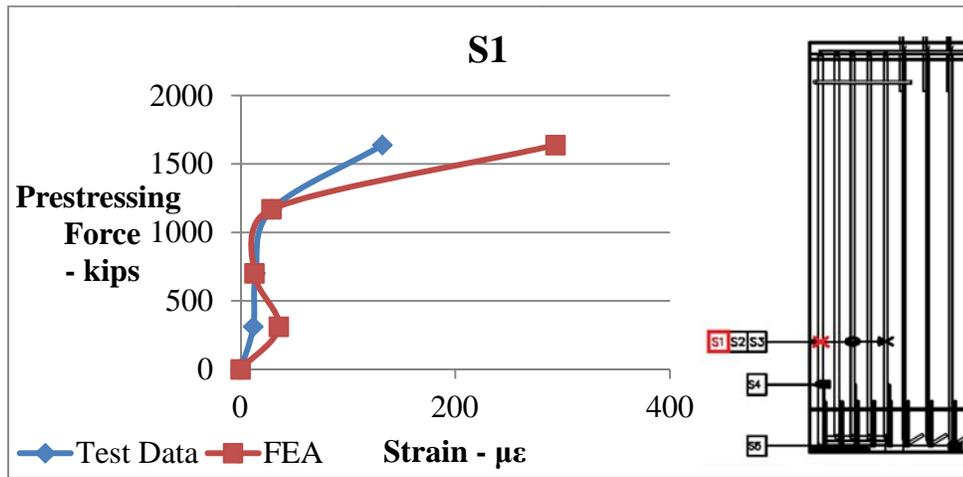
Figure 6-35. Re-bar strain comparisons between data obtained from strain gauge 1 and finite element model during prestress release for bonded girder. (positive = tension)
