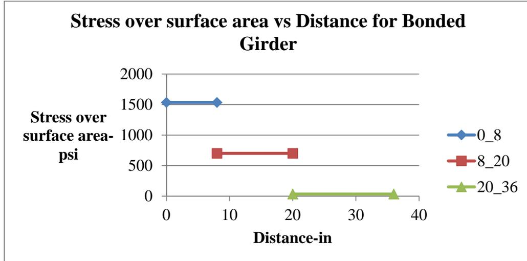
Figure 5-13. Bond Stress vs distance from ends of bonded girders.
