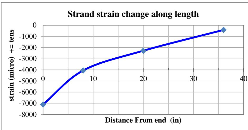
Figure 6-13. The Change in strain at locations along strand of 38% debonded beam.
