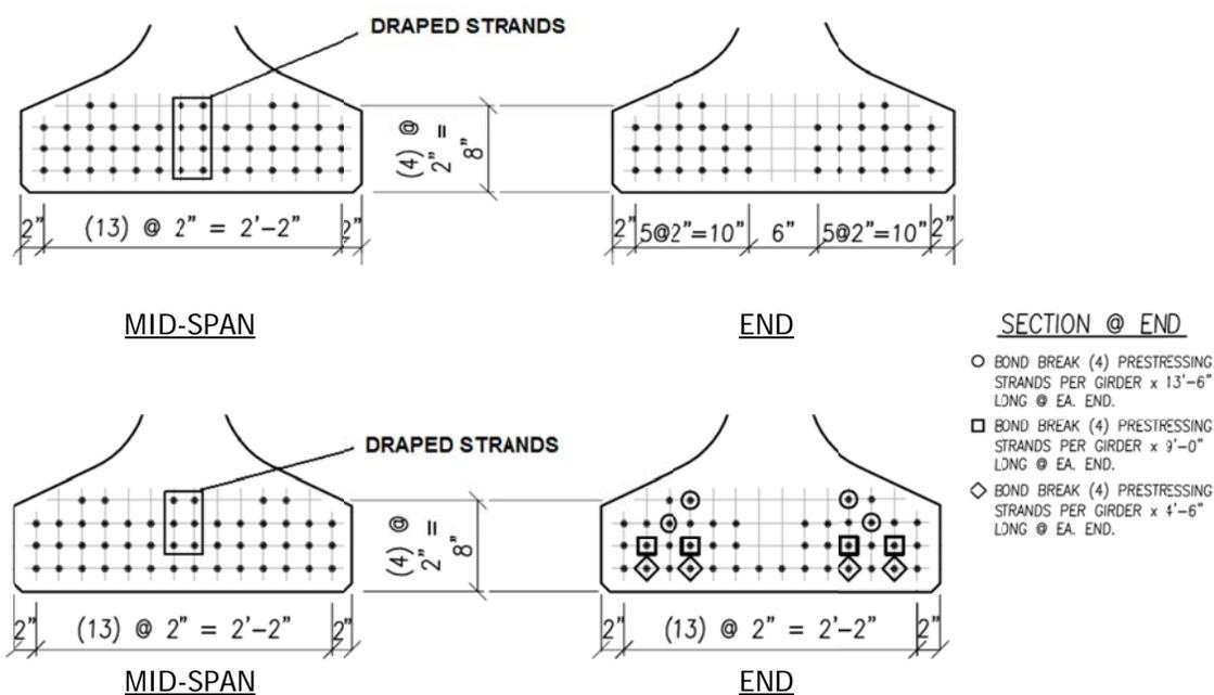
Figure 5-2. Bonded girder strand pattern (top) and de-bonded girder strand pattern (bottom).
