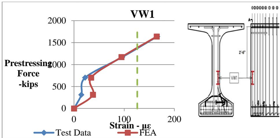
Figure 6-32. Concrete strain comparison between data obtained by VW gauge 1 and finite element model during prestress release for bonded girder. (positive = tension)
