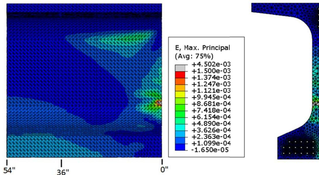
Figure 7-1. Principal tensile strains in concrete, elevation view (left) and cross section view at the end (right). (*positive = tensile*)
