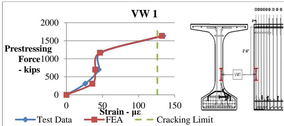
Figure 6-41. Concrete strain comparison between data obtained by VW gauge 1 and finite element model during prestress release for 38% de-bonded girder. (positive = tension)
