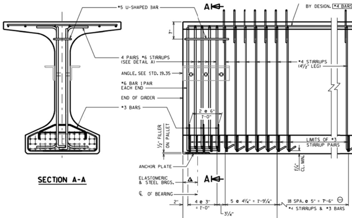
Figure 6-1. End details of 54W girder.
