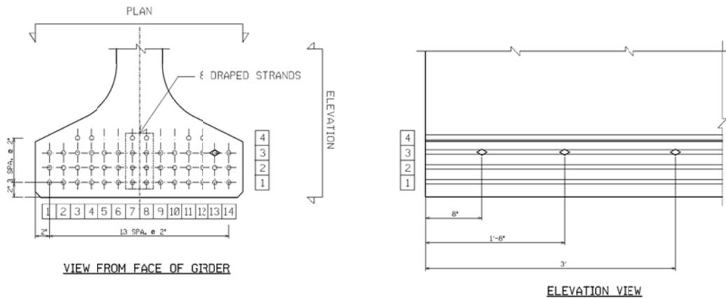
Figure 5-9. Location of strain gauges at strand.
