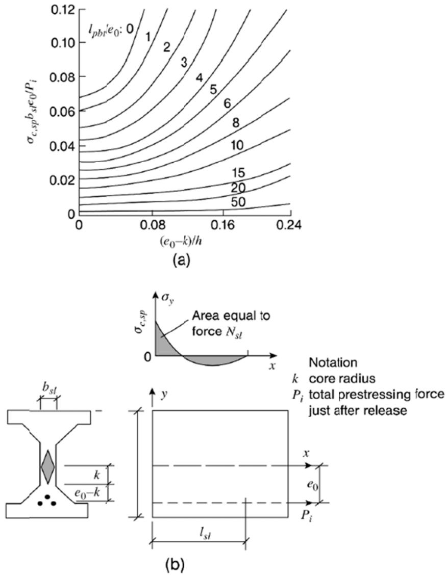
Figure 2-3. Maximum spalling stresses (4).
