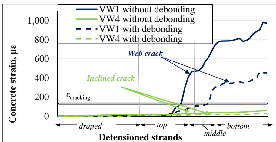
Figure 5-21. Strain change of vibrating wire gauges near the web and inclined cracking region. (*Tension positive, compression negative*)
