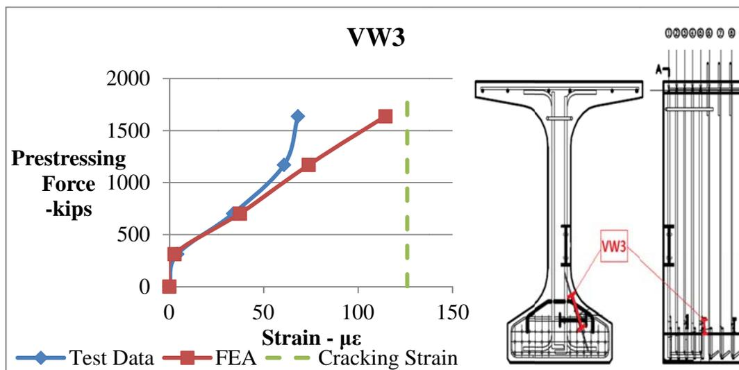
Figure 6-34. Concrete strains comparisons between data obtained by VW gauge 3 and finite element model during prestress release for bonded girder. (*positive = tension*)
