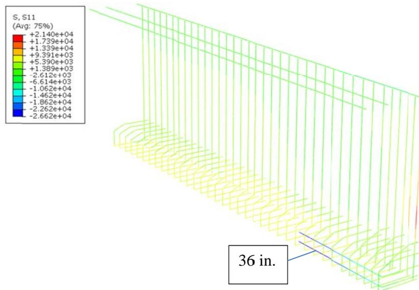
Figure 7-4. Longitudinal stresses – S11 (psi) of reinforcing bars in 72W girder.
