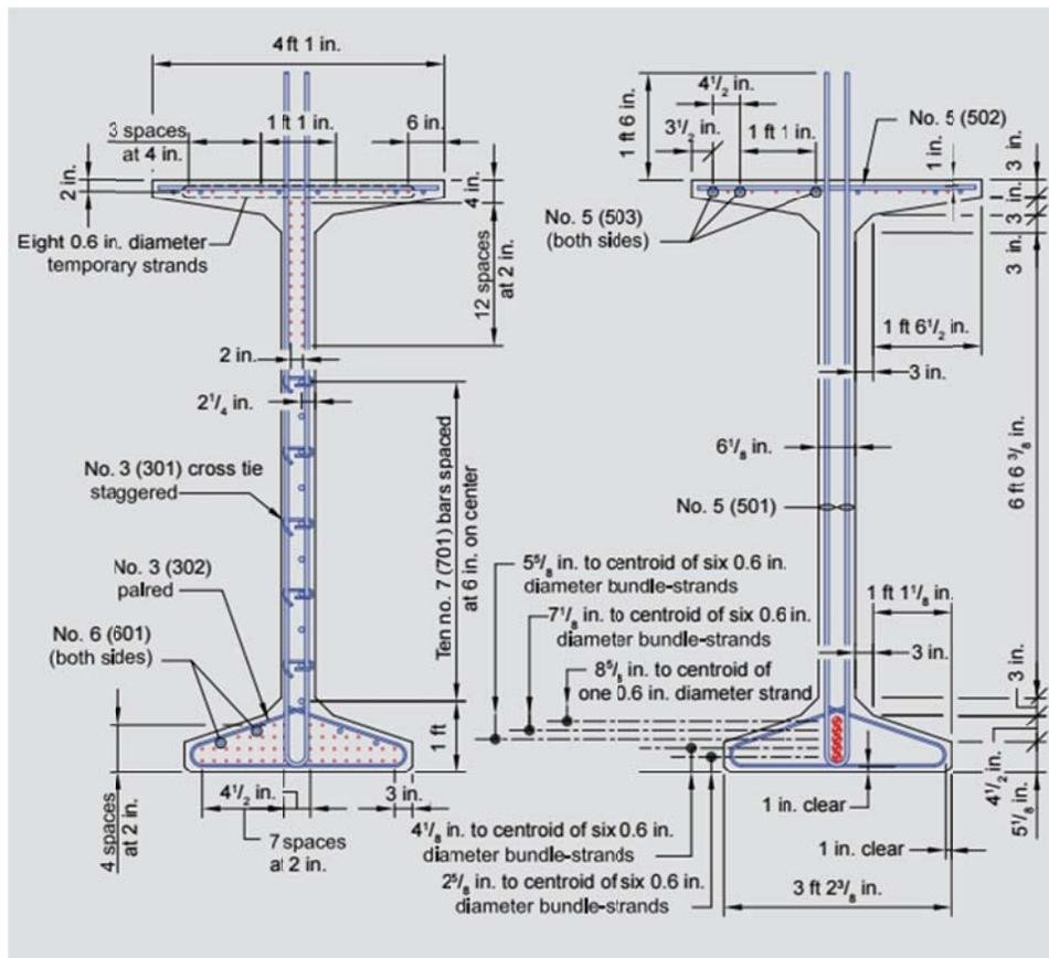
Figure 2-9. Typical cross sections of WF100G girder (9).
