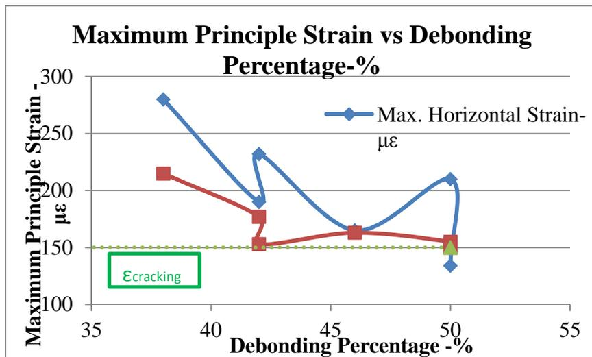
Figure 8-3. Maximum principal strain at horizontal and Y crack region from each girder. (Note: A fully bonded strand pattern resulted in maximum horizontal and Y-crack strains of 1243 and 2734  $\mu\epsilon$  respectively.)
