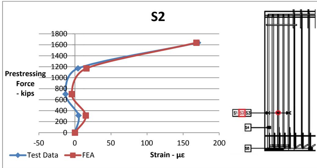
Figure 6-52. Re-bar strain comparisons between data obtained from strain gauge 2 and finite element model during prestress release for 62% de-bonded girder. (positive = tension)
