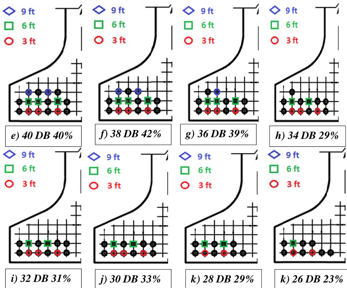
Figure 8-4. Recommended debonding patterns for 72W and 54W girders with different number of strands.
