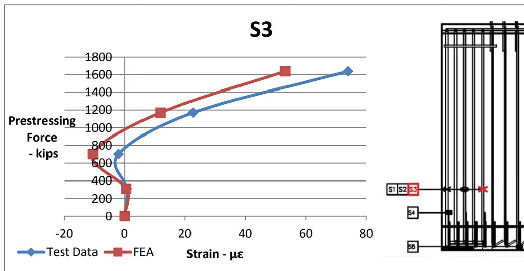
Figure 6-53. Re-bar strain comparisons between data obtained from strain gauge 3 and finite element model during prestress release for 62% de-bonded girder. (positive = tension)
