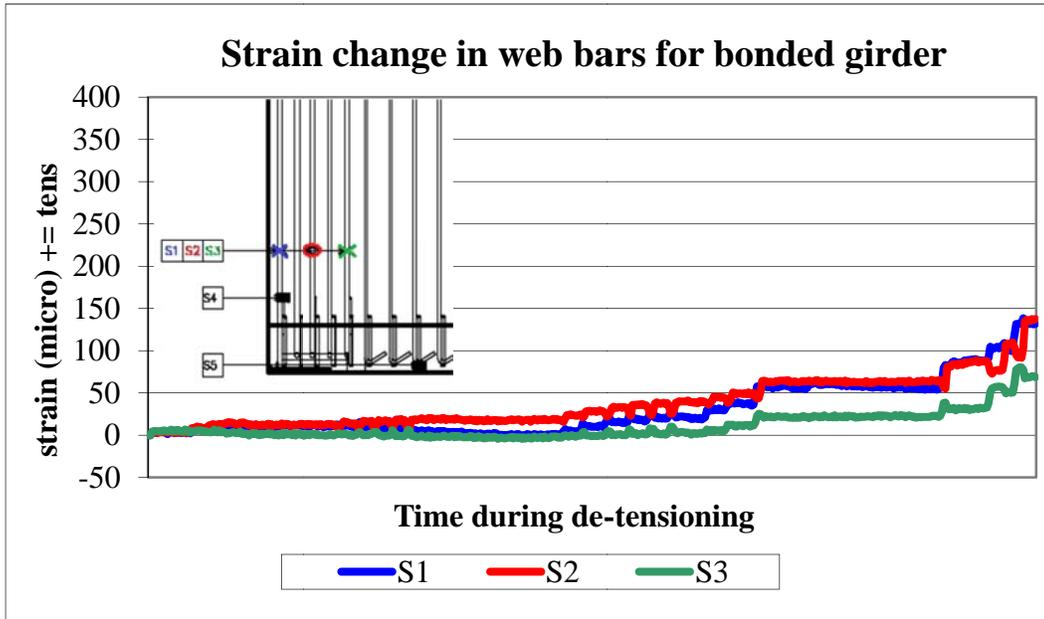
Figure 6-15. The test results of web bar strain gauges S1, S2, and S3 for bonded girder (positive is tension).
