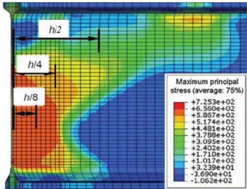
Figure 2-11. Principal stress distribution in concrete along anchorage zone (9).
