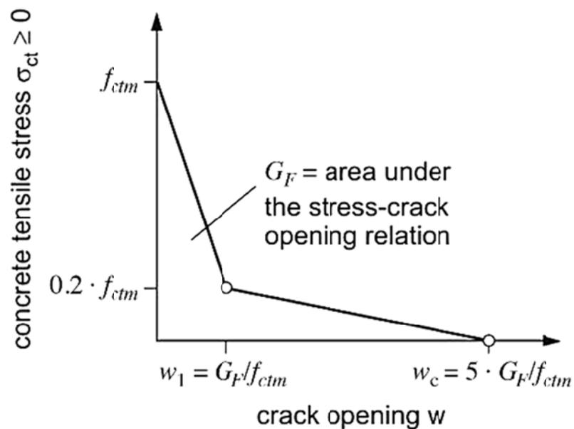
Figure 4-4. Post- Cracking Behavior Graph
