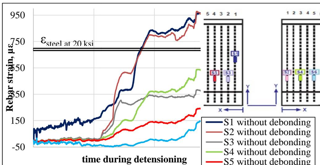
Figure 5-15. Bonded girder: Strain change of reinforcing bars in horizontal web crack region, most are 20" up from bottom (gauges, S2, S3, S4, S5 and S6).
