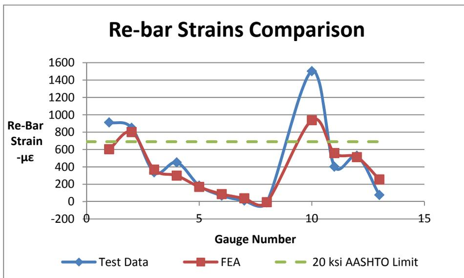
Figure 5-31. Reinforcing bar strain comparison for bonded girder.
