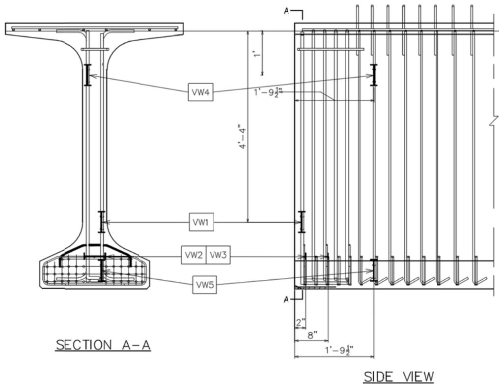
Figure 5-10. Vibrating Wire Gauge Locations.
