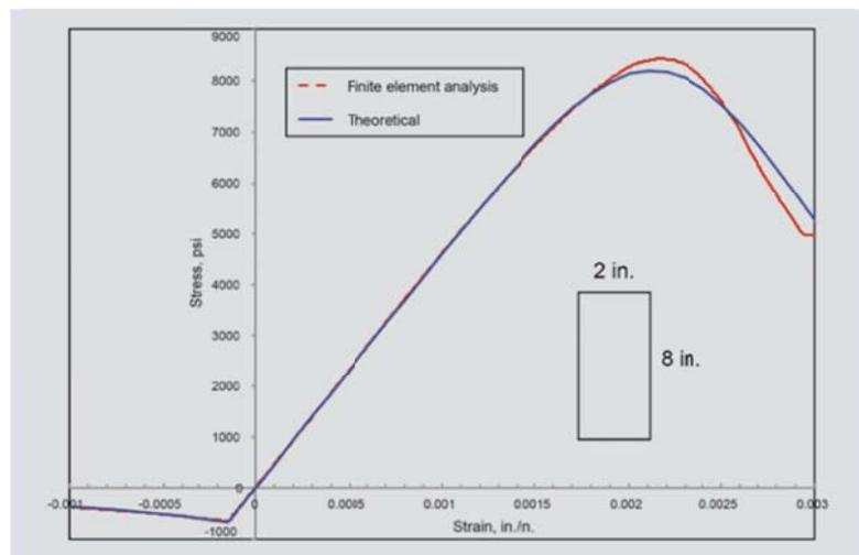
Figure 2-10. Constitutive model and theoretical stress-strain curve (9).
