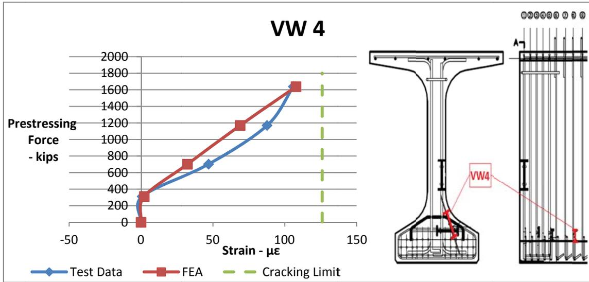
Figure 6-50. Concrete strains comparisons between data obtained via VW gauge 4 and finite element model during prestress release for 62% de-bonded girder. (positive = tension)
