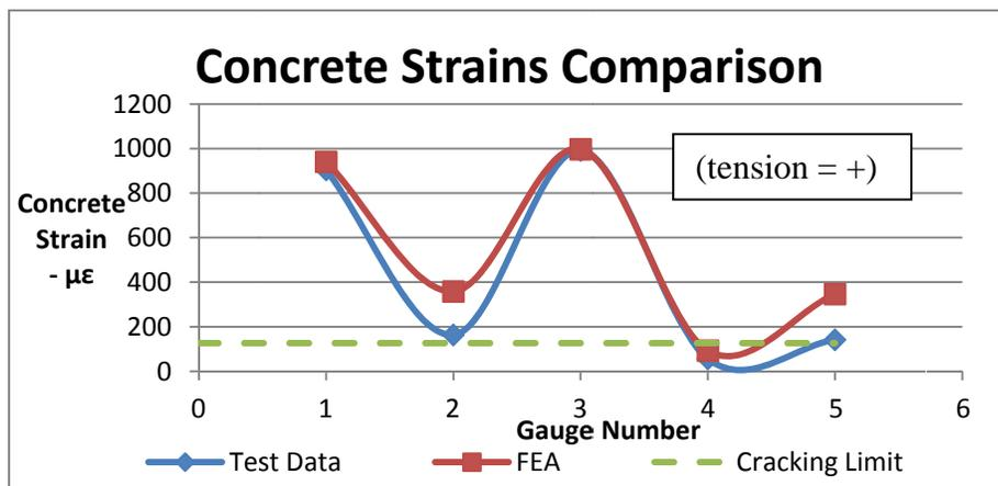
Figure 5-30. Concrete strain comparison for bonded girder.
