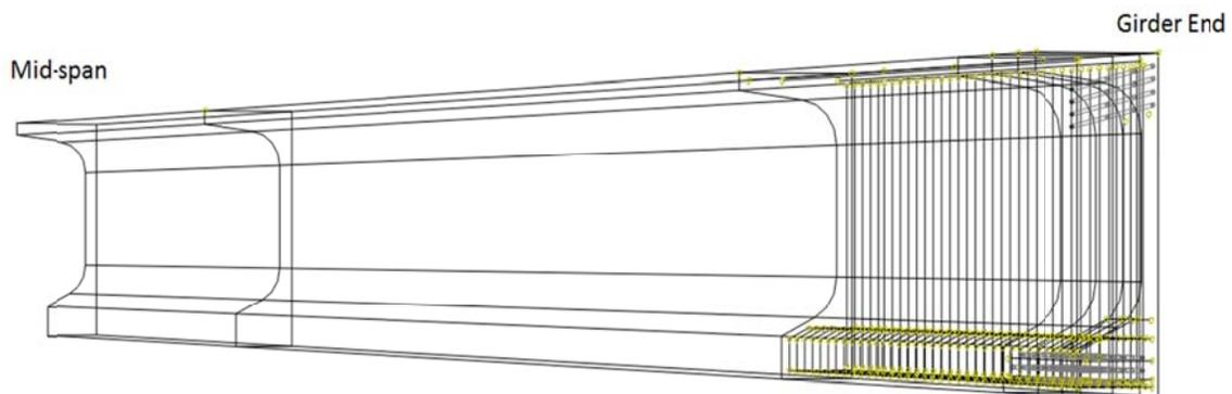
Figure 4-1. Model of Bonded 54W girder in Abaqus.
