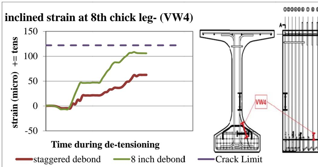
Figure 6-24. Strain Results for Vibrating wire gauge VW4. (*positive = tension*)
