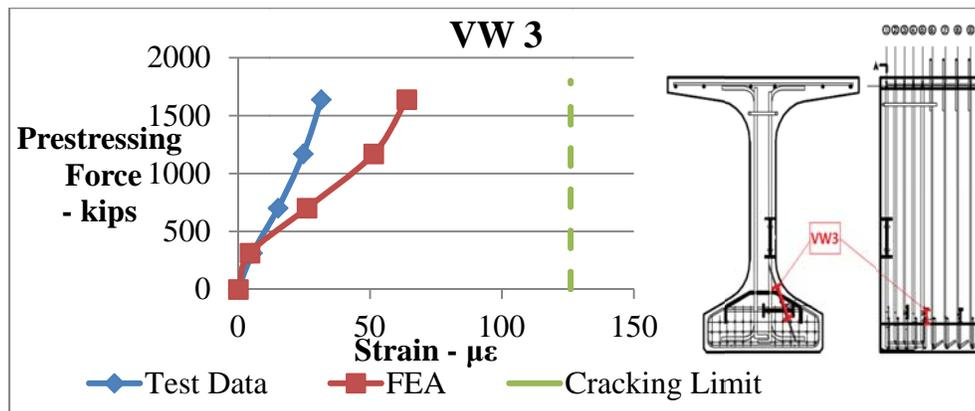
Figure 6-42. Concrete strain comparison between data obtained by VW gauge 3 and finite element model during prestress release for 38% de-bonded girder. (positive = tension)
