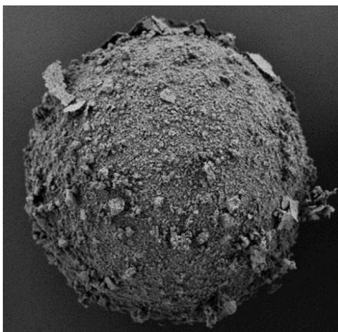
An SEM image of a bubble shell's outer surface
