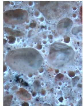
Air voids measuring 10  $\mu\text{m}$  – 1 mm in diameter
