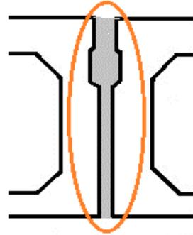
(b) Full-depth grouted partial depth shear key
