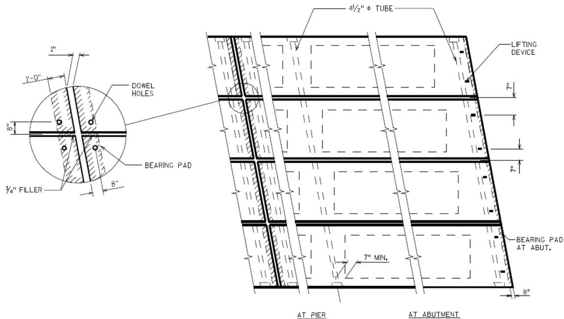
Figure 3-5. The bearing layout given with the most recent standard details
