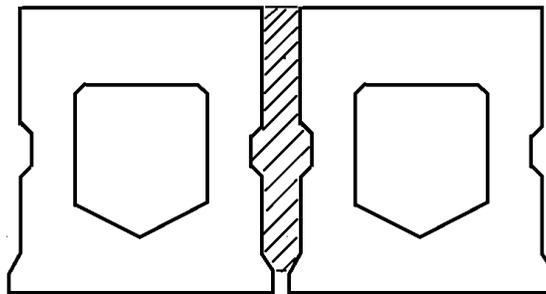
(e) Cast-in-place concrete shear key used in Korea
