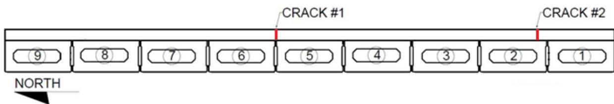
Figure 5-4. Crack locations on west abutment (facing east)
