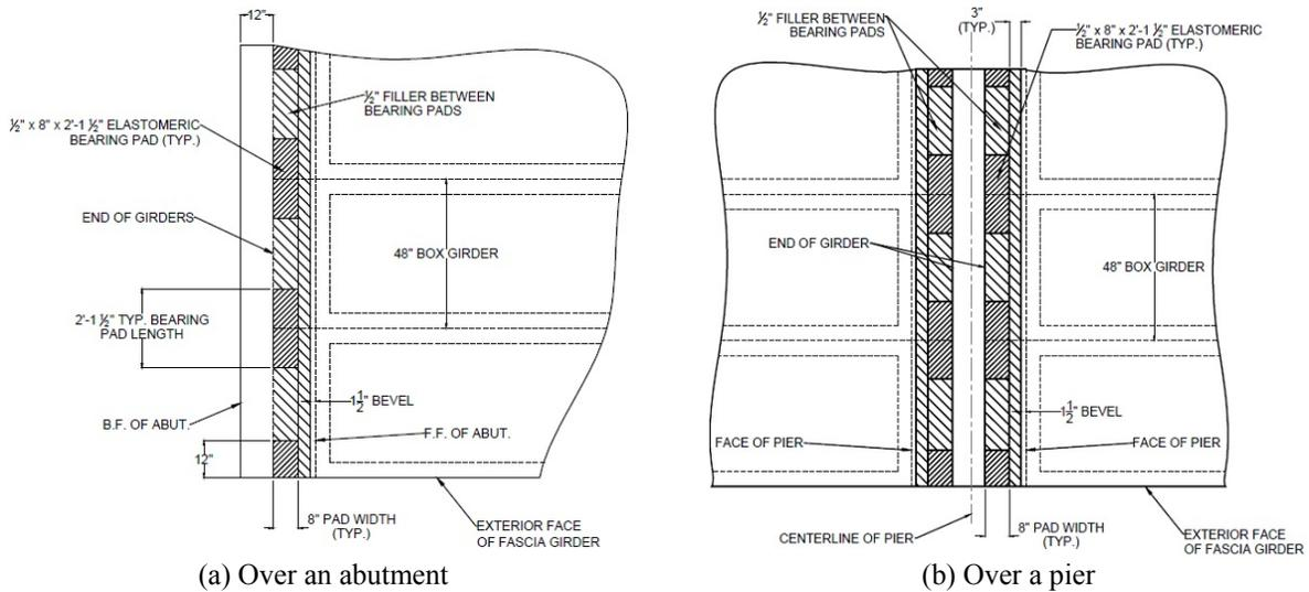
Figure 3-4. Bearing pad plan
