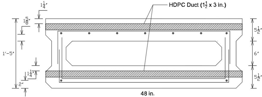
b) Proposed changes to beam details with ducts
