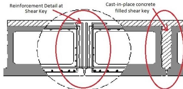
(f) Cast-in-place reinforced concrete shear key used in the UK.
