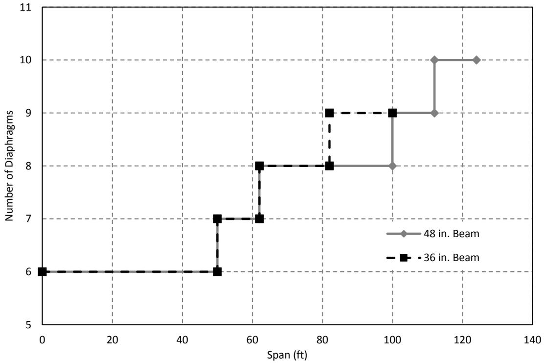
Figure 2-4. Recommended number of diaphragms (source: Grace et al. 2012)
