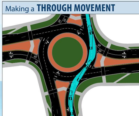
► **Case 1** designs have a single white pavement marking line separating the entry lanes. Large trucks are expected to encroach into adjacent lanes as they approach, enter, circulate, and exit the roundabout.
