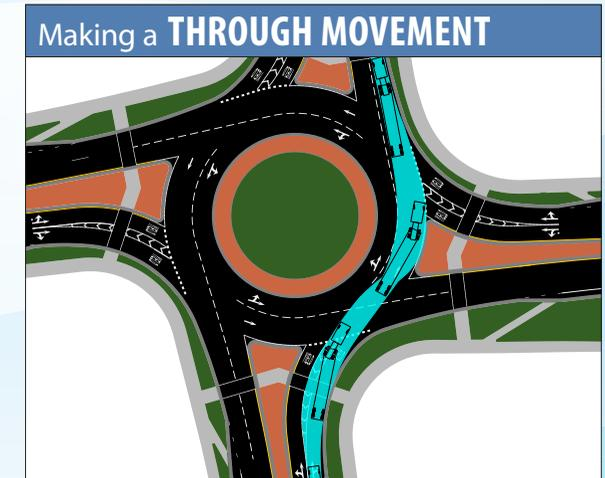
► **Case 2** designs have painted gores that provide separation between the entry lanes. Large trucks can stay in-lane as they approach and enter the roundabout, but may need to encroach into adjacent lanes as they circulate and exit the roundabout.
