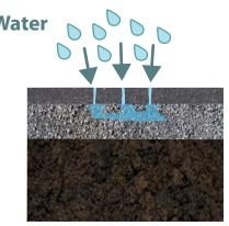
As vehicles repeatedly drive over the uneven sub-base, the pavement experiences atypical stresses and develops additional cracks. Eventually the pavement breaks apart and a pothole forms.
