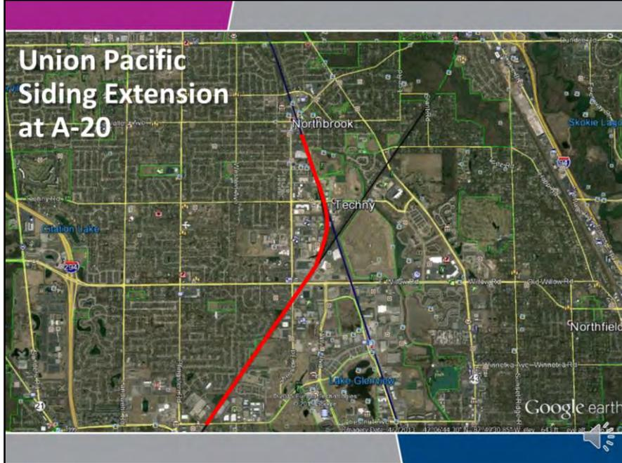
Let's take a closer look at the Union Pacific Siding Extension project. A range of six alternatives was considered to address capacity and delay issues at the Union Pacific junction with the Canadian Pacific at the A-20 control point in Northbrook, IL. Four of the alternatives did not meet the purpose and need of the project and/or had significant environmental impacts associated with them. Two alternatives for the Union Pacific siding projects advanced to the EA.
