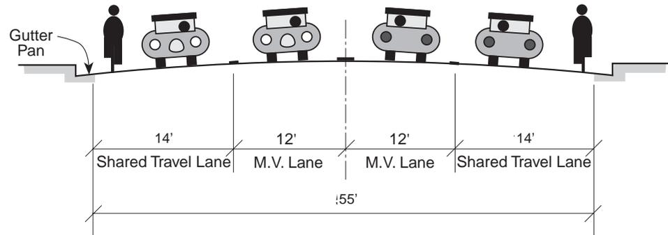
For instance, on those road segments where no parking is allowed, the travel lane (from gutter pan joint line to lane stripe) should be 14 feet in width, reflecting the unsuitability of bicycle riding too close to the curb face or in the gutter pan, itself.
