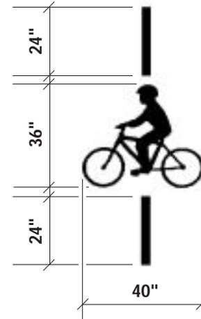
square or rectangular loops, for example, the right edge of the loop is often sensitive enough to detect bikes and can be marked with a special pavement marking. A number of cities have experimented with various designs; the Madison design is shown above.
