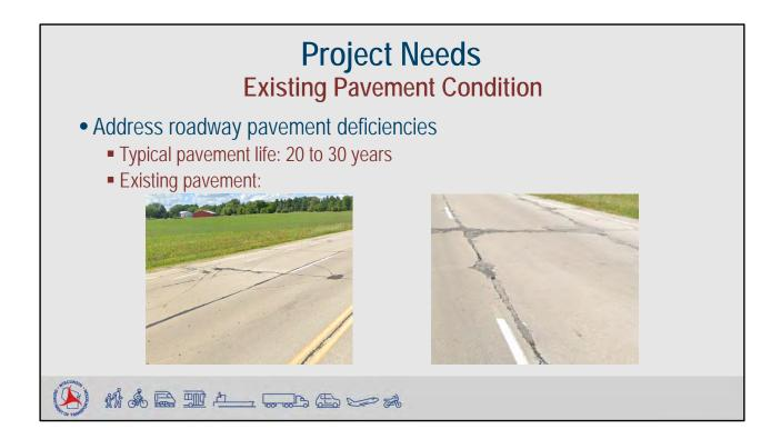
Another need that was previously noted includes addressing the existing pavement condition. Typically, pavement will last approximately 20 to 30 years. The existing concrete pavement was installed in 1992 and is at its 30-year lifespan. As you can see from the pictures, it is deteriorating and in need of improvements.
