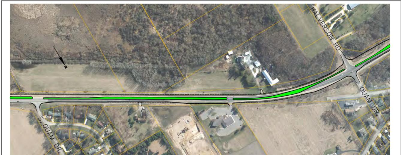
**Figure 13 Example of Raised Median Between Closely Spaced Intersections in 2-lane Section**
