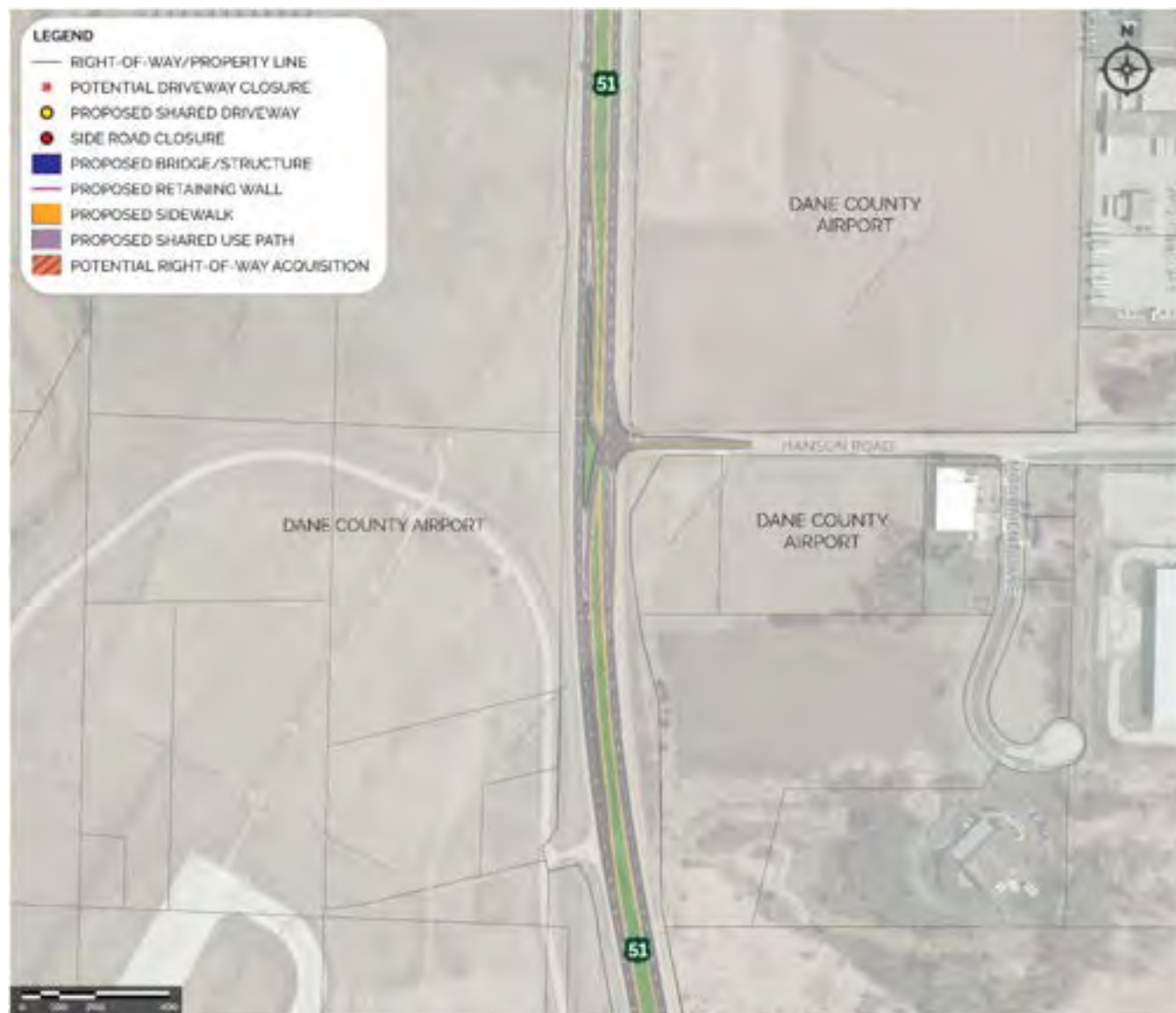
Figure 31: Preferred Alternative for the Hanson Road Intersection
