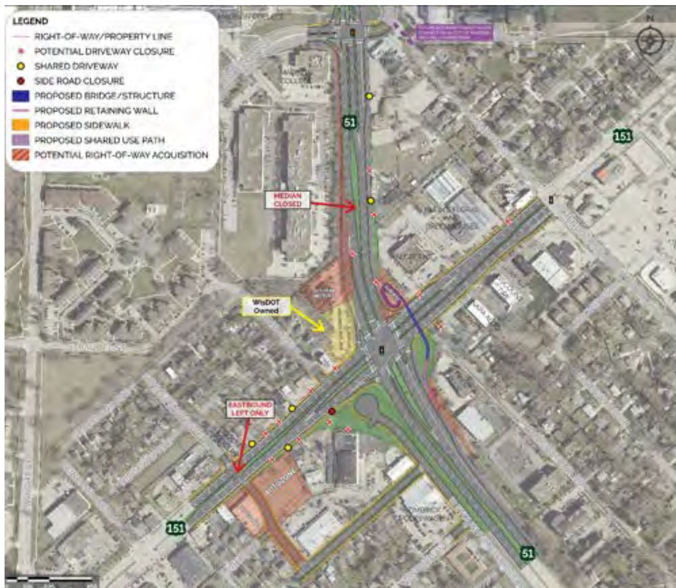
Figure 25: Preferred Alternative for the US 151/East Washington Avenue Intersection
