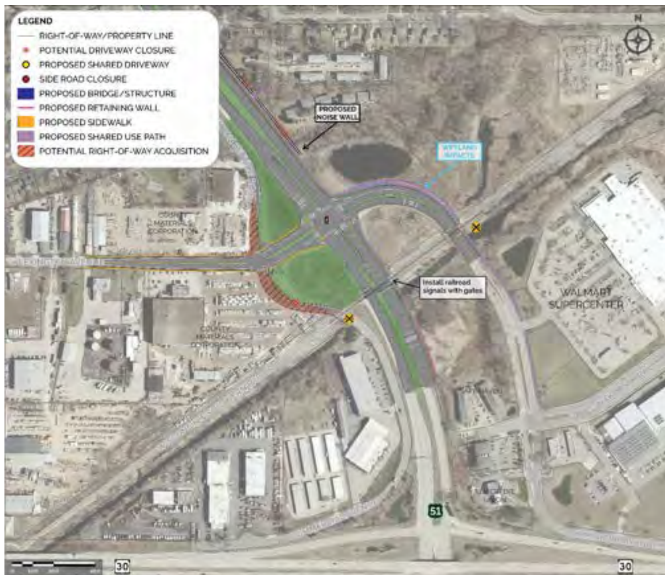
Figure 24: Preferred Alternative for the Commercial Avenue/Lexington Avenue Intersection
