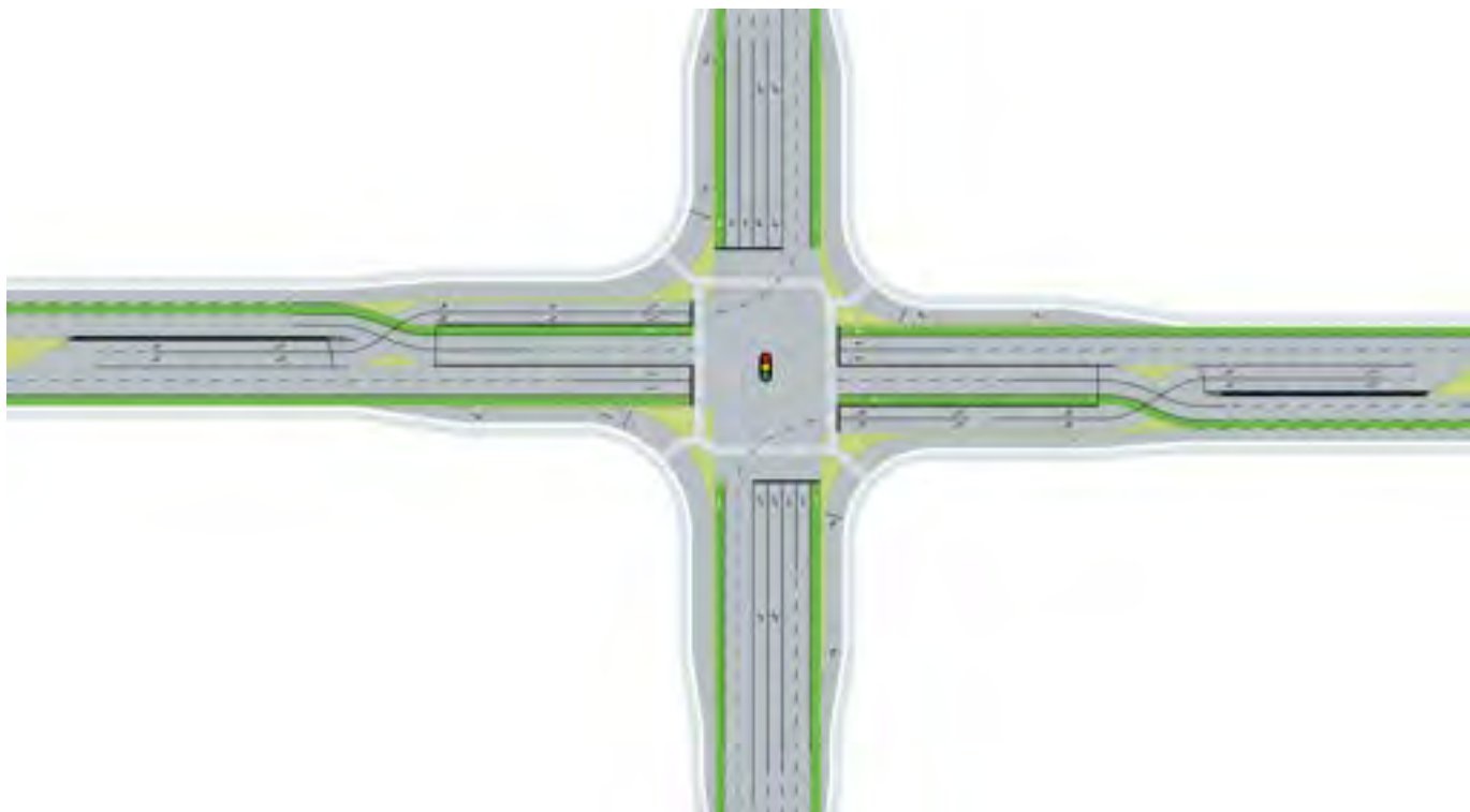
Figure 20: Displaced Left Intersection
