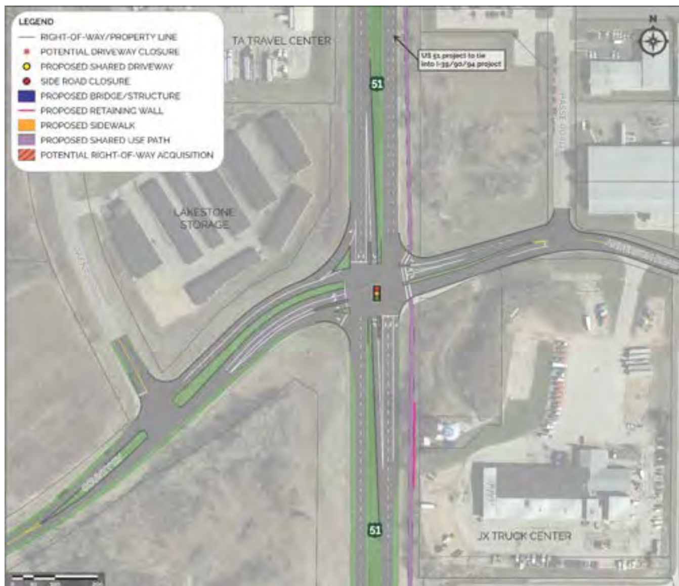
Figure 34: Preferred Alternative for the County CV/Anderson Road Intersection
