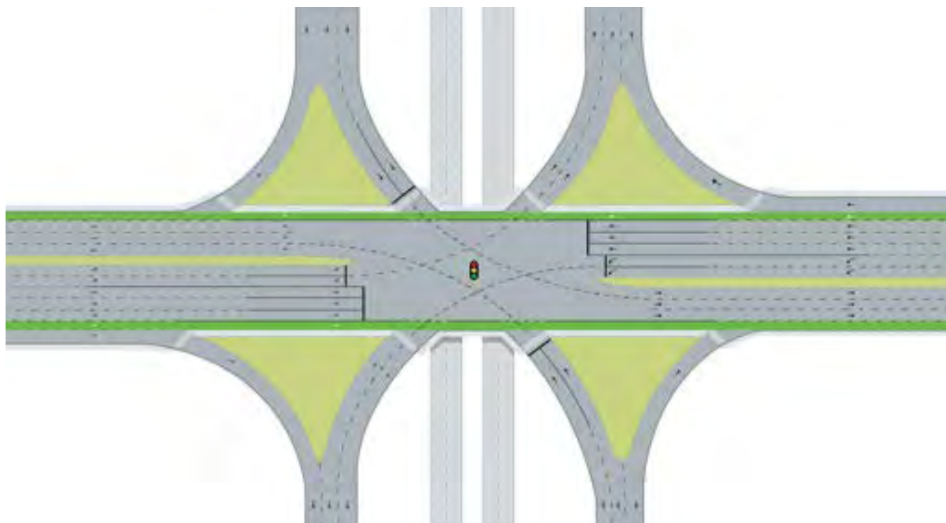
Figure 22 Single Point Urban Interchange (SPUI)
