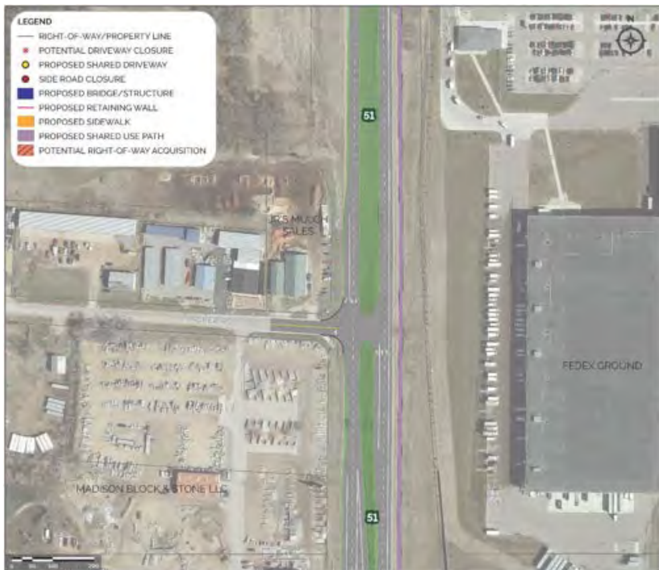
Figure 33: Preferred Alternative for the Acker Road Intersection
