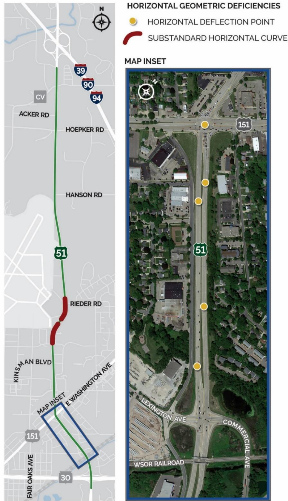
Figure 3-19: Horizontal Alignment Deficiencies
