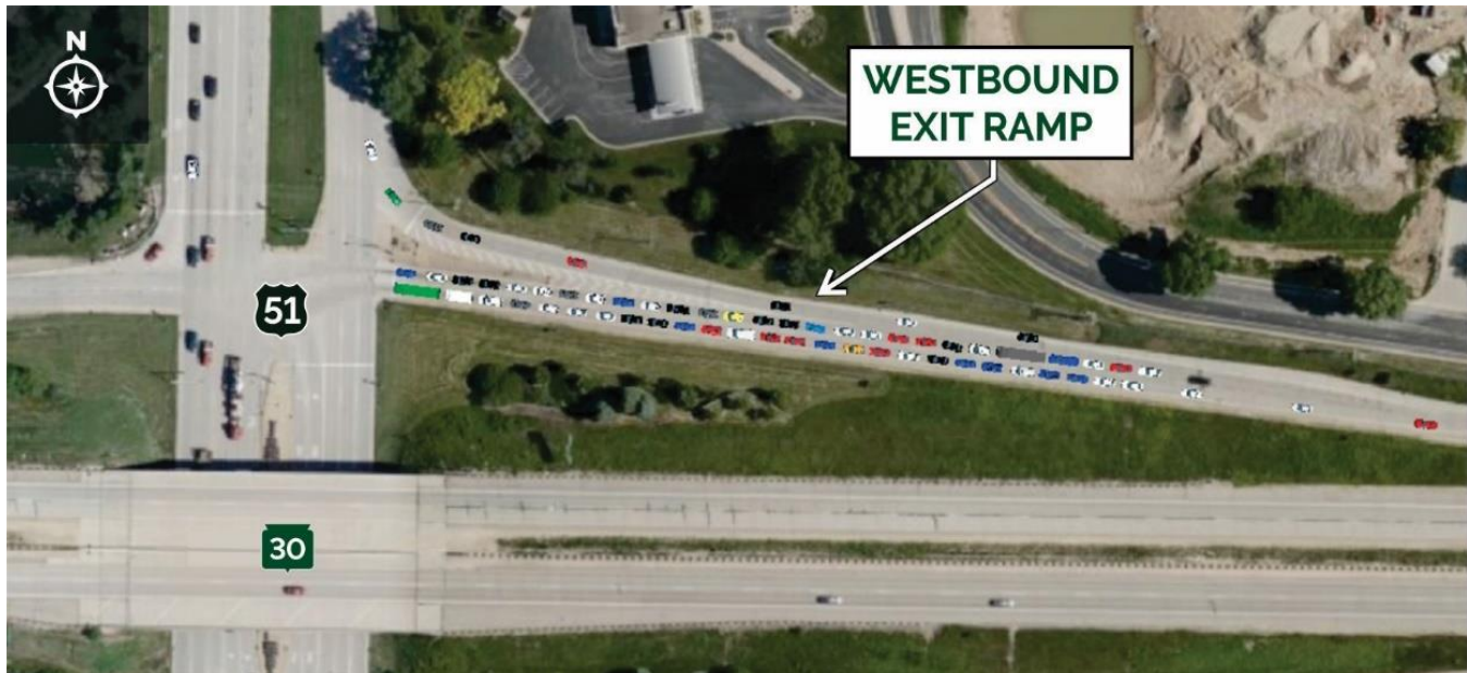
Figure 3-16: Year 2022 AM Peak Hour Vissim Model WIS 30 Exit Ramp Congestion
