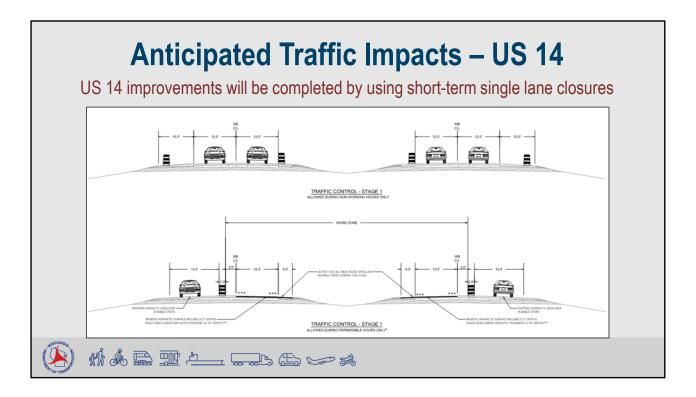
When lane closures are in place on US 14, traffic would be shifted onto the respective inside or outside shoulder, depending on the stage of work. As shown above for stage 1 work, traffic will be on the outside shoulders. During stage 2 and 3 traffic would be on the inside shoulders during lane closures. During stage 4 they would be back on the outside shoulder during lane closures.
