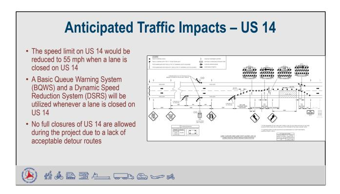
When lanes are closed on US 14, the posted speed limit would be reduced from 70 mph to 55 mph. The contractor would not be allowed to close US 14 during the project.
