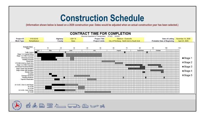
When construction does occur, there are four stages of work to be completed and the project is estimated to last approximately 6 months – from late April through late October of a calendar year.
