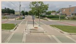
Median openings for bicyclists at intersections with an RRFB, including push buttons that activate the RRFB system. A similar configuration is at the WIS 35 & King Street intersection.
