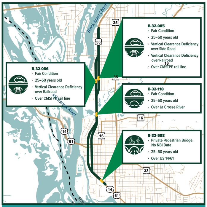
The three US 53 bridges are scheduled for a concrete overlay. The pedestrian bridge near the Gunderson hospital is a private facility and no rehabilitation work is anticipated.
