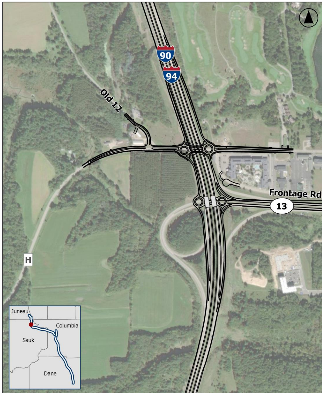
Figure 2-21: WIS 13 – Split Diamond Interchange
