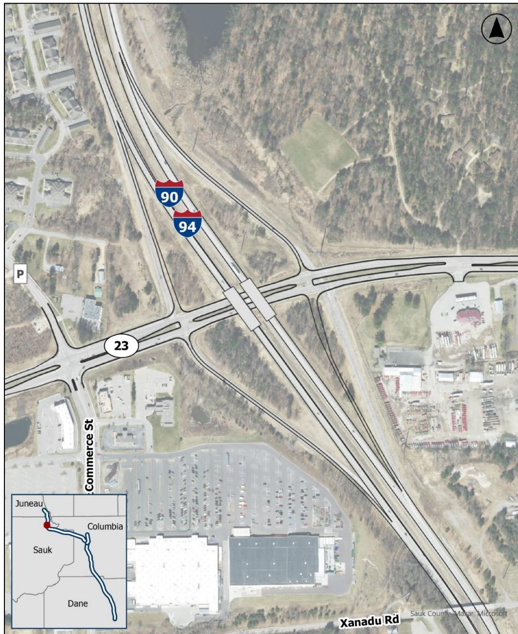
Figure 2-20: WIS 23 – Diamond Interchange
