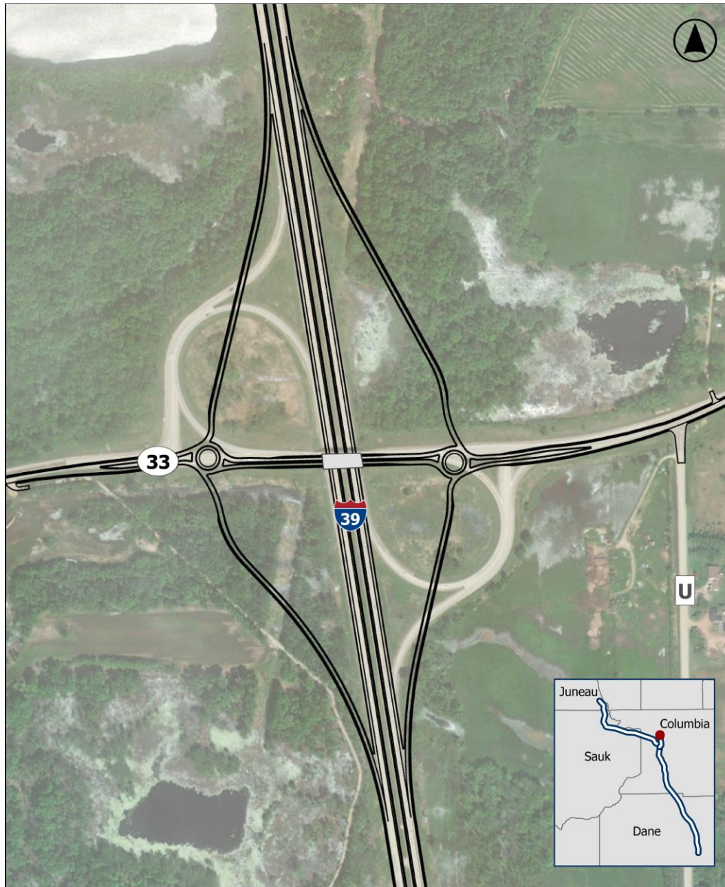
Figure 2-17: WIS 33 at I-39 – Diamond Interchange
