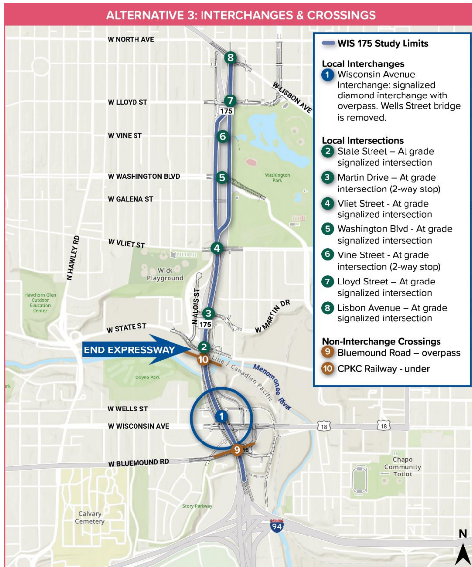
Figure 35 – WIS 175 Interchanges and Crossings – Alternative 3
