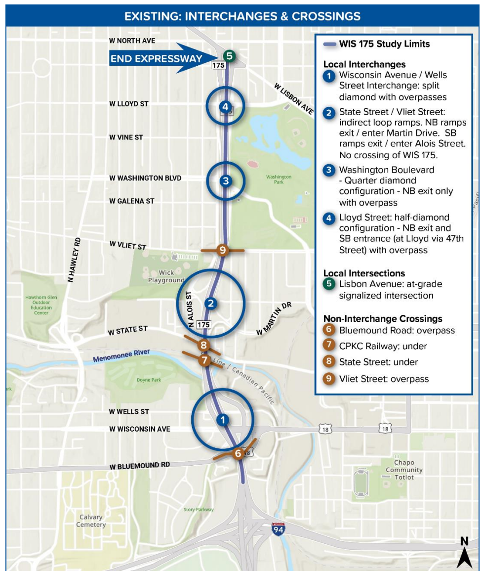
Figure 11 - Interchanges and Crossings – Existing
