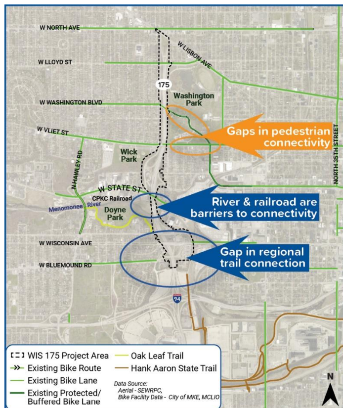
Figure 16 - WIS 175 Existing Bicycle & Pedestrian Facilities
