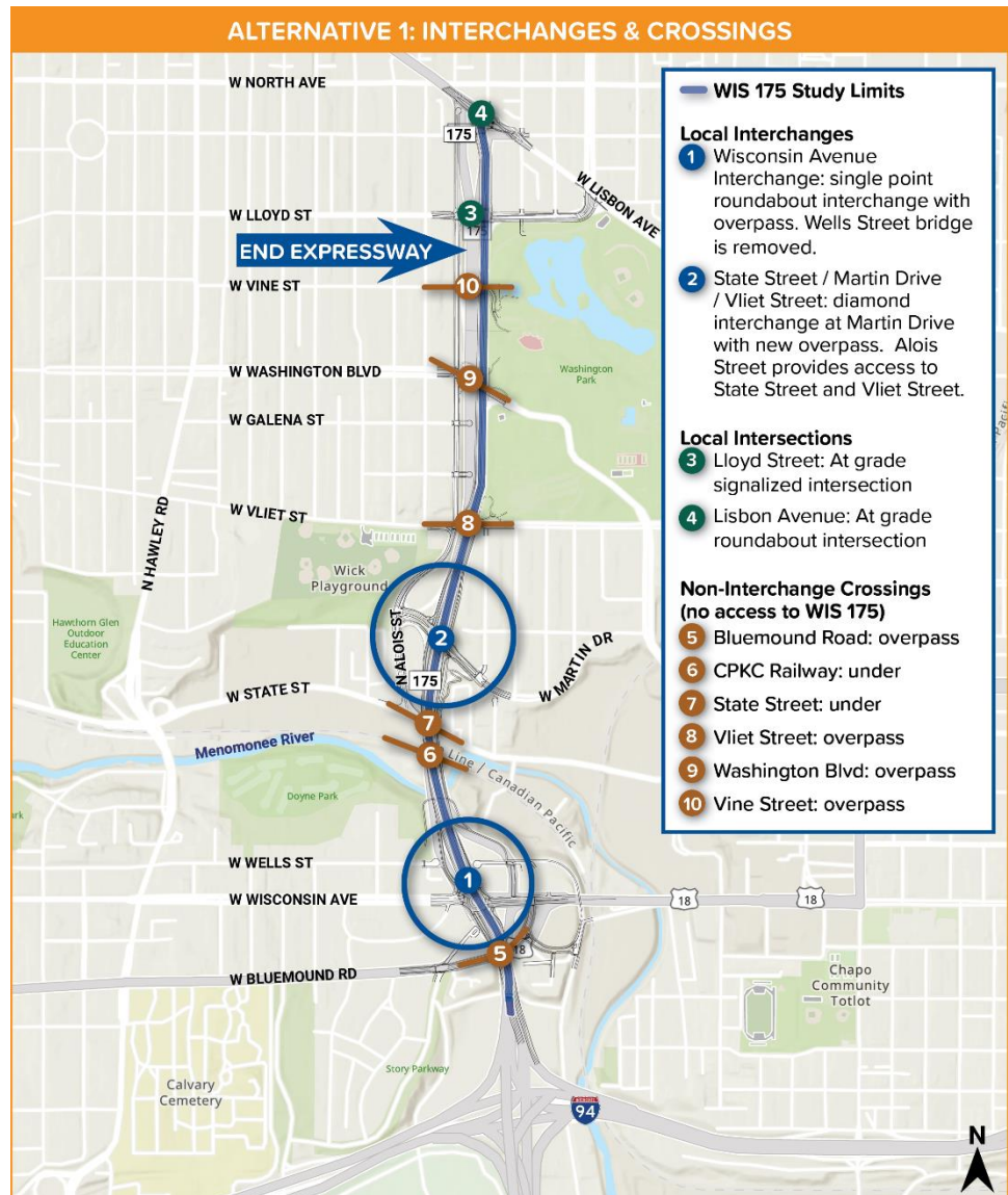
Figure 31 – WIS 175 Interchanges and Crossings – Alternative 1
