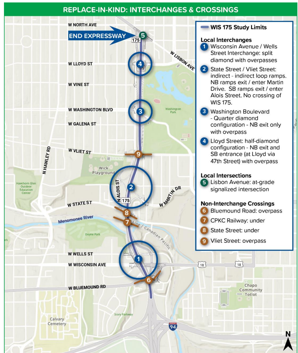
Figure 29 – WIS 175 Interchanges and Crossings – Replace-In-Kind
