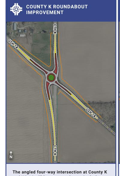
The angled four-way intersection at County K and US 14 will be converted to a single-lane roundabout to improve vehicular safety.
