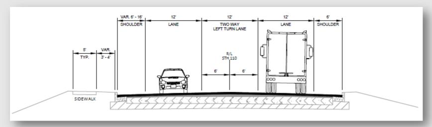
Finished typical section through lane reconfiguration areas
